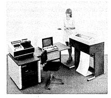
spooling, a standard on the system, makes it possible to input jobs from the 300 or 600 cpm card reader to disc, output another job from the disc to the 300 to 1800 lpm printer, and receive or transmit a third job over a
