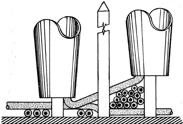
FIG. 16 - CHANNEL BUILD-UP EFFECT ON SHORT Z-1 WRAPS WHEN THEY ARE NOT PUT ON FIRST
