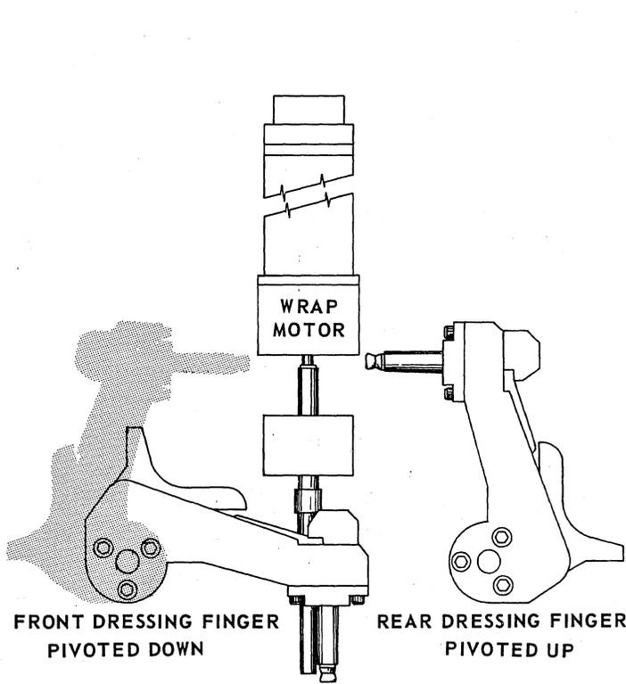
FIG. 5 - DRESSING FINGERS PIVOTED AND STORED (SIDE VIEW)
