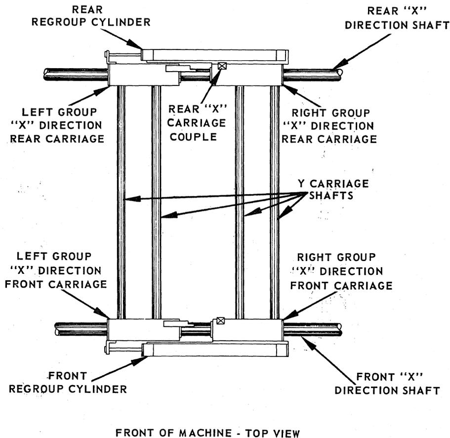
FIG. 1. "X" MOTION CARRIAGES AND REGROUP CYLINDERS
