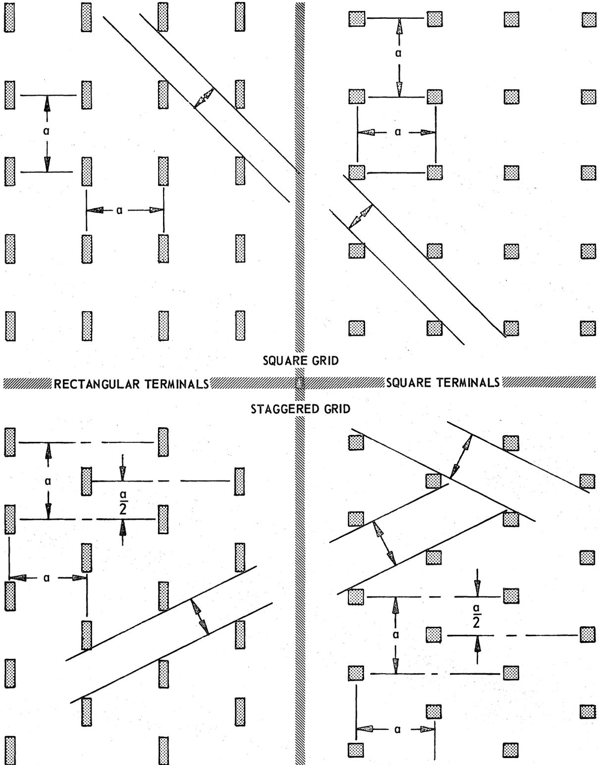
FIG. 15 - PANEL TERMINALS AND GRIDS
