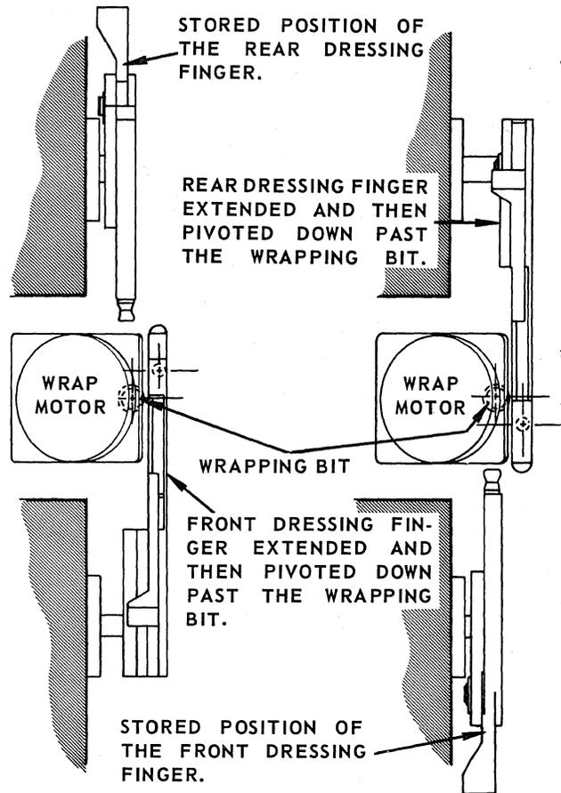
FIG. 6 - DRESSING FINGERS PIVOTED AND STORED (TOP VIEW)
