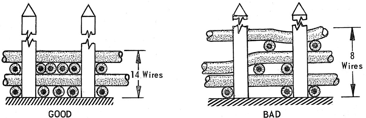
FIG. 18 - SEQUENCING TO REDUCE CHANNEL BUILD-UP
