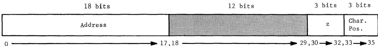
Figure III-9. Indirect Word as Interpreted under CI
