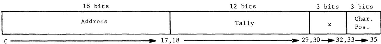
Figure III-8. Indirect Word as Interpreted under SC
