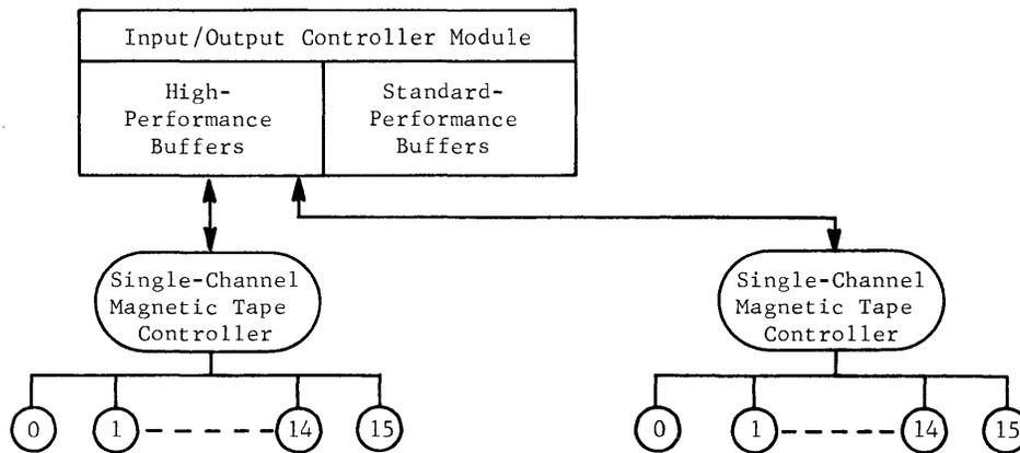
A single-channel magnetic tape subsystem connected to a high-performance channel of an Input/Output Controller permits reading or writing on any one of up to 16 magnetic tape units connected to that controller. Reading or writing proceeds simultaneously with other peripheral operations on other peripheral channels and with Processor operations. Multiple single-channel tape subsystems make possible simultaneous read-read, read-write, or write-write operations.
