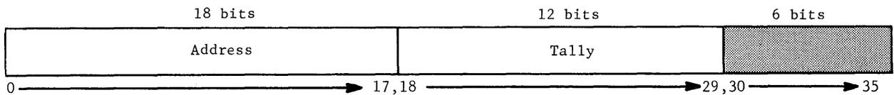
Figure III-7. Indirect Word as Interpreted under ID or DI
