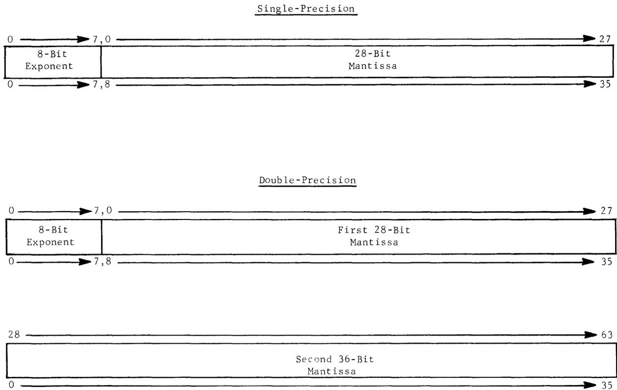
Figure III-3. Floating-Point Data Formats
