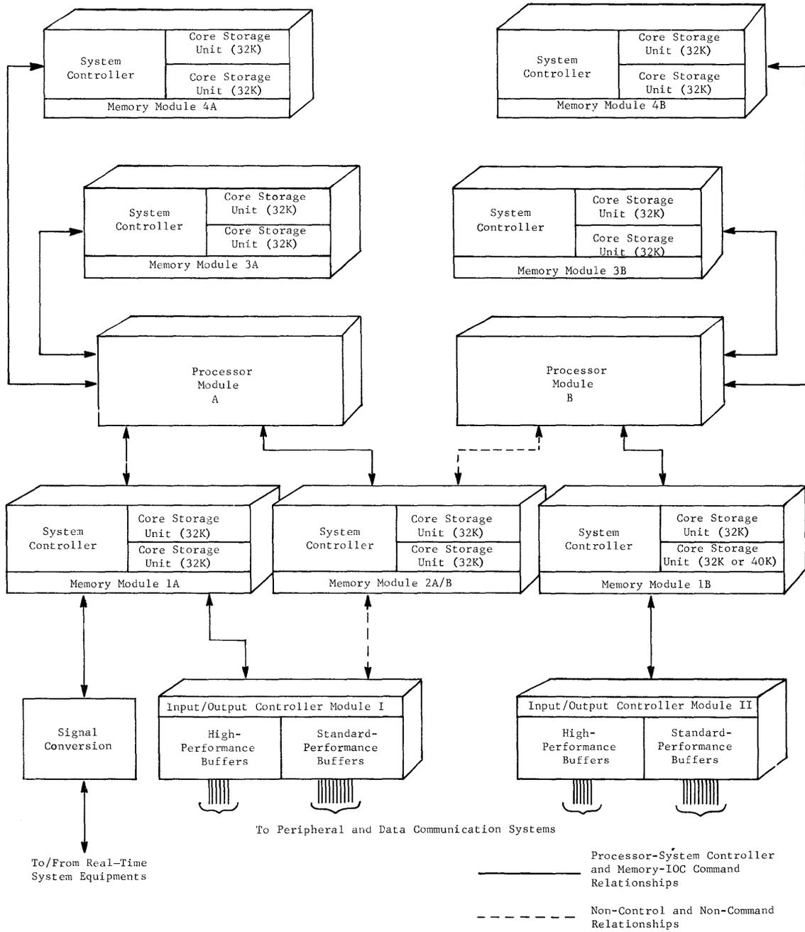
Figure I-4. Multicomputer Configuration with One Shared Memory Module
