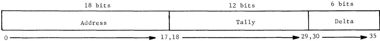
Figure III-10. Indirect Word as Interpreted under AD
