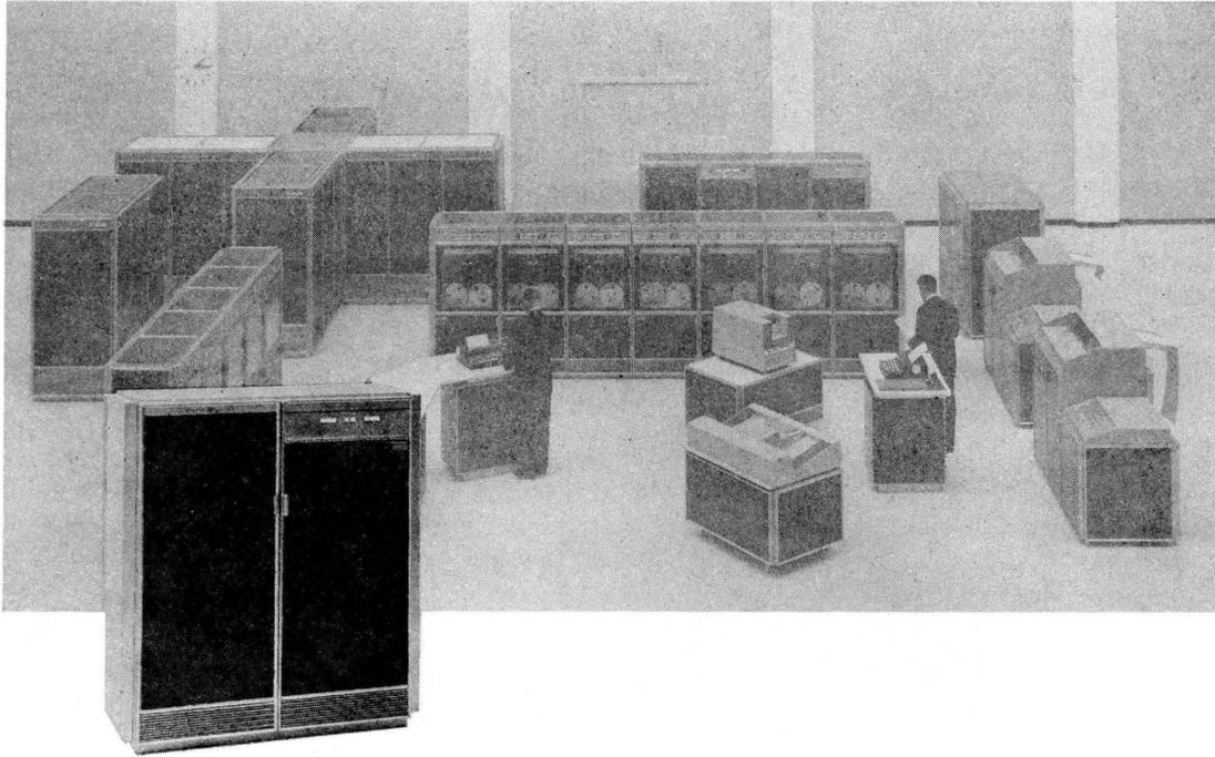
The MD-20 Magnetic Drum Subsystem is a high-performance auxiliary data storage facility. Communication with the GE-635 is through a high-performance channel on the Input/Output Controller at a rate of up to 370,000 characters per second. The storage capacity of one magnetic drum is six million characters (one million words). Average access time is 8.5 milliseconds. Data is stored in blocks of 384 six-bit characters, with all blocks addressed sequentially.
