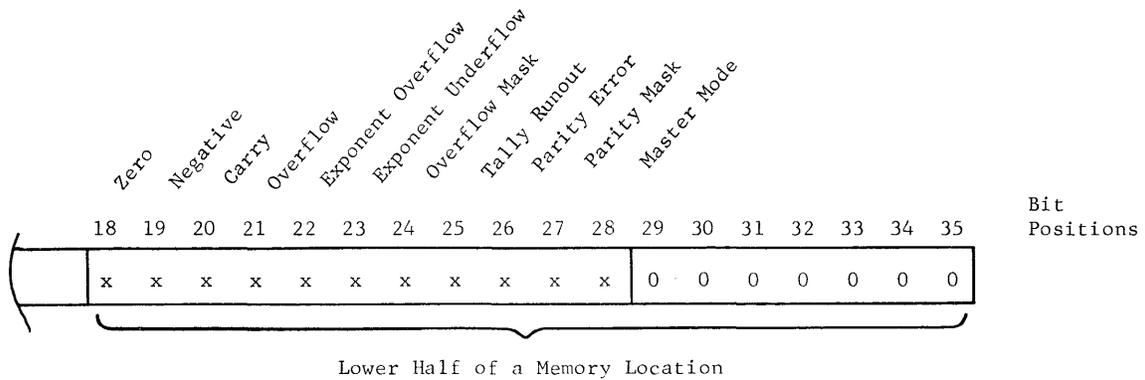
Figure III-1. Indicator Register Format
