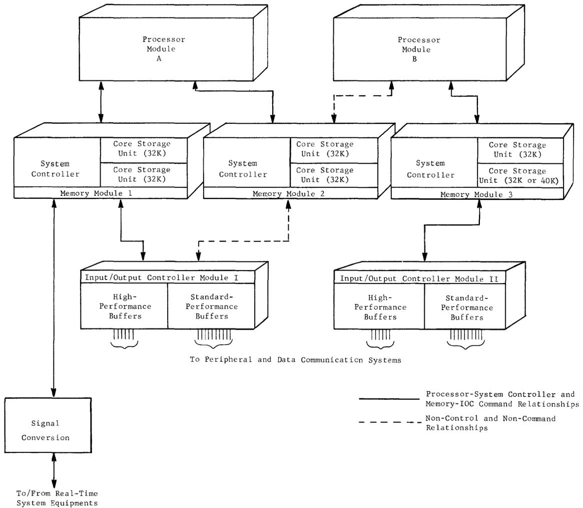
Figure I-3. Multicomputer Configuration
