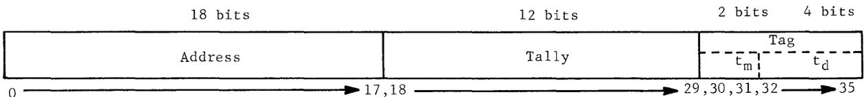
Figure III-11. Indirect Word as Interpreted under IDC and DIC
