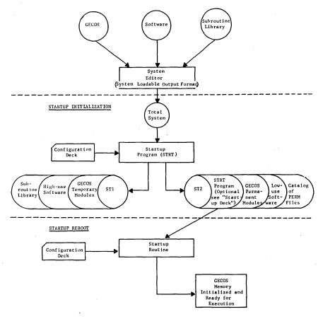
Figure 1. System Startup
