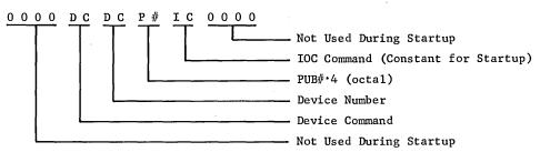
The specific setting for the DATA thumbwheels for a Card Bootstrap for GE-625/635 system with the Card Reader on PUB #6 as follows:
