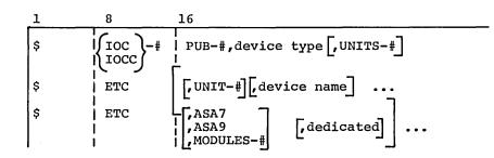
The CONFIG entry for an IOC channel specifies the IOC number (0-3), channel (PUB) number (0-15), and the type of peripheral device attached. The IOC model, number of attached units, and individual unit characteristics may also be included.
