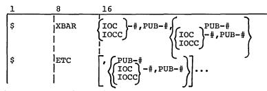
The hardware configuration entry for a crossbar arrangement specifies all of the IOC channels which are mutually crossbarred.
