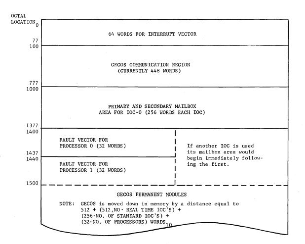
Figure 11. GECOS Lower Control Memory Layout
