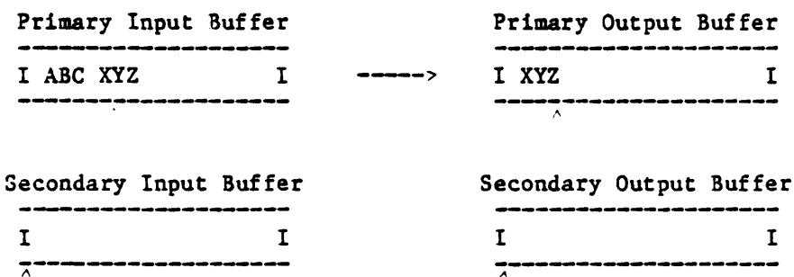
Here the PROC has been invoked by the characters ABC XYZ, which are then automatically placed in the primary input buffer. PROC commands have then been processed which position the input pointer of the primary input buffer to the second parameter (XYZ), and then subsequently move that parameter to the primary output buffer as illustrated by the path between the buffers (i.e., the currently active buffers are the primary input buffer and the primary output buffer).
