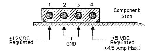
Note: Current requirements for the +12 Volt DC supply depend on the serial adapter board used.
