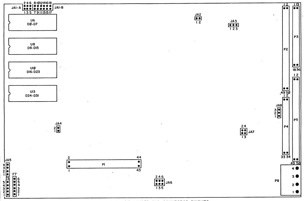
GMX MICRO-20 JUMPER AND CONNECTOR PINOUTS
