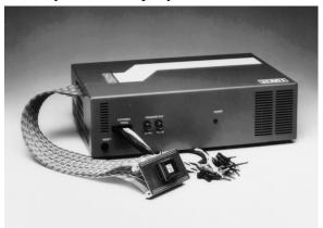
The HMI-200-68000 emulator is a high performance development system which combines the control of an in-circuit emulator with the power of a logic analyzer to provide a complete debugging environment for hardware and software.
