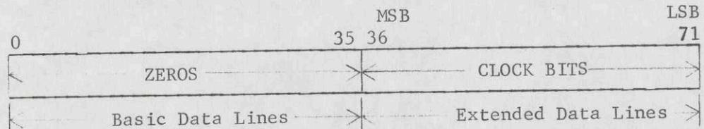
Bit 71 is the least significant bit (LSB). The ETC is incremented by one at one microsecond intervals. Maximum ETC capacity is approximately 19 hours before "rollover". This ETC is not settable. Active System modules shall not be notified when "rollover" occurs.
