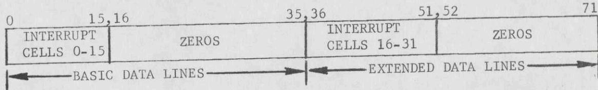
The RGR-IC command does not alter the contents of the interrupt cells.
