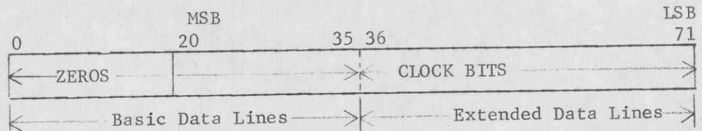
Bit 71 is the least significant bit (LSB). The ETC is incremented by one at one microsecond intervals. Maximum ETC capacity is approximately 142 years before "rollover", if bits 20 thru 55 are set to zero. Active System modules shall not be notified when "rollover" occurs.
