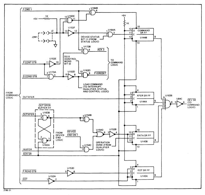
Figure 3-24. Device Service Request Logic
