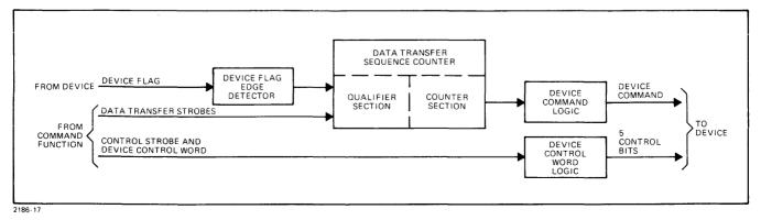
Figure 3-10. Device Control Logic Block Diagram
