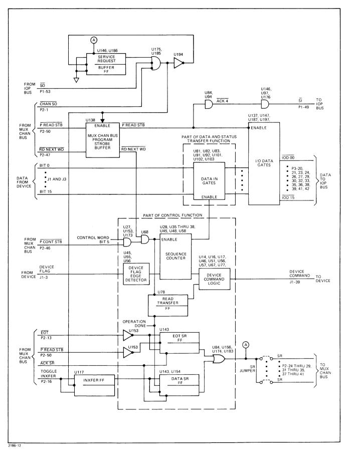
Figure 3-5. Program Read Strobe Functional Logic Diagram
