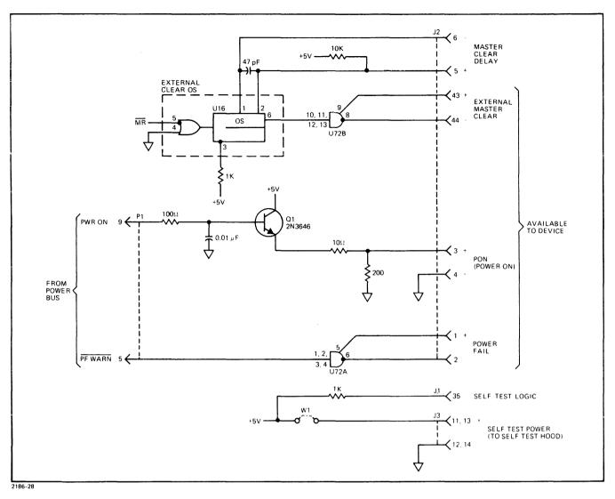
Figure 3-21. Discrete Device Control Signals
