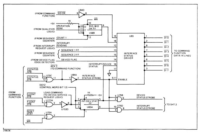
Figure 3-29. Status Logic and Control (Sheet 1 of 2)
