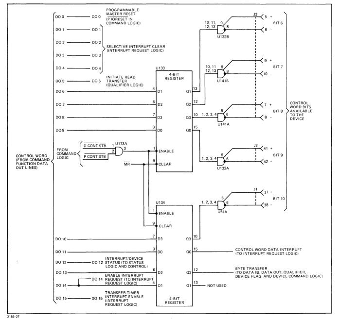
Figure 3-20. Device Control Word Logic
