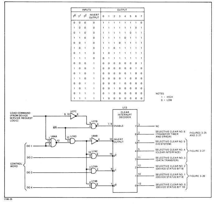
Figure 3-28. Clear Interrupt Decoder Logic
