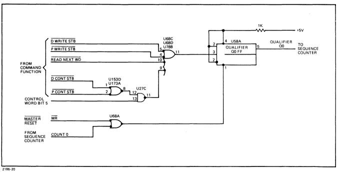
Figure 3-12. Qualifier Q0 Simplified Diagram
