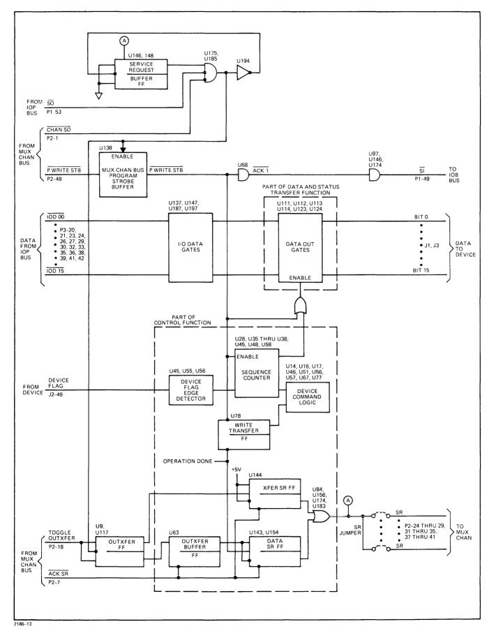
Figure 3-6. Program Write Strobe Functional Logic Diagram
