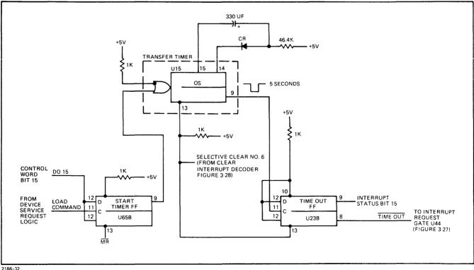
Figure 3-25. Data Transfer Timer Interrupt Request Logic
