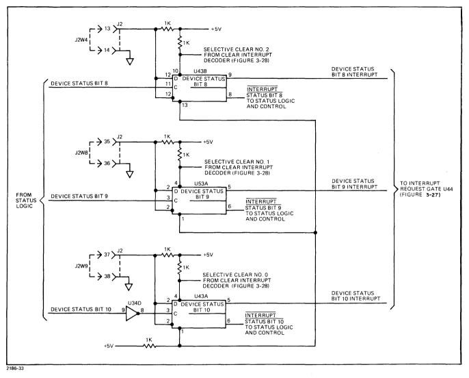
Figure 3-26. Device Interrupt Request Logic
