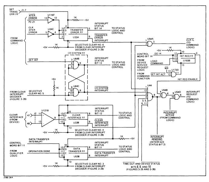
Figure 3-27. I/O System and Interface Interrupt Request Logic
