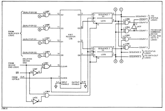
Figure 3-16. Sequence Counter Simplified Diagram
