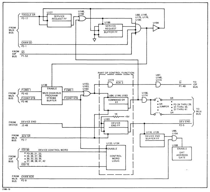
Figure 3-3. Program Control Strobe Command Functional Logic Diagram
