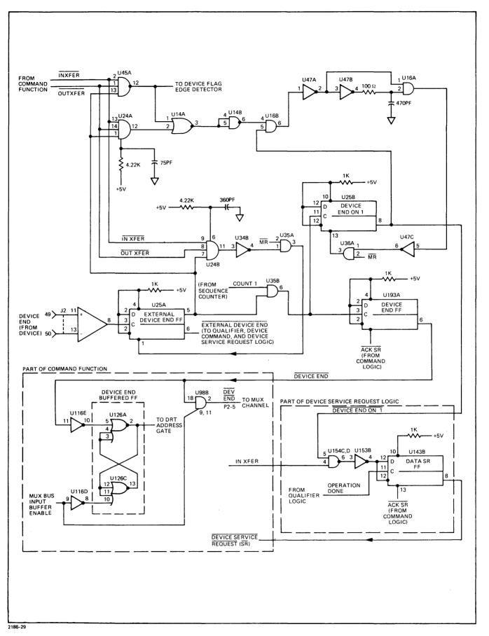
Figure 3-22. Device End Logic
