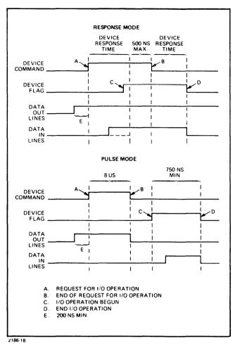
Figure 3-11. Response Mode and Pulse Mode Timing Diagrams
