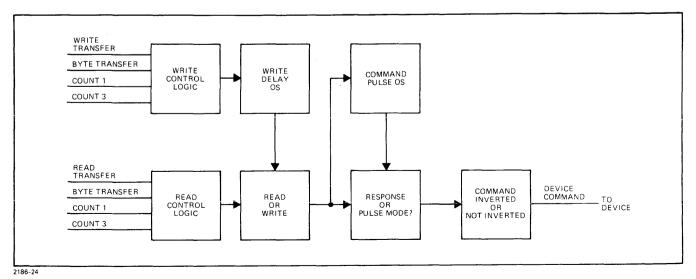
Figure 3-17. Device Command Logic Block Diagram
