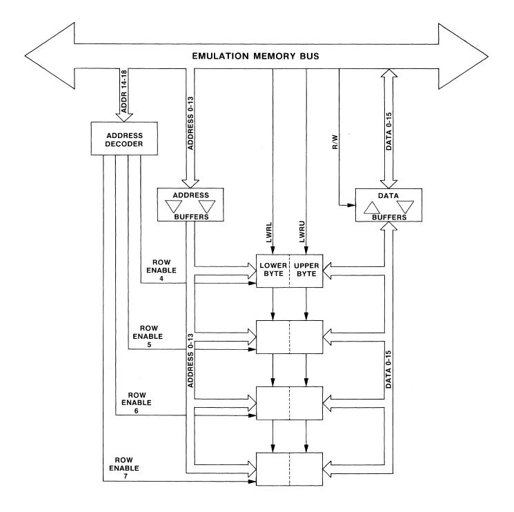
Figure 8-2. Emulation Memory Block Diagram.
