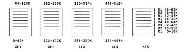
XE1-4 determine the addressable range of the Memory Card. The primary purpose for XE5 is to configure the 6416X series Memory to be compatible with the 6415X series Memory. XE5 performs row mapping. The following guidelines will help you avoid memory mapping errors.
