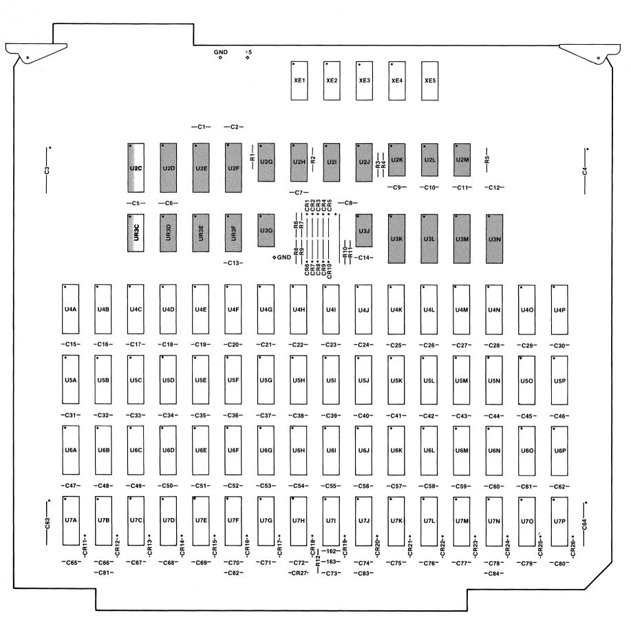
Figure 8-3. Model 64161A/162A/163A Component Locator 8-12
