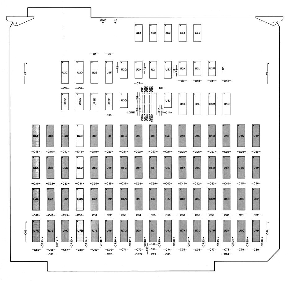
Figure 8-5. Model 64161A/162A/163A Component Locator 8-14
