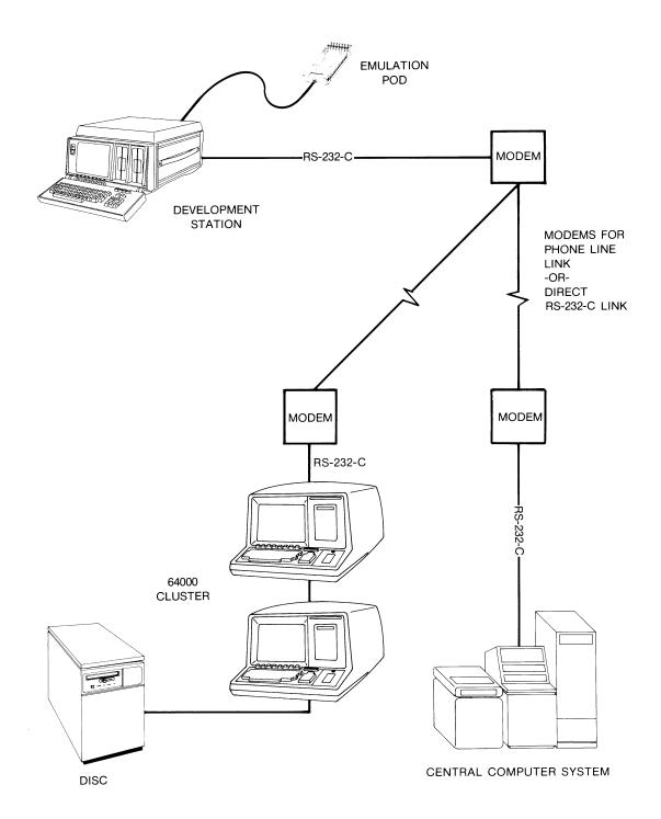
Figure 2-7. RS-232-C Linking a Remote Development Station
