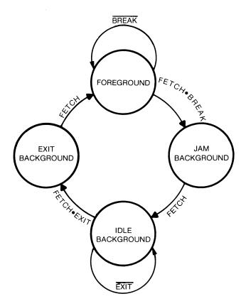
Figure 5-7. Emulator Four-state Operation
