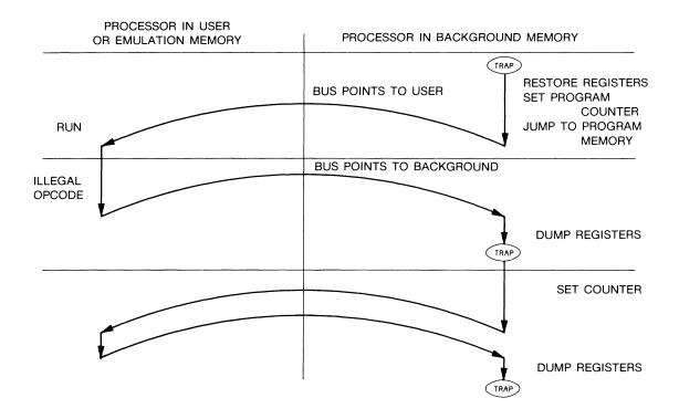
Figure 5-9. Non-real-time Analysis Operation
