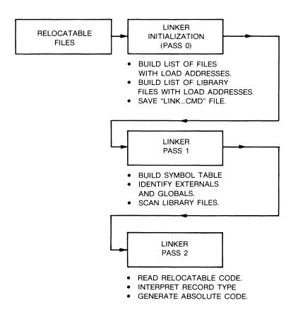
Figure 5-5. Linker Module Functions
