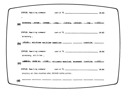
Figure 4-3. Constructing a Command Using the Softkeys
