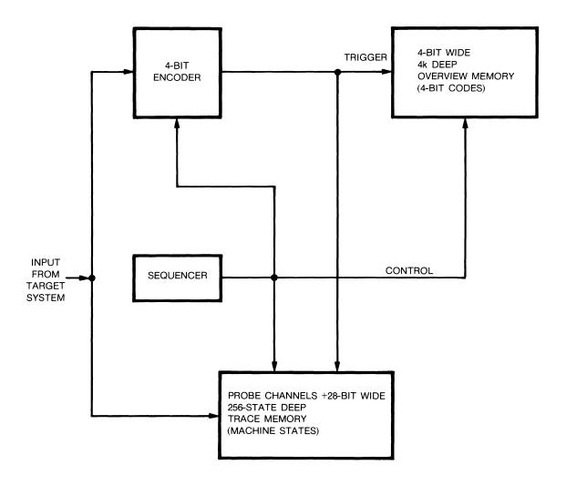
Figure 5-12. Logic State/Software Analyzer Memory
