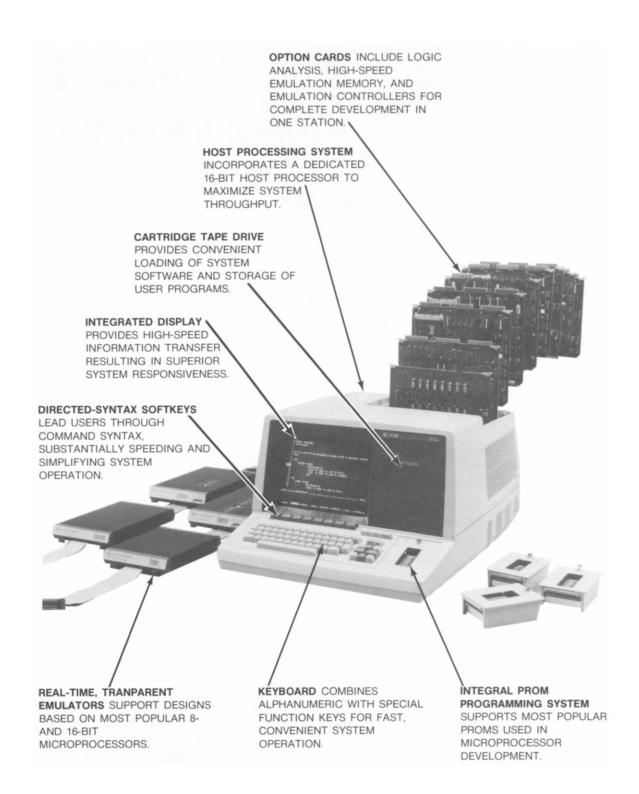
Figure 1-1. The 64000 Logic Development System
