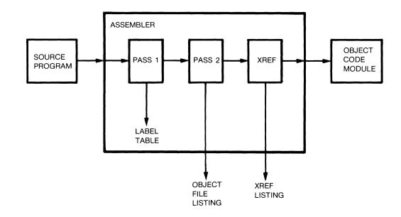
Figure 5-3. Assembler Two-pass System
