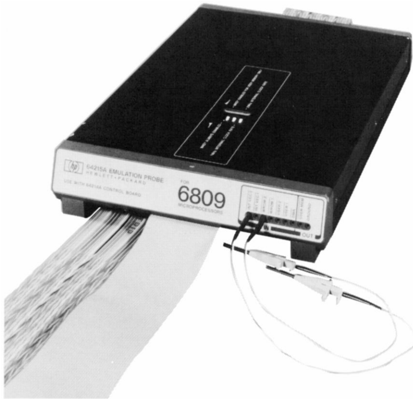
Figure 3-2. 6809 Series Emulator Pod
