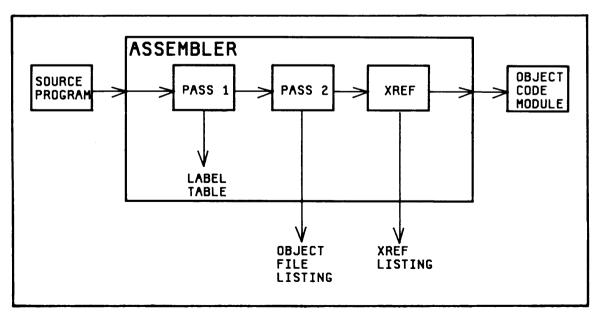
Figure 6-1. Assembly Flow Diagram
