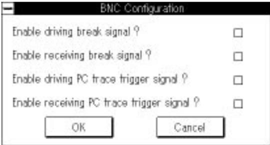
Enable driving break signal? When selected, the Processor Probe outputs the signal on the "TRIGGER OUT" BNC port as it breaks.
