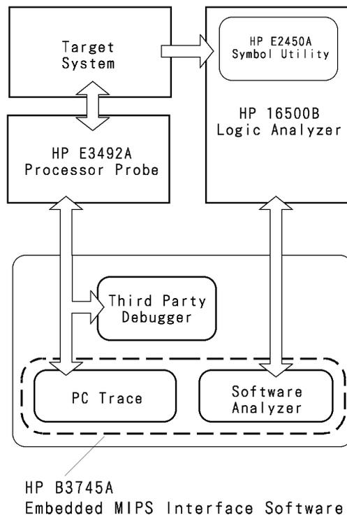
HP B3745A Embedded MIPS Interface Software consists of two software components interfacing individual debugging tasks; the PC Trace for tracing PC of user program and the Software Analyzer for controlling the HP 16500B Logic Analyzer.
