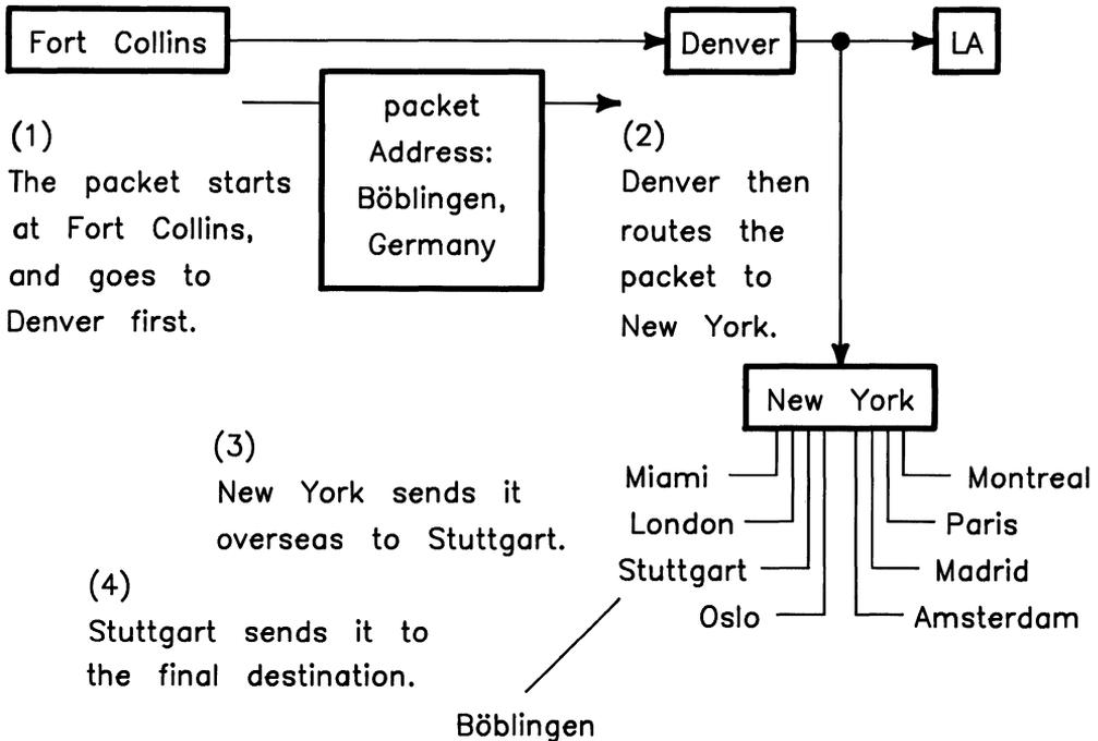
**Figure 8-2. Packet Switched Network**
