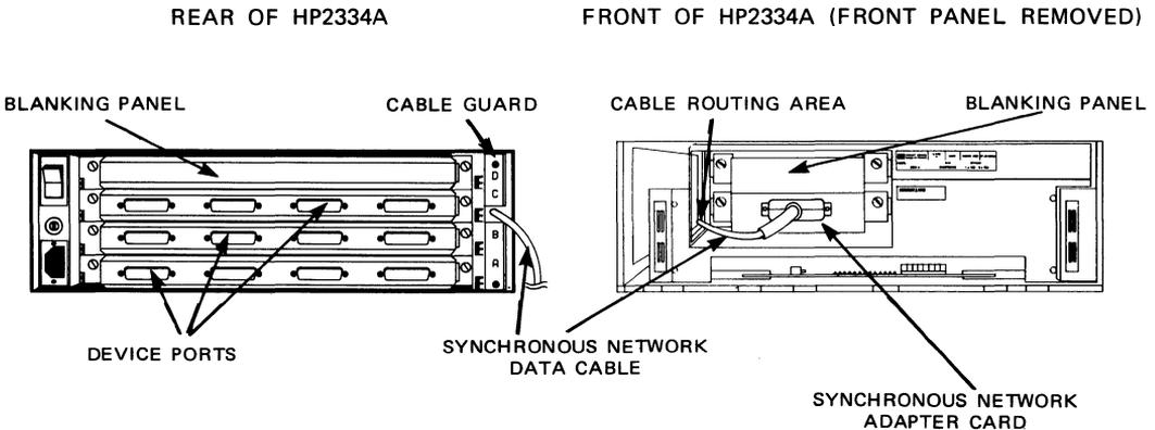
**Figure 8-4. HP 2334A to Device and Synchronous Network Connection**
