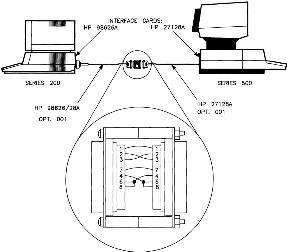
**Figure 2-7. Series 200 to Series 500 (bidirectional)**
