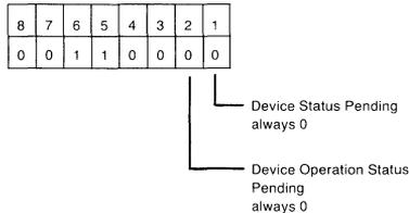
(tracks "S", "F", or "U" completion codes associated with E&p device control sequences.)
