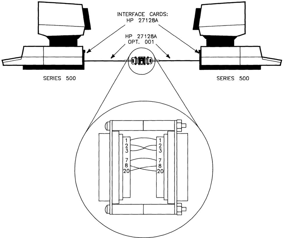
**Figure 2-11. Series 500 to Series 500 (unidirectional)**
