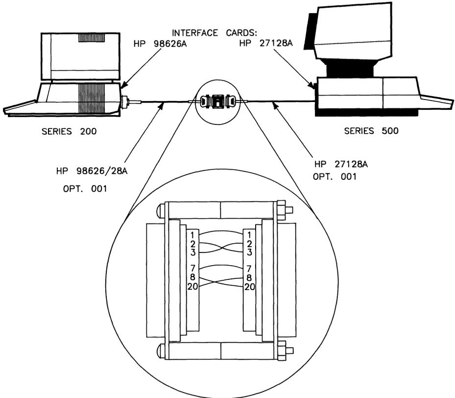
**Figure 2-6. Series 200 to Series 500 (unidirectional)**
