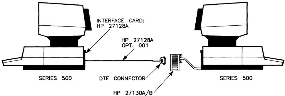
**Figure 2-9. Series 500 to Series 500 MUX**
