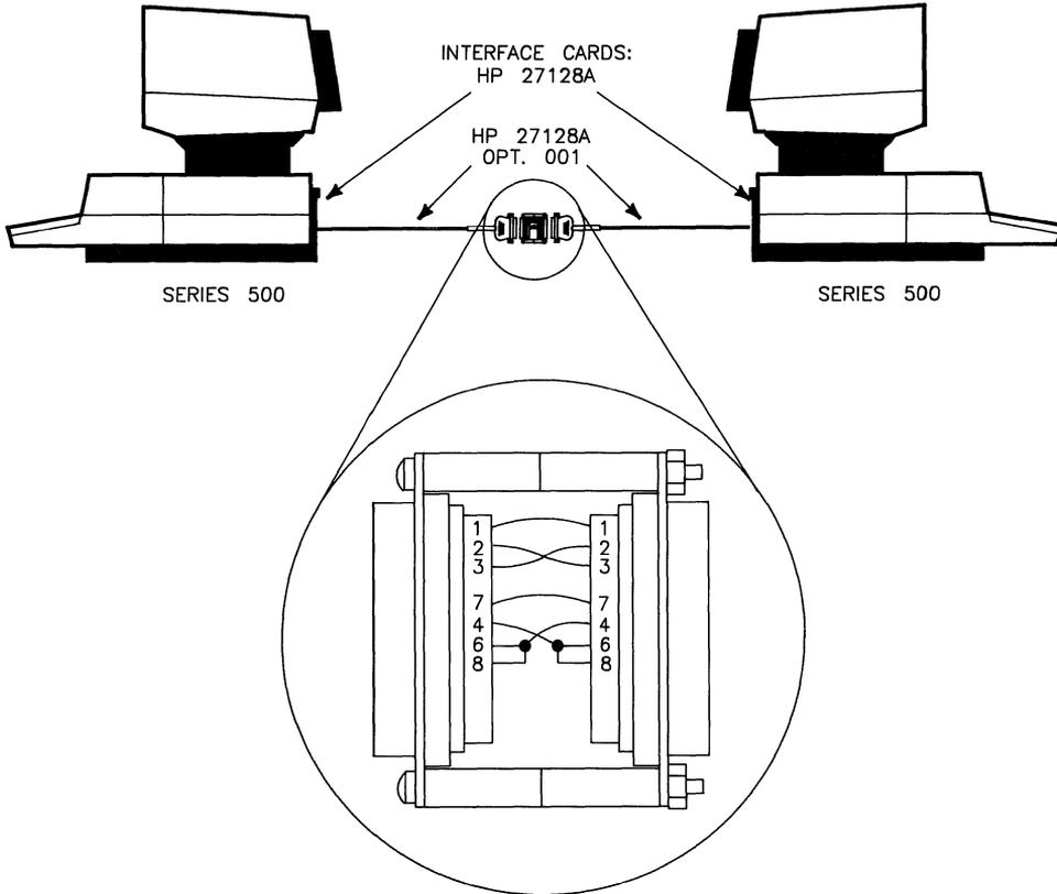
**Figure 2-12. Series 500 to Series 500 (bidirectional)**
