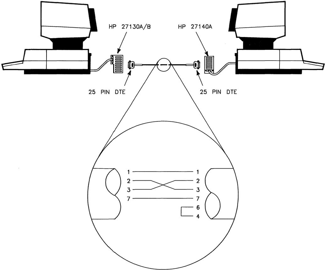
**Figure 2-14. HP 27130A/B to HP 27140A**
