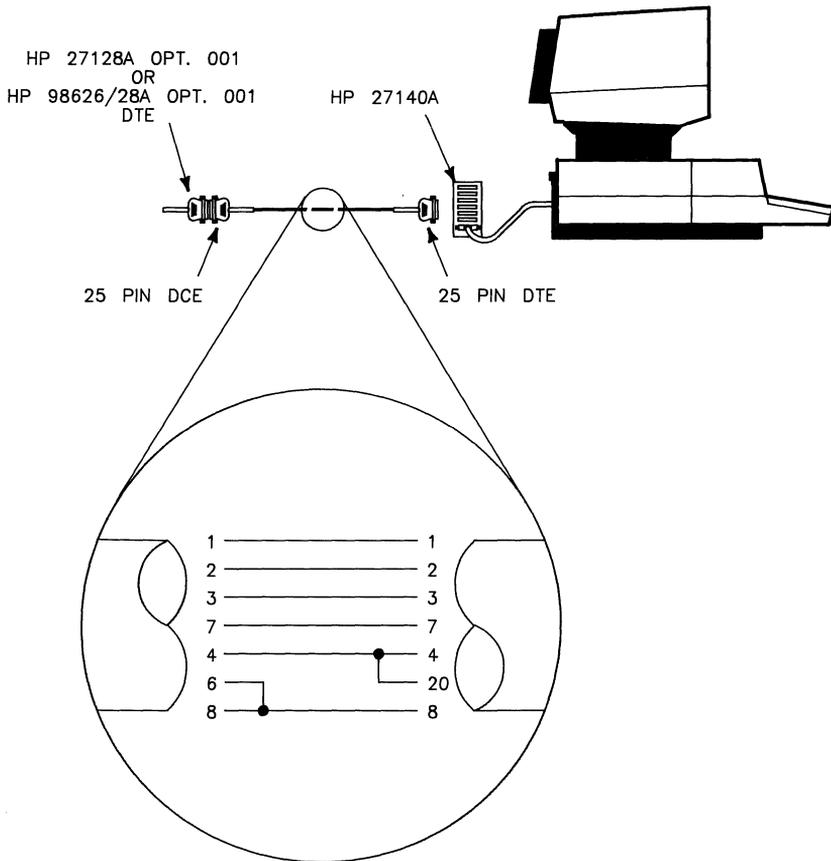
**Figure 2-16. Serial Interface card to HP 27140A**
