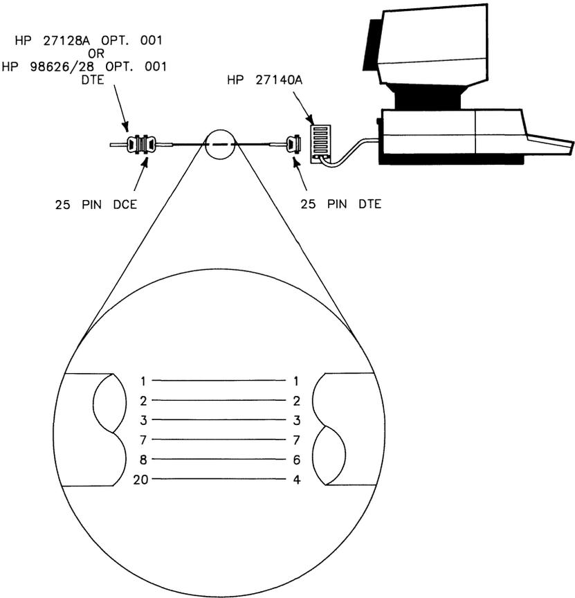
**Figure 2-13. Serial Interface card to HP 27140A**
