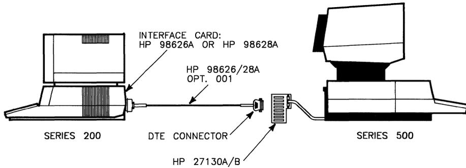
**Figure 2-5. Series 200 to Series 500 MUX**
