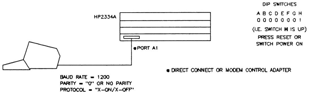
**Figure 8-7. Local Off-line Configuration**
