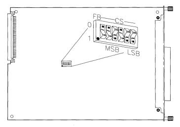
Figure 5-25. HP 98725A LGB Interface Switches
