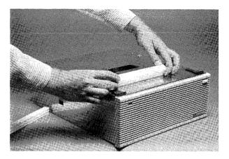
Removing the Outer Sleeve
