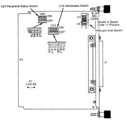
Figure 5-6. HP 98623A BCD Interface switches.
