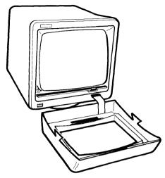
Figure 10-3. Aligning HP Touch plug with monitor socket.
