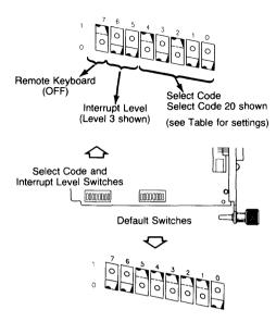
Figure 5-12. HP 98628A Datacomm Interface Switches
