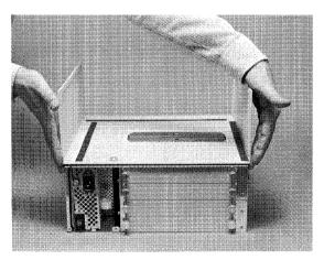
Aligning the Top from Side-to-Side
