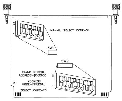
Figure 5-2. Graphics Display Station Interface switches.
