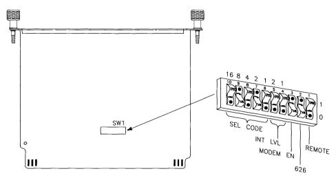
Figure 5-17. HP 98644A Asynchronous Serial Interface switches.
