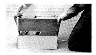
Aligning the Expander and Computer
