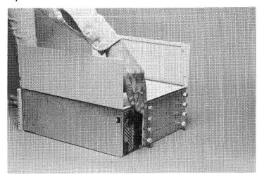
Aligning the Top from Front-to-Back
