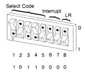
Figure 5-18. HP 98695A 3270 Coax Interface Switches
