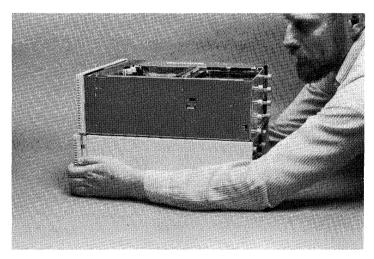
Installing the Cover on the Computer
