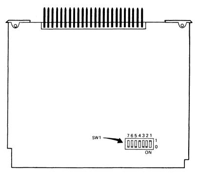
Figure 5-14. Analog Input Card Switches
