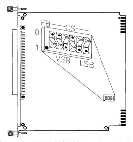
Figure 5-24. HP 98724A LGB Interface Switches
