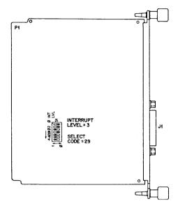
Figure 5-13. Multiprogrammer Interface Switches
