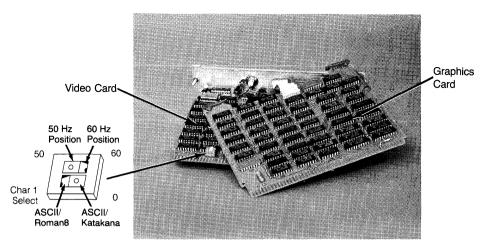
Figure 5-3. Display Compatibility Interface switches.
