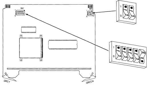
Figure 6-2. Bubble Memory Card Switches
