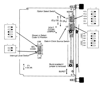
Figure 5-5. HP 98622A GPIO Switches and Jumpers
