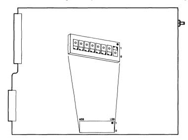
Figure 5-23. Video Board Configuration Switches
