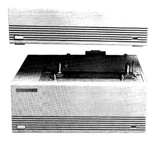
Figure 8-2. Connecting the HP 98700 to the HP 98710A
