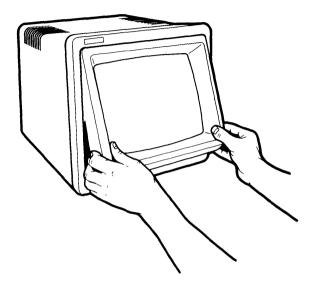
Figure 10-1. Removing CRT bezel.
