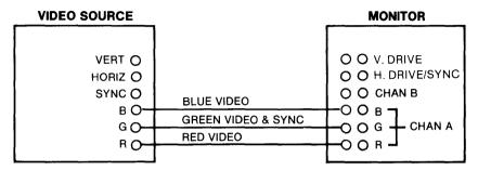
Figure 8-3. HP 13279B Cable Connections.
