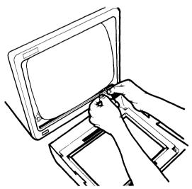
Figure 10-4. Connecting plug to socket.
