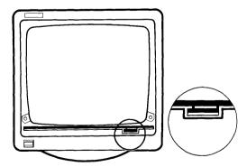
Figure 10-2. Locating socket on monitor.
