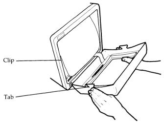
Figure 10-5. Aligning HP Touch with monitor.
