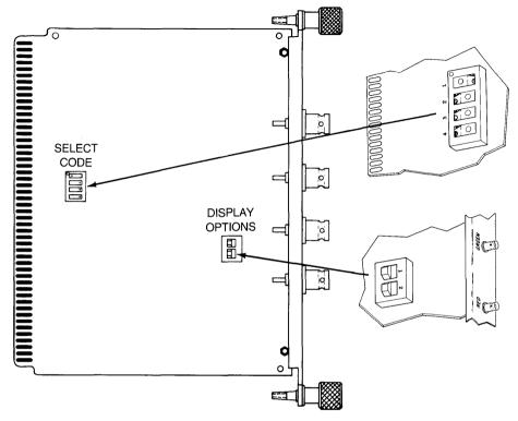
Figure 5-11. HP 98627A Color Video Output Interface Switches
