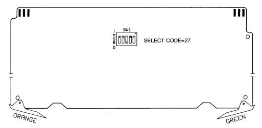
Figure 5-1. EPROM Programmer Interface select code switches.
