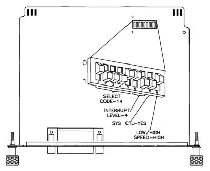
Figure 5-9. HP 98625B Disc Interface switches.
