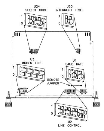
Figure 5-10. HP 98626A RS-232C Serial Interface Switches
