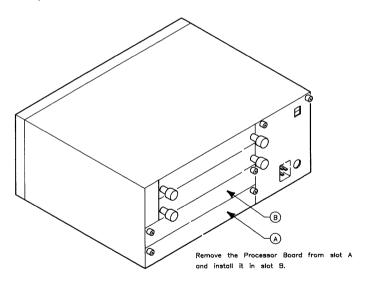
Figure 5-20. Processor Board Placement
