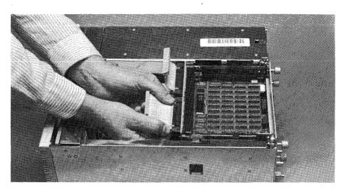
Installing the Two Cables
