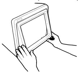
Figure 10-6. Attaching HP Touch.
