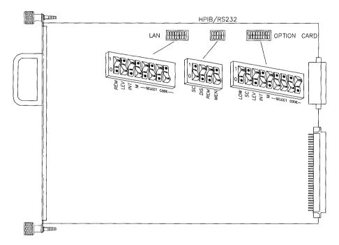
Figure 5-19. Human (System) Interface board switches
