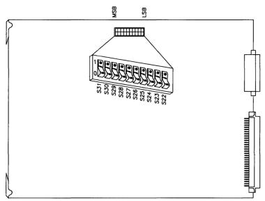
Figure 3-3. Built-in RAM switch settings
