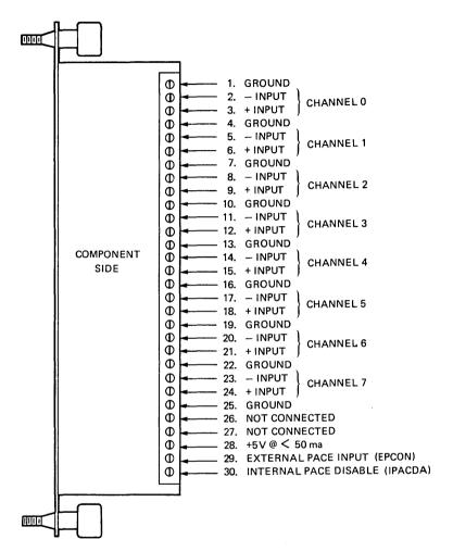
Figure 5-15. Wire termination inputs.
