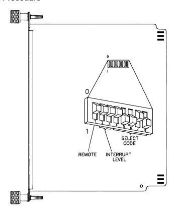
Figure 5-16. HP 98642A 4-Channel Multiplexer Interface switches.
