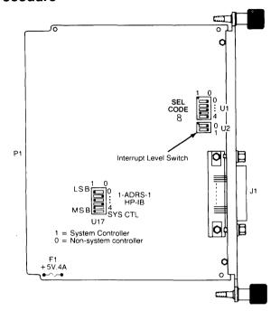
Figure 5-7. HP 98624A HP-IB Interface switches.
