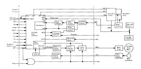
Tape Cartridge Block Diagram
