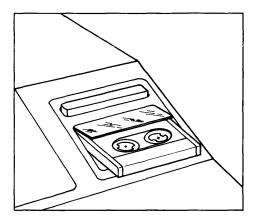
To remove the tape cartridge, press the eject bar. If it is pulled out without pressing the eject bar, another catridge cannot be inserted until the eject bar is pressed. Do not remove the tape or execute reset while it is moving; damage to the tape may result.
