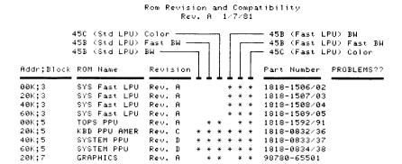
To check for problems, first find your particular machine configuration at the top of the report (9845B (Fast LPU) Fast Black & White, for instance). Then check that column to see if it is filled with asterisks (\*'s). If one or more are missing, or if there are any messages under "PROB-LEMS??", refer to the troubleshooting section.
