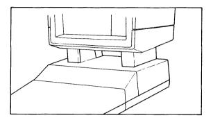
Now push the sliding lock handles in, to secure the CRT to the mainframe.
