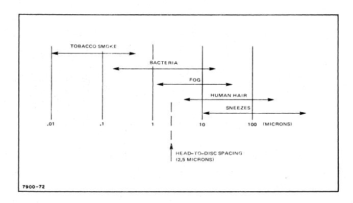
There are particles in the air in almost every environment. The chart above shows the range of particle size which can be found. Note that the head to disc spacing is 2.5 microns.
