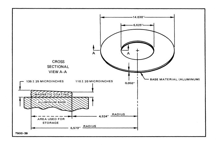
The medium of storage in a disc drive is a thin layer of magnetic material. This magnetic material (ferromagnetic iron oxide) is bonded to both sides of an aluminum disc. Ferromagnetic iron oxide is used because:
