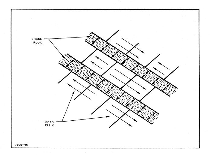
Current state-of-the-art disc drives, including the HP 7900A, use the straddle erase technique. The results of this are illustrated above. The direction of erase magnetization on the surface of the disc is perpendicular to the direction of data magnetization. The erase flux will not affect the data flux, even if the head is not centered on the data track.
