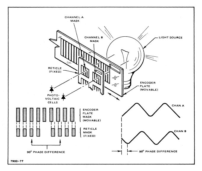
Carriage position detection is accomplished by means of an optical encoder. The encoder provides two channels of position information which are separated in time by 90°. The information is detected by sensing a value of light from a fixed source through a reticle and encoder plate. A third channel of information is used to sense CYLINDER ZERO or HOME POSITION.
