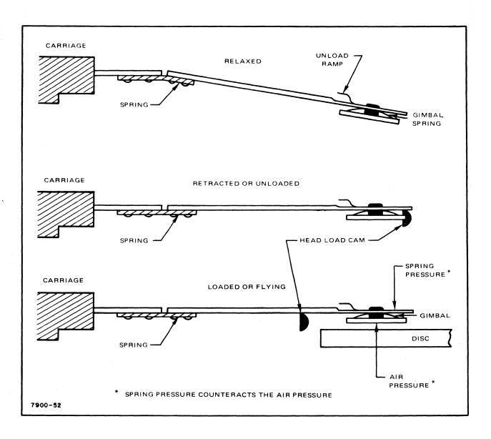
A layer of moving air caused by rotating the disc is used to support the head over the disc surface. The aerodynamic characteristics of the shoe tend to force the head away from the surface while spring tension on the arm counteracts, causing the head to fly at the desired height.
