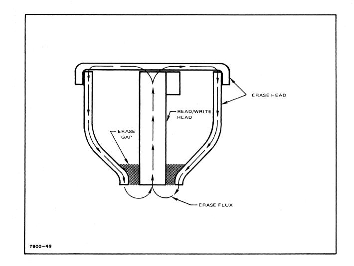
The erase head "straddles" the read/write head. As the figure shows, the read/write head is part of the path for erase flux. The resulting erase magnetization of the disc surface is perpendicular to the direction of data magnetization. The placement of the erase gaps with respect to the write gap is such that erasing occurs after writing.
