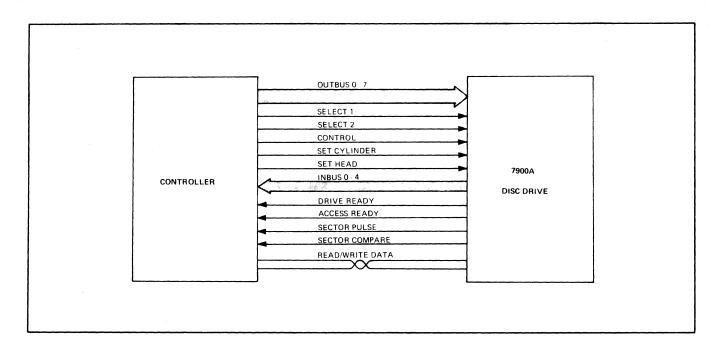
Operation of the 7900A Disc Drive is the responsibility of a controller. The controller resides logically between the CPU and the disc drive. Its function is to receive commands from the CPU and translate them into a form that the disc drive can use. Communication between the controller and disc drive is accomplished over outbus lines (8), inbus lines (5), status information lines, select lines, data lines, and drive control lines.
