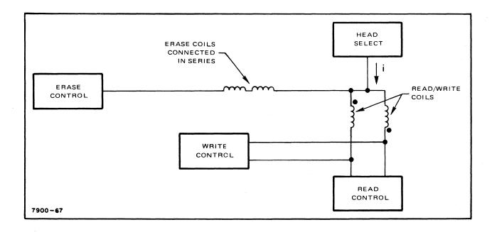
The central element in the DATA CONTROL section of the disc drive is the head assembly. There is one head for each disc surface, each of which consists of an erase element and a read/write element mounted in a ceramic shoe. The shoe is contoured to fly over the disc surface supported by a cushion of moving air. The coils in the head assembly are electrically connected as shown.
