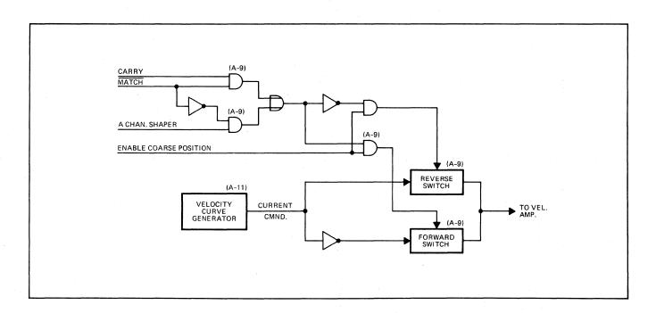
The Direction Control circuitry is used to gate the proper polarity velocity command to the Servo Amplifier.
