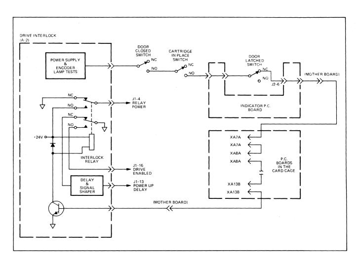
The purpose of the drive enable circuitry is to provide a safety interlock system. To satisfy the interlock system, the following conditions must be met:
