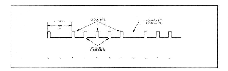
Data transfer to or from a disc is accomplished in serial fashion. That is, one BIT at a time as opposed to parallel data, which transfers 8 bits (one byte) at a time. To accomplish this transfer, data is "clocked" in a "bit cell". Clock bits are present every 400 n-seconds. A bit between the clock bits represents a logic 1 and the absence of a bit represents a logic zero. Consequently, an all one record is twice the density (twice the number of flux reversals) as an all zeros record.
