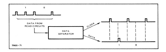
The function of data separation is shown above. Data from the read circuits is a combination of data bits and data recovery clock bits. The data separation must synchronize with the clock pulses and use this synchronization to extract the data. The HP 7900A does not have a data separator within the drive.
