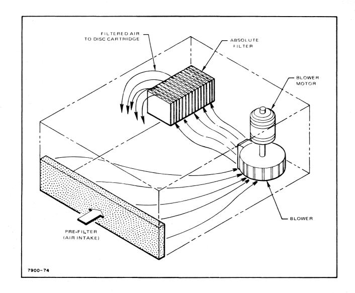
Previous pages have shown the importance of filtering the air which cools and cleans the disc cartridge. Equally important are the details of the implementation.
