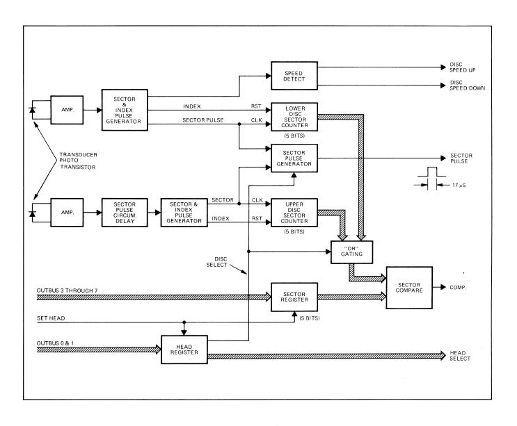
There are two functions performed by the SECTOR DETECT portion of the drive. One function is rotational speed detection and the other is rotational position detection. The same mechanical elements are involved in both functions.
