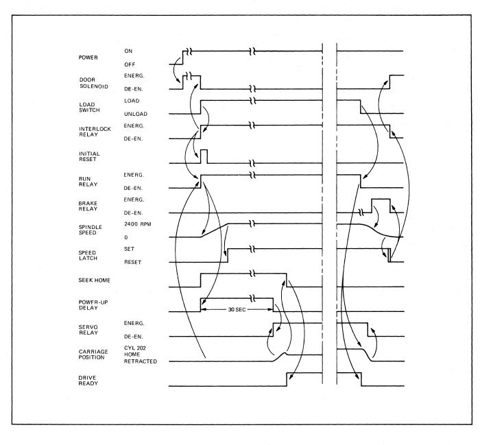
NOTE: The arrows point from the source signal to the result signal, i.e. Power "ON" initiates door solenoid "ENERGIZED".
