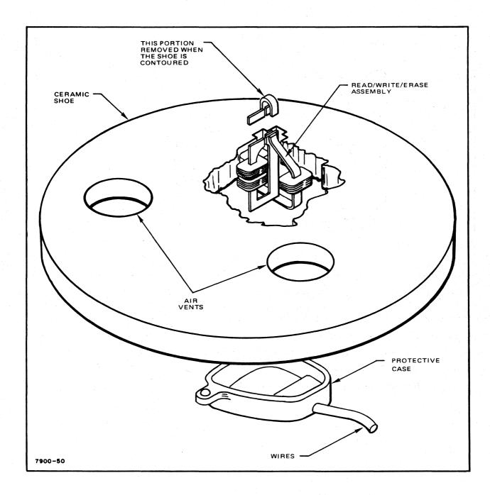
The Read/Write/Erase assembly is then mounted and glued into a ceramic show. The shoe is then contoured and polished to provide an aerodynamic surface which is used to fly the head above the rotating disc surface.
