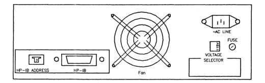
HP 9125S REAR PANEL Figure 3-2 There is only one fuse required for each of the two voltage ranges of 110-120 and 220-240 VAC. The part number for the fuse is 2110-0002.
