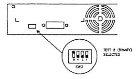
Figure 4-3. Rear view of HP 9122 disc drive.
