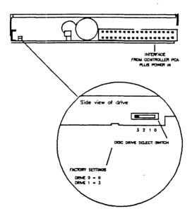
Figure 4-5. Disc Drive Select Switch (09123-69101).
