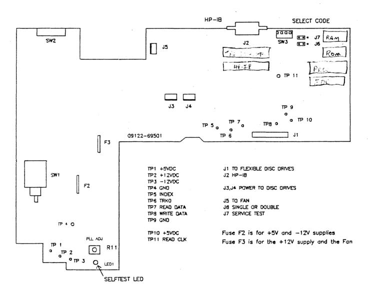
Figure 4-1. Controller and Power Supply PCA(09122-69511)
