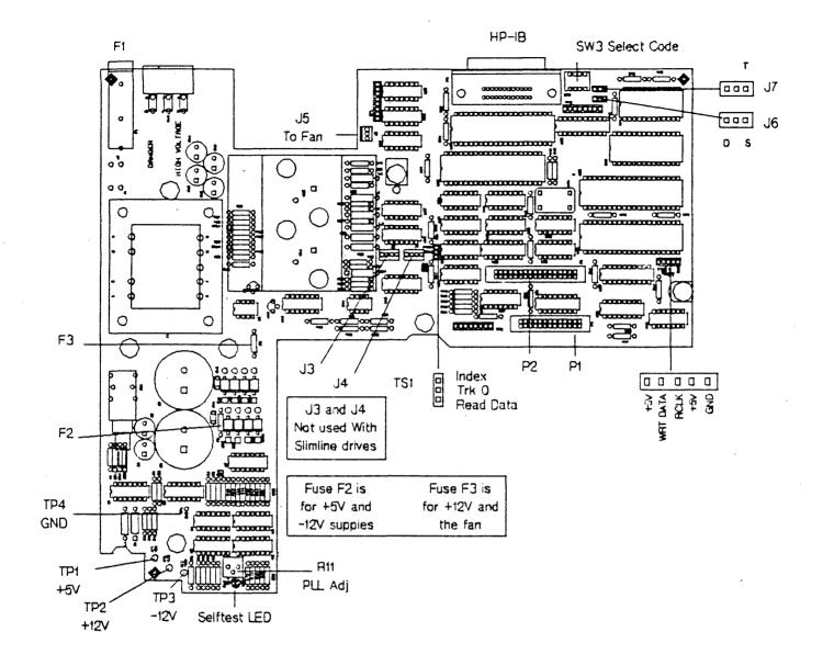
Figure 4-2. Controller and Power Supply PCA (09122-69504)
