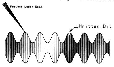
Figure 1: WORM Optical Recording
