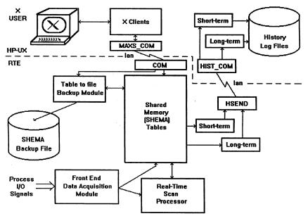
figure 3. Distributed system module layout
