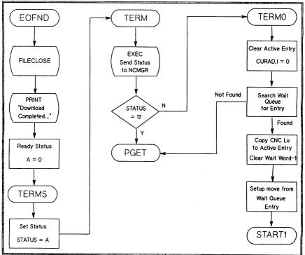
Figure-17. End-Of-File/Termination Section Flowchart
