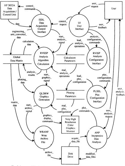
Fig. 2 Integrated Workstation Data Flow Diagram (Context Level)
