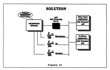
We have given several examples of how the technology is used. Now let's look at how this service is implemented. With Hewlett-Packard, the solution is called Applied Computerized Telephony (ACT). The solution consists of "5 Easy Pieces": 1. Public telephone network - This typically will be one of
