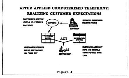
Now lets see what happens when an intelligent link exists between the telephone switch and the computer. We'll take the same example used above and describe how the phone would be handled differently had they had integrated their telephone and computer system with a product like ACT (Applied Computerized Telephony) from HP.
