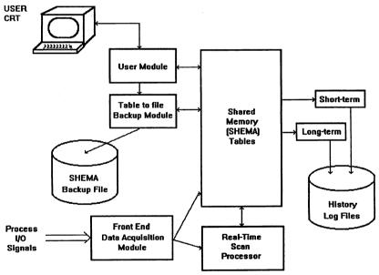
figure 1. Stand-alone system module layout
