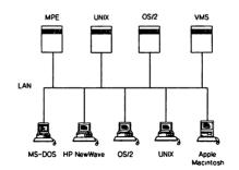
The clients are various types of personal computer. These are connected via a local area network to a range of server minicomputers. For simplicity, printing resources are ignored.
