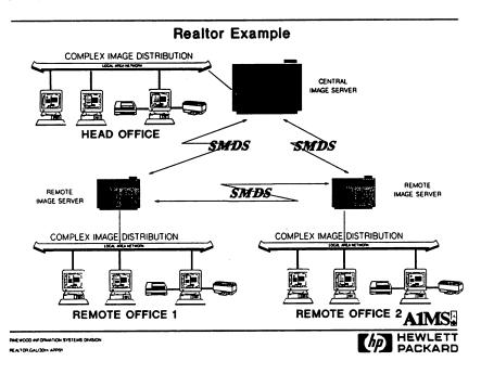
This realty has a head office, with an image server which is used for storing other information as well as images of the properties in the area. Each remote office has a smaller image server which is used to store images of the properties in the area.
