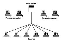
In this environment, all processing and data storage occurs on the host. The terminal provides a simple, single tasking user interface. The cost per user of the terminal hardware is relatively low compared to a personal computer client. However, the host computer must be larger than its server counterpart because of the greater processing and storage requirements. The user is totally dependant upon host availability for any activity.
