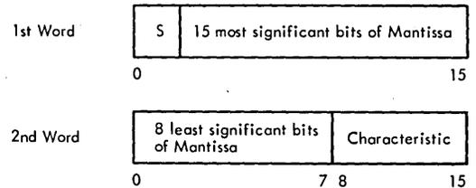
Extended precision provides up to 31 significant bits of precision (9 plus significant digits) stored in core storage as shown below:
