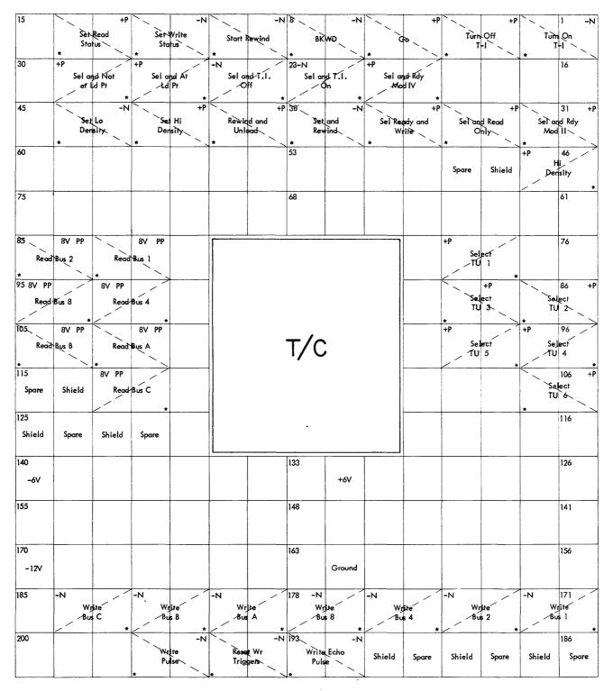
Figure 16. IBM 1401 to IBM 729 Magnetic Tape Unit Connector Receptacle (Wiring Side—Fixed Mount)
