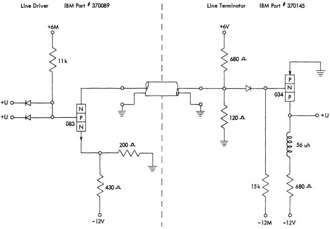
Figure 7. Line Driver and Terminator
