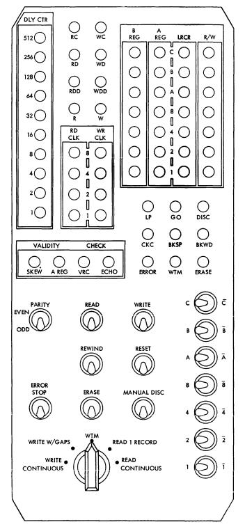
Figure 6. Customer Engineering Diagnostic Panel
