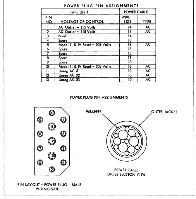
Figure 17. IBM 1401 to IBM 729 Magnetic Tape Unit Power Plug Pin Assignments
