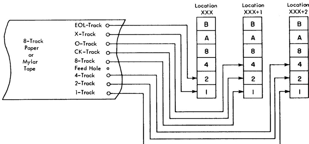
Figure 31. Eight-Track Tape Punching to Bit-Pattern Translation
