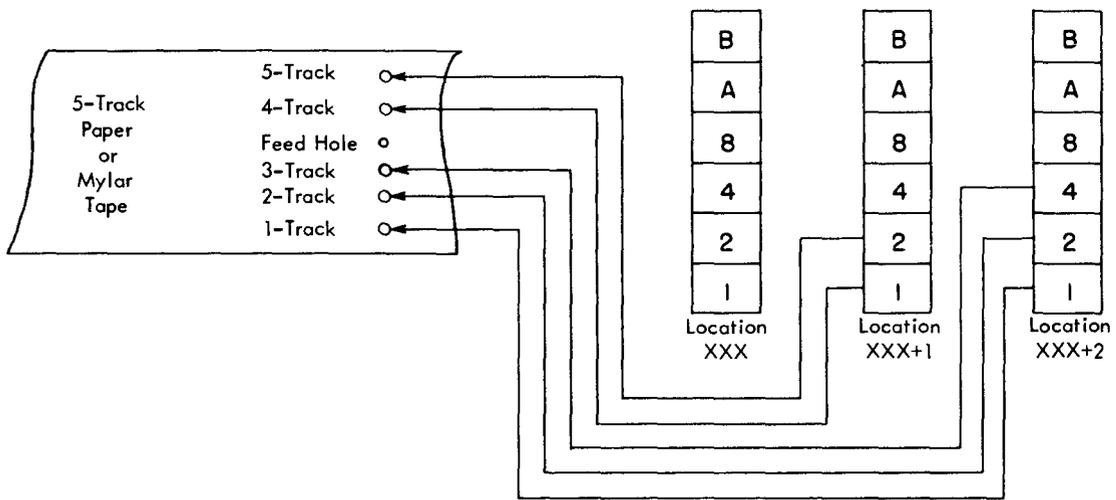
Figure 34. Five-Track Bit Pattern to Tape Punching Translation
