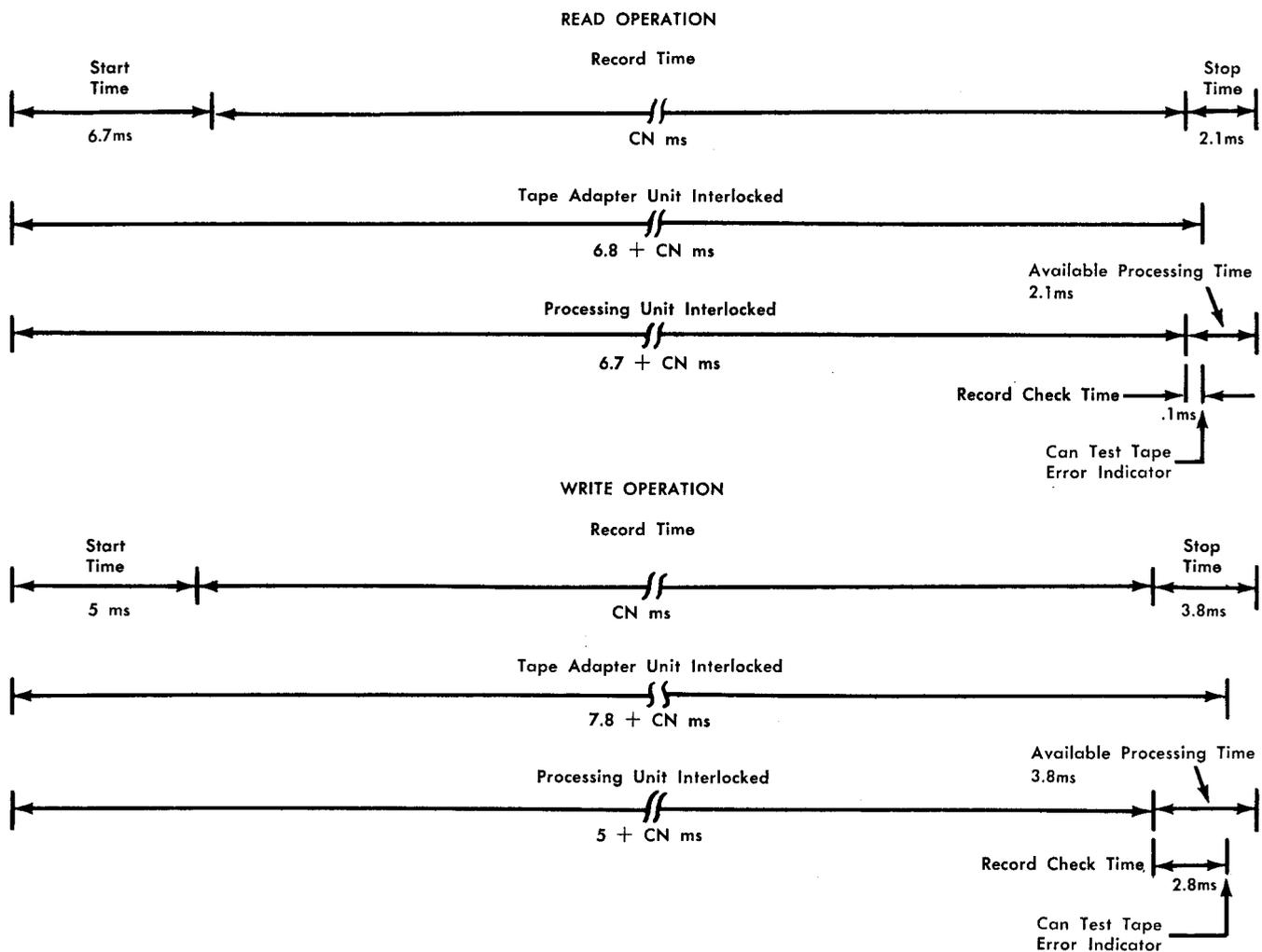
Figure 20. IBM 729, Model VI, Read-Write Operation Timings
