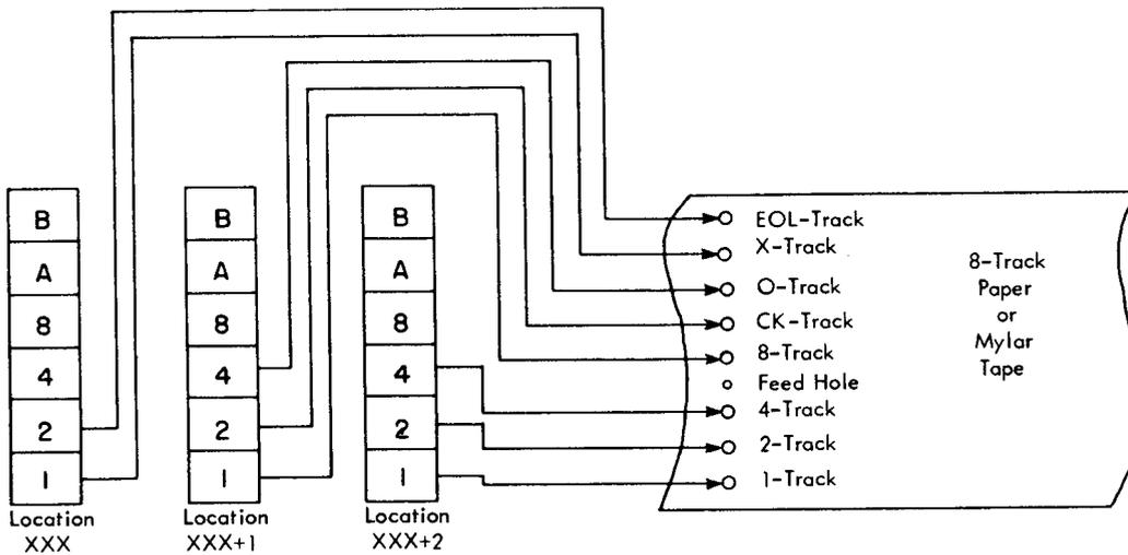
Figure 30. Eight-Track Bit Pattern to Tape Punching Translation
