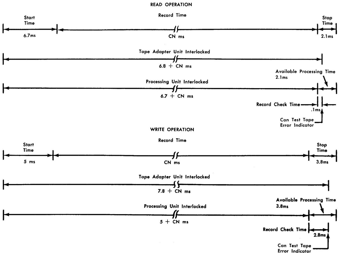
Figure 18. IBM 729, Model IV, Read-Write Operation Timings
