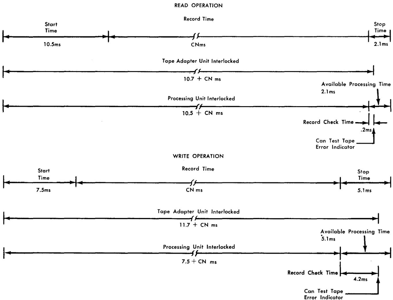
Figure 19. IBM 729, Model V, Read-Write Operation Timings
