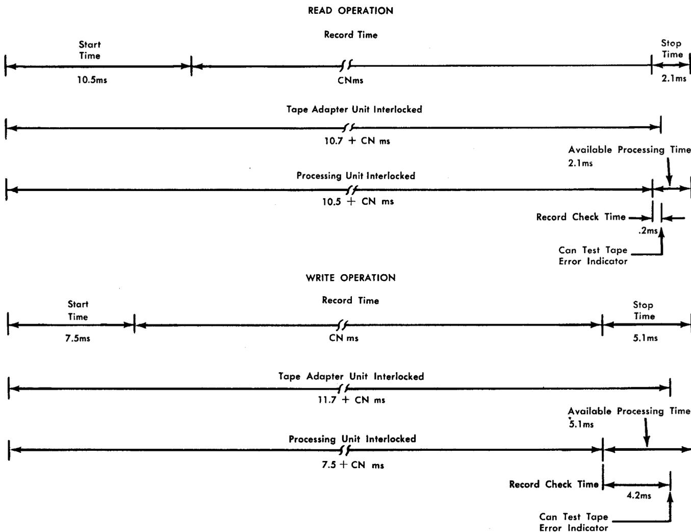
Figure 17. IBM 729, Model II, Read-Write Operation Timings
