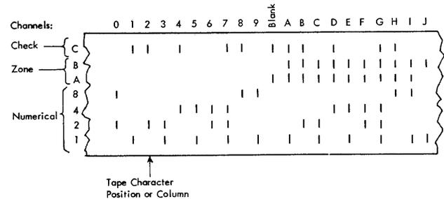
Figure 1. Magnetic Tape Data in the BCD Code
