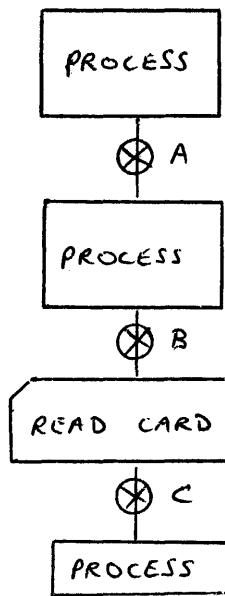
A and C would only branch control to the printer program if the Printer and Carriage were not busy. B would branch unconditionally to the printer program. This might not utilise some of the available process time, but would ensure that the card read operation occurred as soon as control was returned by the printer program, and thus that the printer was not held up by the card read.
