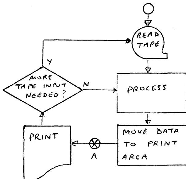
The exit to the process program would occur at point A - this ensures that when the process program returns control to the printer program (at point A), the next print instruction is given as soon as possible.
