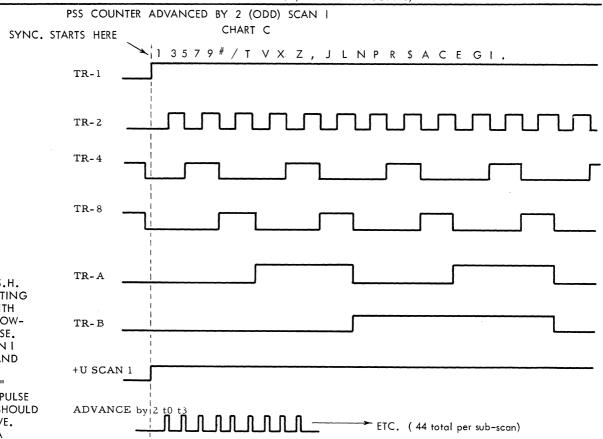
1. JUMPER (REFER TO S.H. 58) TO ALLOW PRINTING TO BEGIN ONLY WITH THE PSS PULSE FOLLOW-ING THE HOME PULSE. SYNC. ON +U SCAN I GOING POSITIVE AND PRINT. TRIGGER I SHOULD TURN "ON" WITH THE FIRST PSS PULSE AND THE PATTERN SHOULD BE AS SHOWN ABOVE. EACH DIVISION IS A CLOCK CYCLE. (II.I MICSECONDS)
