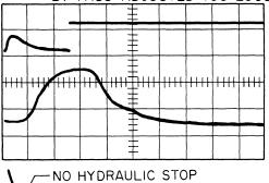
FIG. II BY-PASS ADJUSTED CORRECTLY
