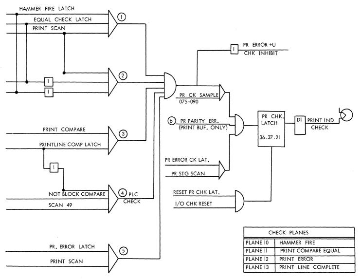
NON BUFFER PRINT CHECK CKTS. ARE SIMILAR TO THE PRINT BUFFER SYSTEM. SOME OF THE DIFFERENCES ARE NOTED.
