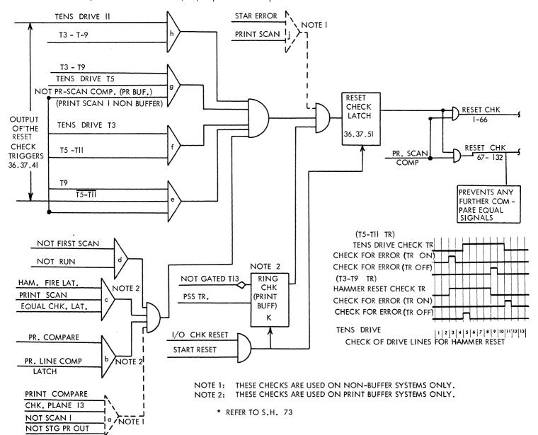
S.H. 74 PRINT CHECKS CAUSED BY NOISE
