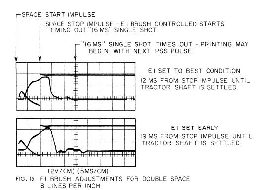
NOTE: Final setting of emitter adjustment arm should be for the least time from the stop impulse until the tractor shaft movement is settled, compromised between triple space six lines per inch and double space eight lines per inch.
