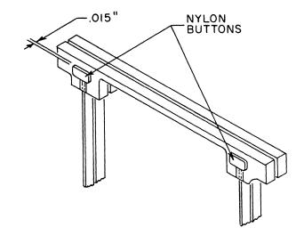
The button hammer assemblies must not be intermixed with non-button Hammer Assemblies 474805 (alpha-numeric) or 475486 (numeric), or increased hammer spring breakage may occur. Field changeover to the new assemblies is not necessary.
