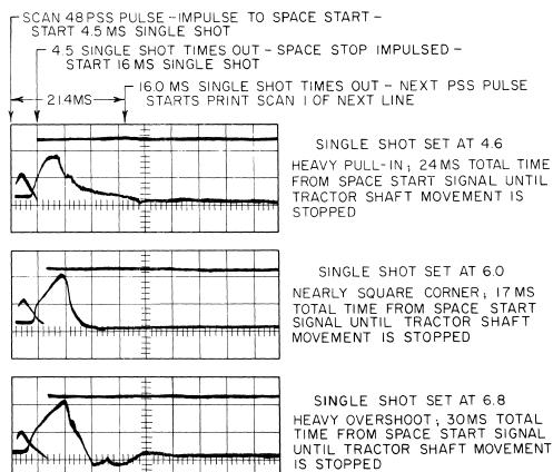
FIG. 13 SINGLE SPACE - 6 LINES PER INCH ADJUSTMENTS OF THE 4.5 MS SINGLE SHOT
