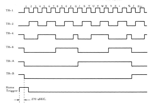
I. DO NOT PRINT: SYNC ON HOME TRIGGER GOING POSITIVE. COUNTER SHOULD ADVANCE BY I EVERY THIRD PSS PULSE (PSS PULSE ASSOCIATED WITH A SUB SCAN I. PATTERN SHOULD BE AS SHOWN EACH DIVISION REPRESENTS 3 SUB-SCANS (I.65 MILLISECONDS).
