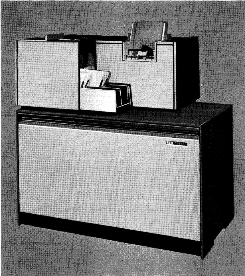
Figure 1. IBM 1442 Card Read-Punch
