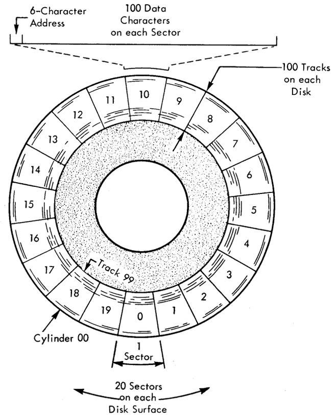
Figure 12. Arrangement of Data on Disk Surface
