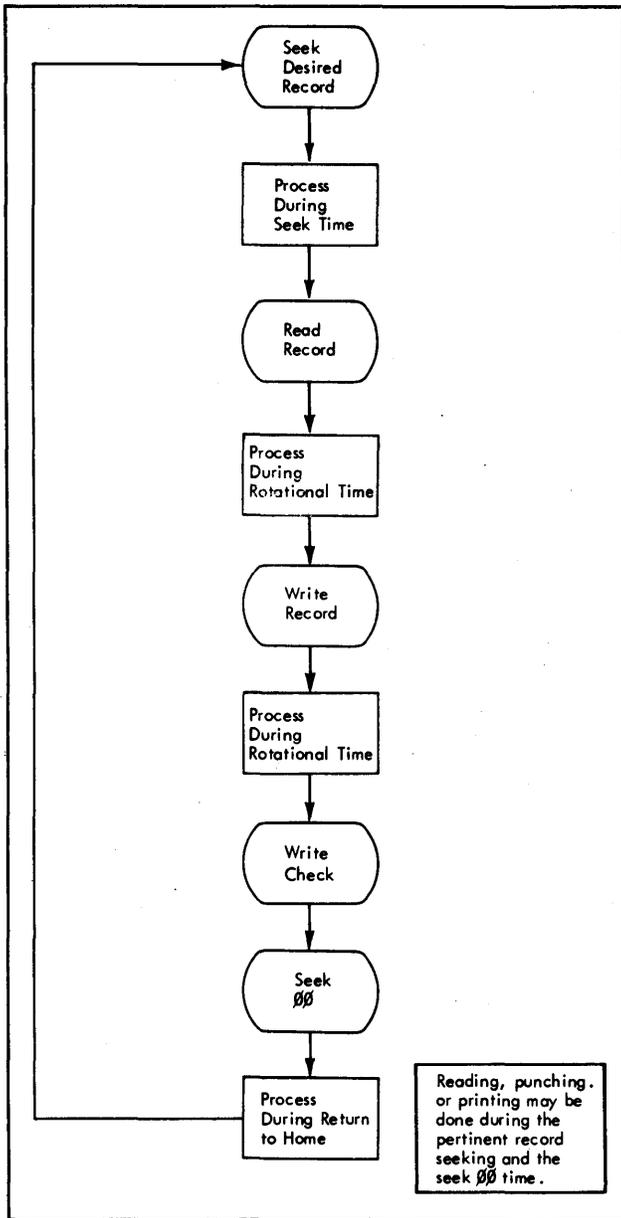
Figure 42. Block Diagram for Dummy Seek Technique
