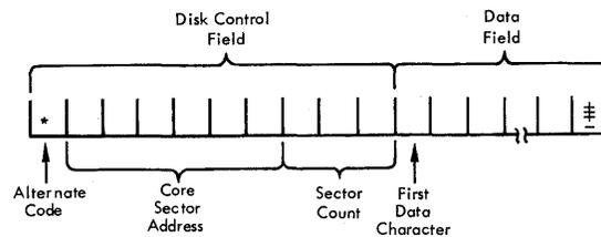
The *core sector address* portion of the disk control field contains the disk address of the data to be read or written. If more than one sector is read or written, the address of the first sector is specified.
