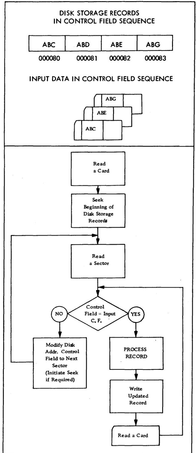
Figure 23. Abbreviated Block Diagram of Consecutive Processing Approach
