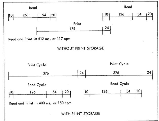
Figure 37. Listing with 1443 Printer, Model 1, 52 Character Set and 1442 Card Read Punch, Model 1
