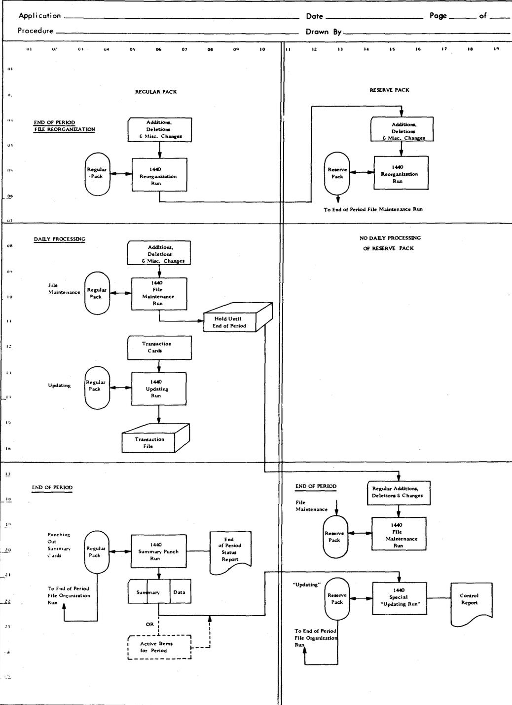
Figure 26. Overall Flowchart: Reserve Pack and Summary Punchout Technique (Also Active Record Punchout Technique)
