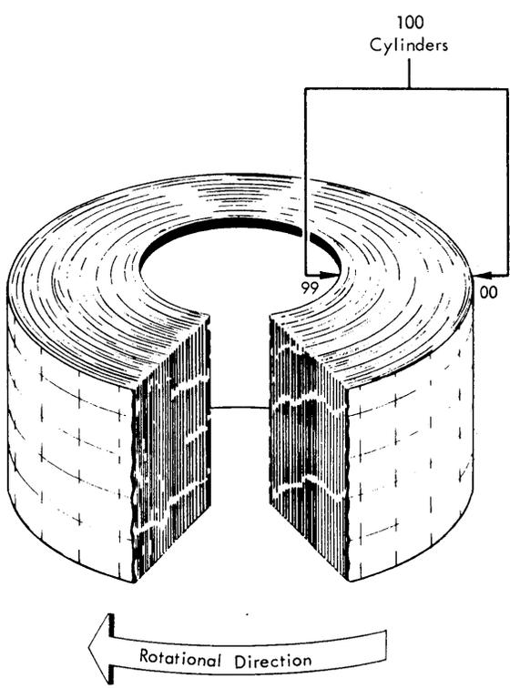
Figure 13. Visualization of Cylinder Concept
