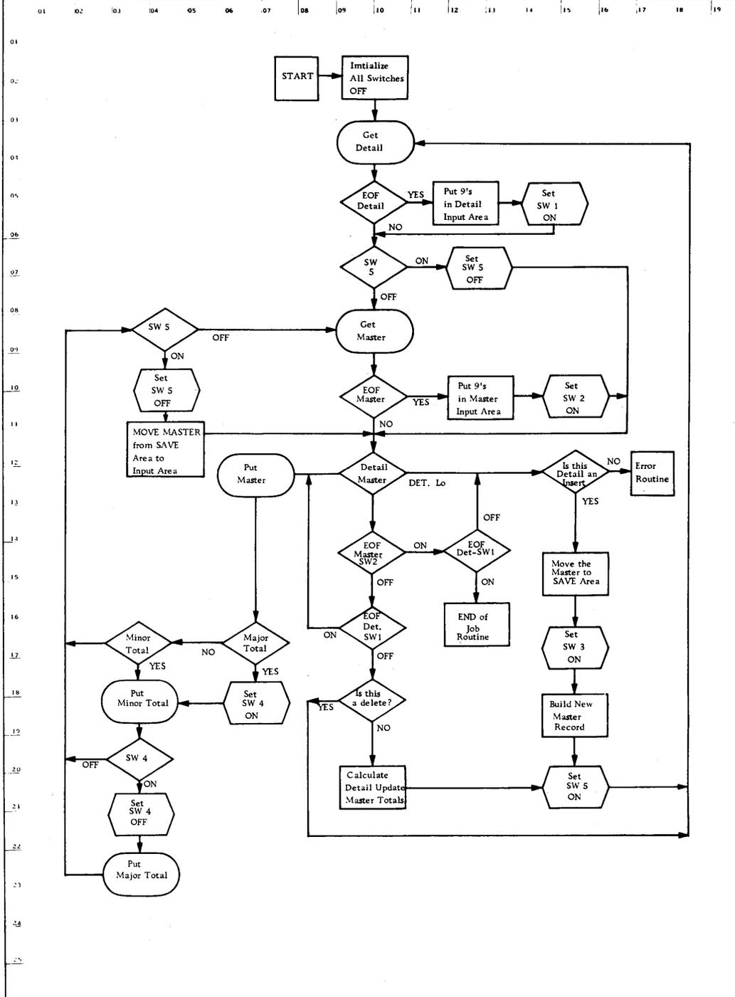
Figure 9. Illustrative General Logic Block Diagram
