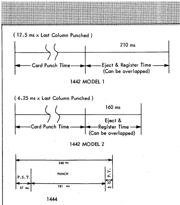
Figure 32. Punch Cycles (Punch and Feed Instruction Used)
