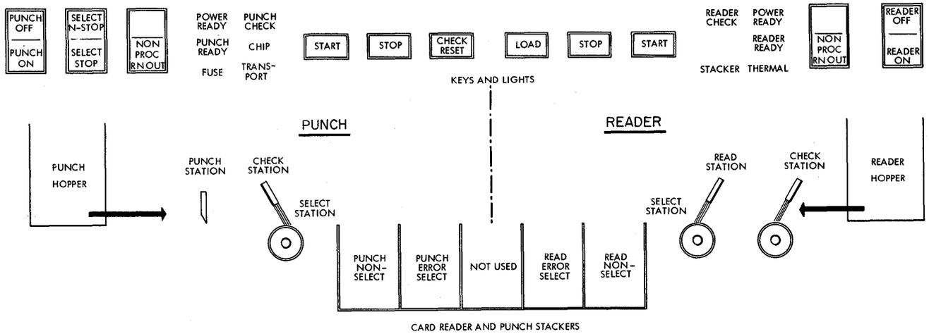
Figure 5. 1622 Keys, Lights, and Card Feed
