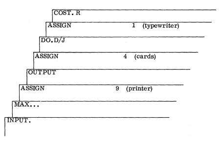
The agenda above would put the normal OUTPUT on the printer, the  $D_j$ 's (reduced costs) on cards, and the cost ranges on the typewriter. Note that any INPUT. card will reinitialize the output unit to card. For assigning output devices for the iteration log and the agenda log see "ASSIGN".
