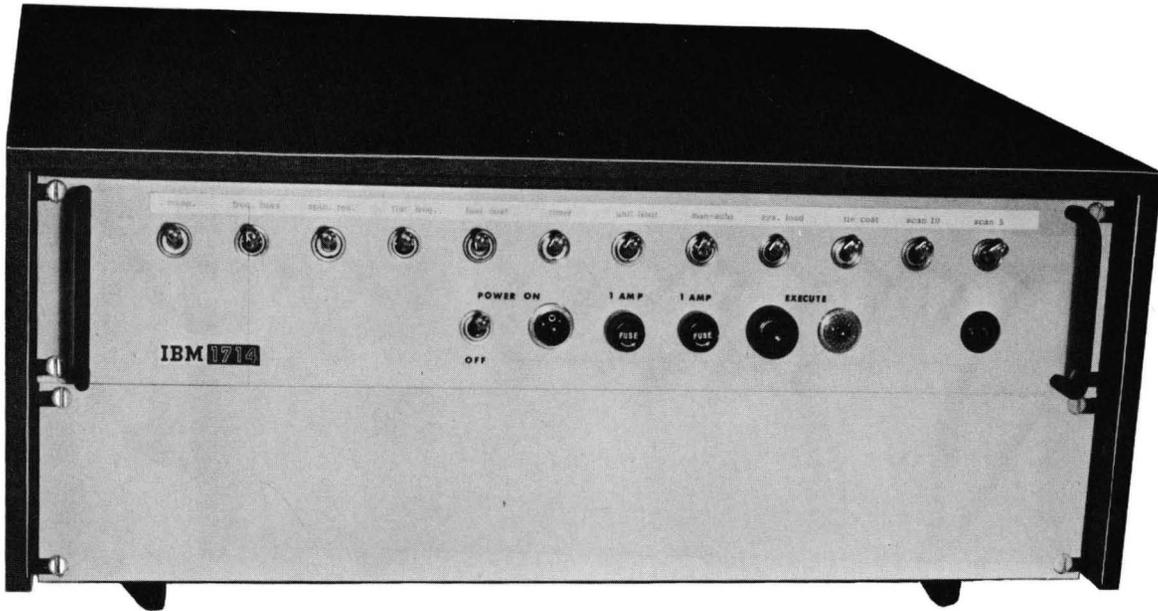
Figure 22. IBM 1714 Sense Switch Unit
