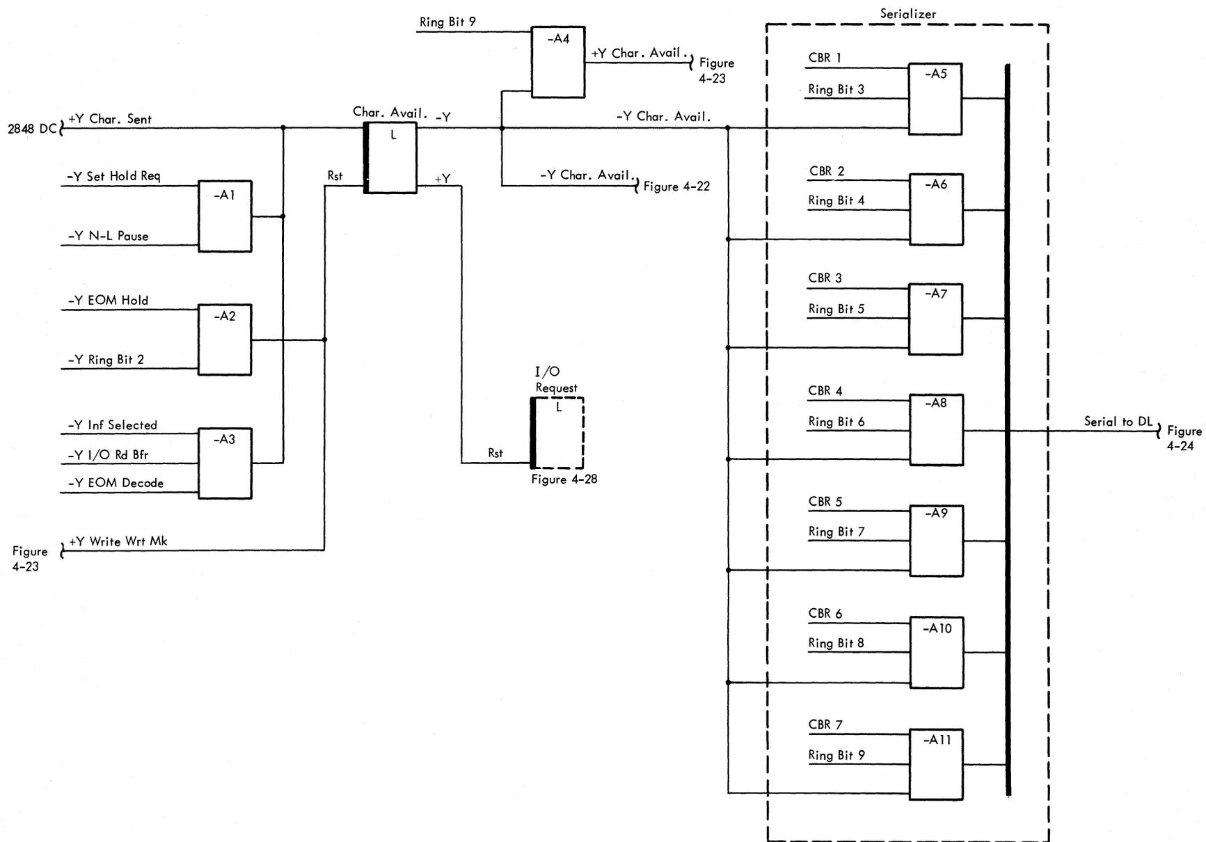
Figure 4-31. Read Operation - Common Buffer to Serializer Transfer
