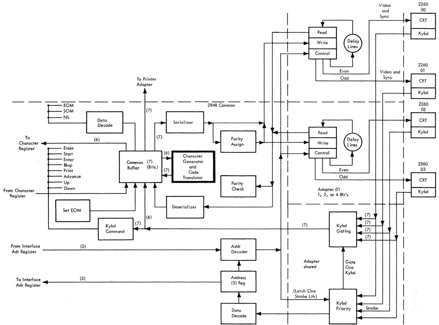
Figure 2-22. Display Control, Simplified Block Diagram
