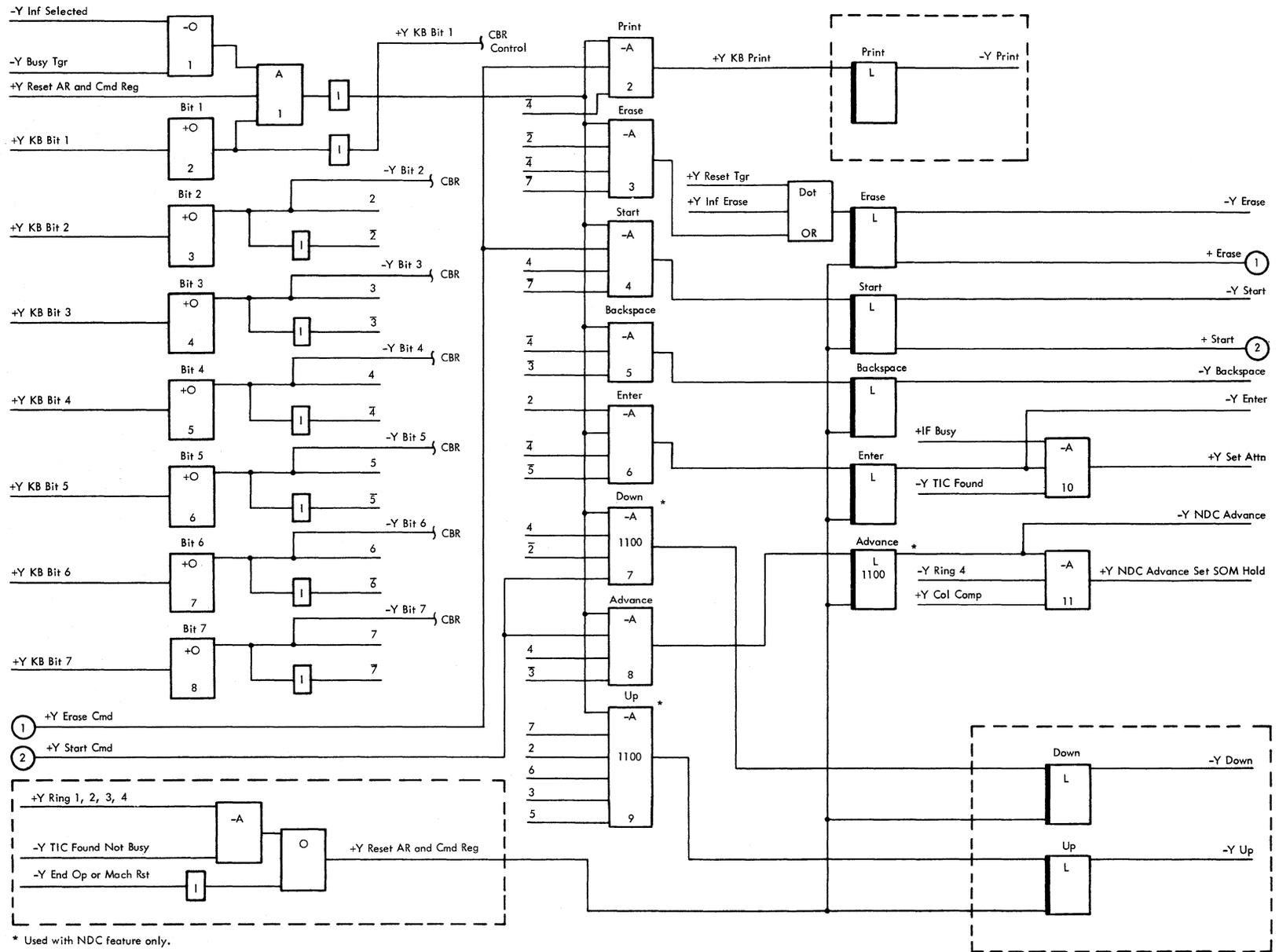
Figure 2-85. Keyboard Command Decoder and Command Latches
