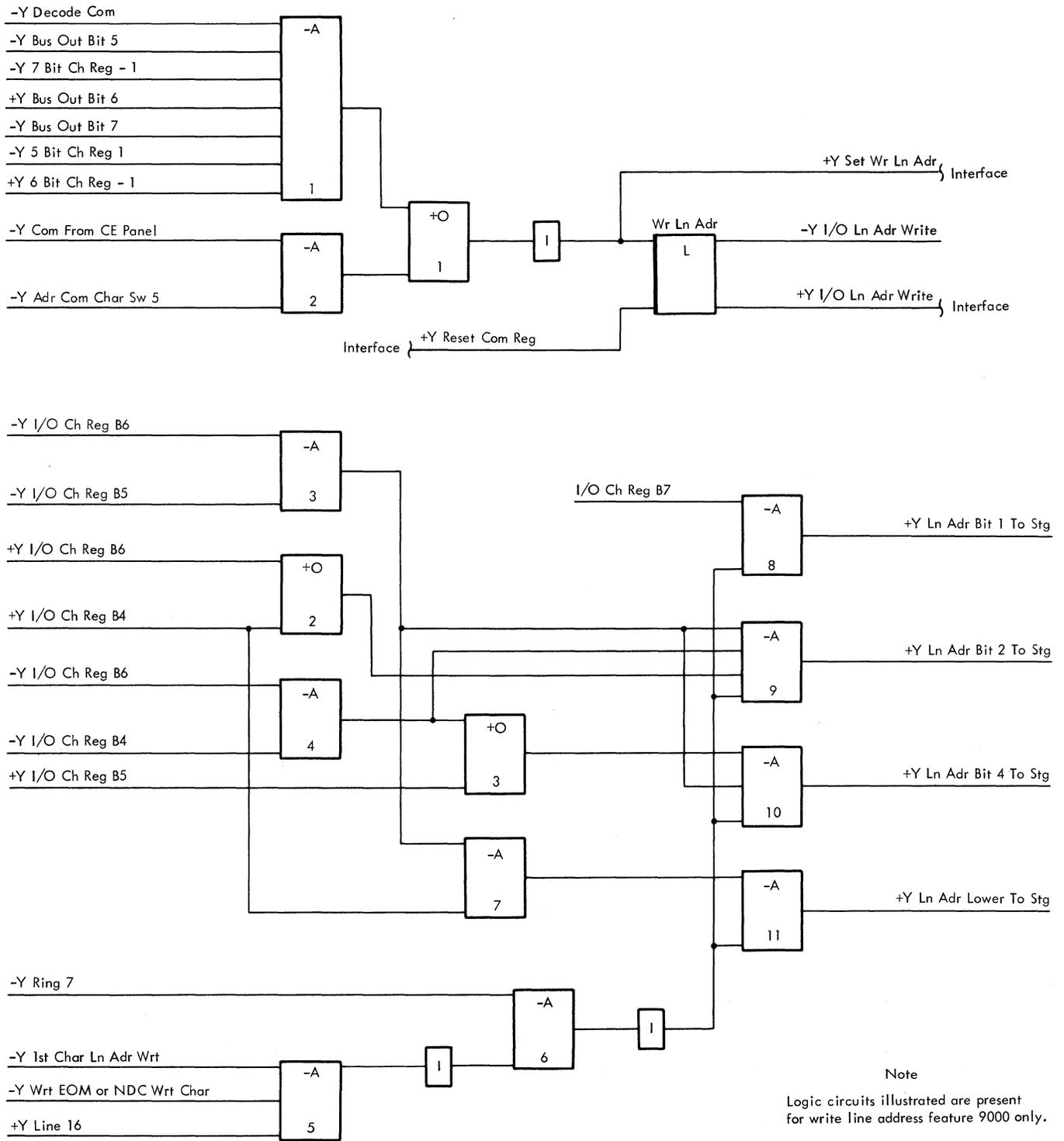
Figure 2-83. Write DS Line Address Decode and Gating
