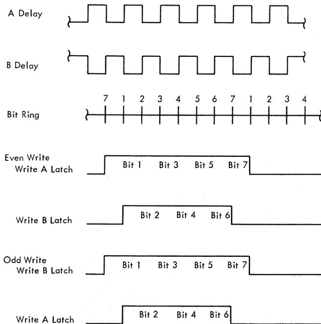
Figure 2-52. Write A and Write B Latches, Timing Chart
