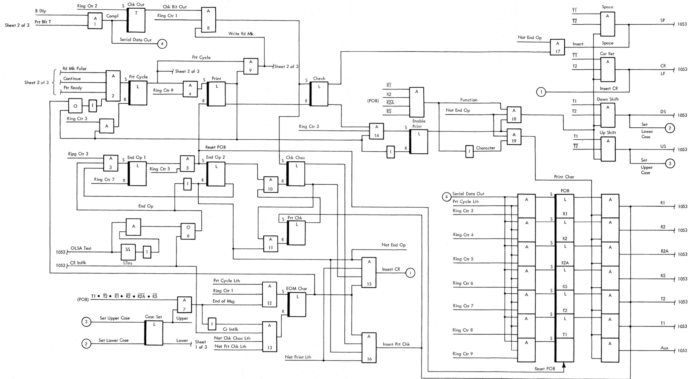
Figure 2-117. Printer Adapter, Logic Diagram (Sheet 3 of 3)
