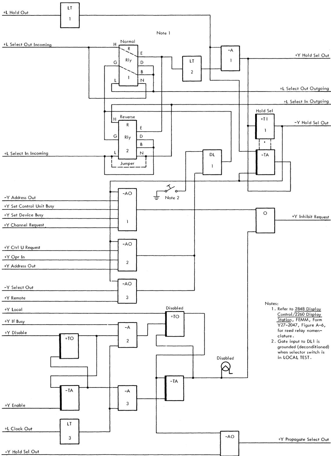
Figure 2-96A. Hold-Select Circuit for Units Equipped with Isolation Feature
