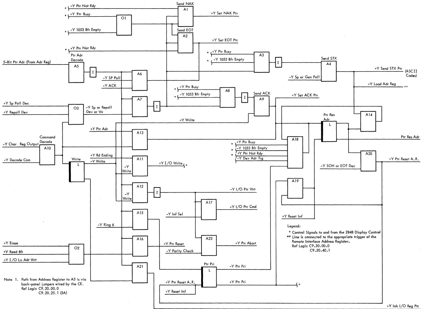
Figure 4-26. Write Printer Control
