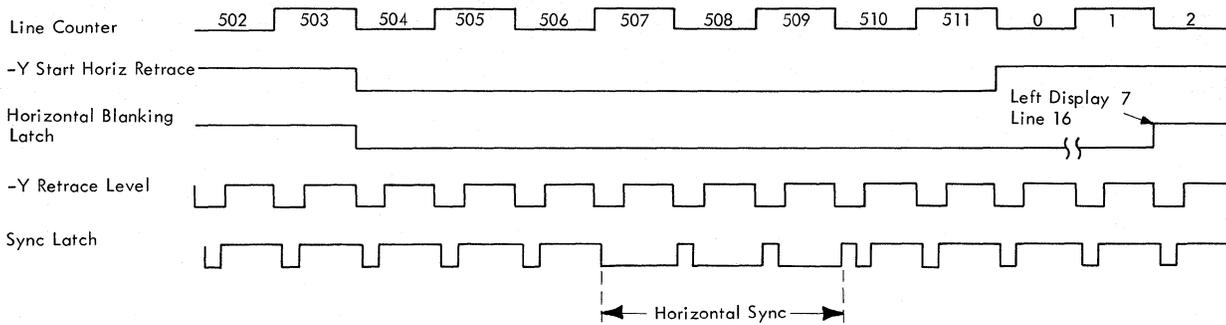
Figure 2-43. Sync Generator Timing
