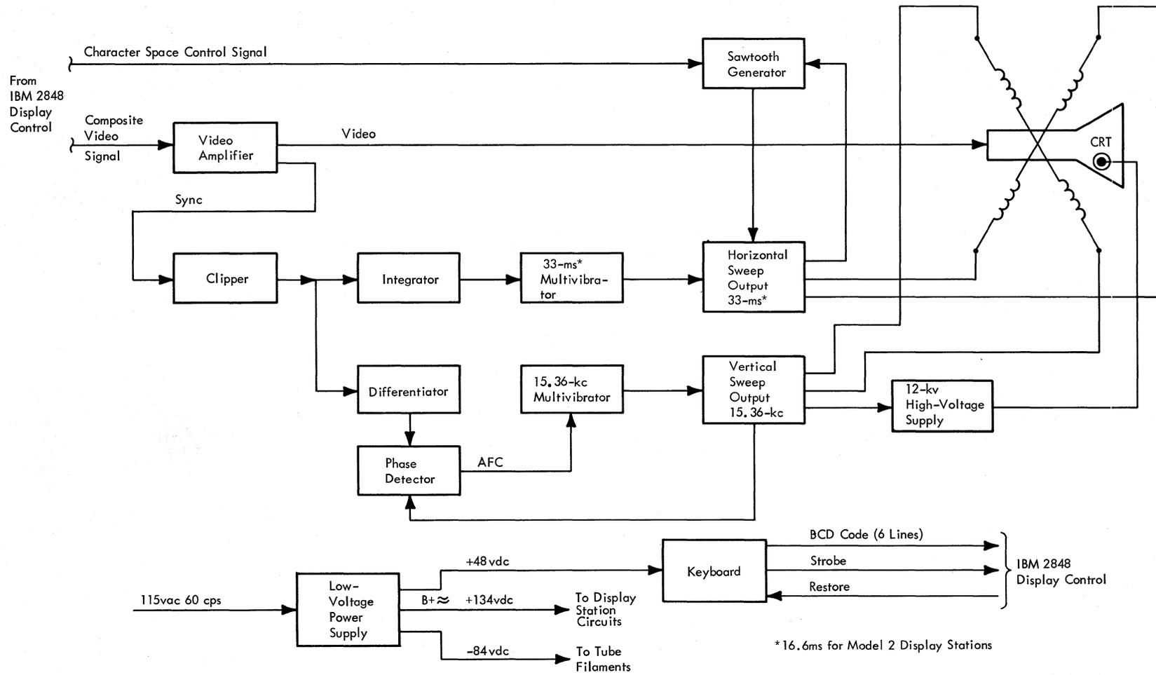
Figure 2-1. Display Station Block Diagram
