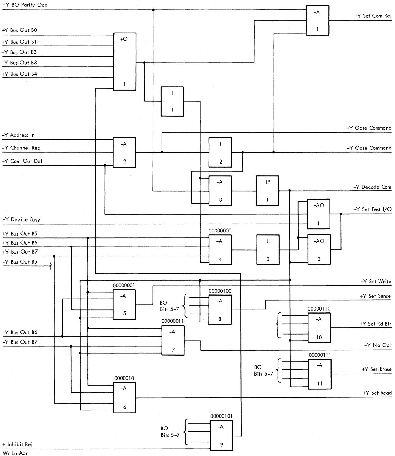
Figure 2-99. Command Decode
