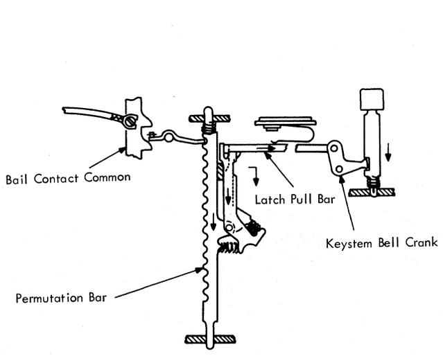
Figure 2-12. Permutation Bar and Keyboard Latch (Normal)
