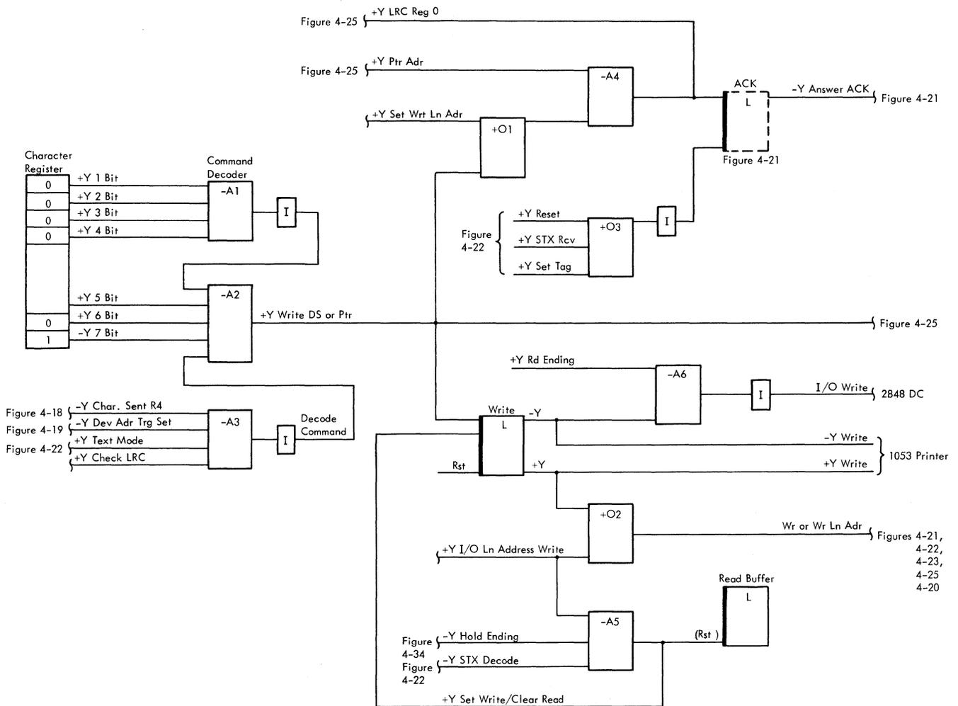
Figure 4-20. Channel Response - Command Character Decode
