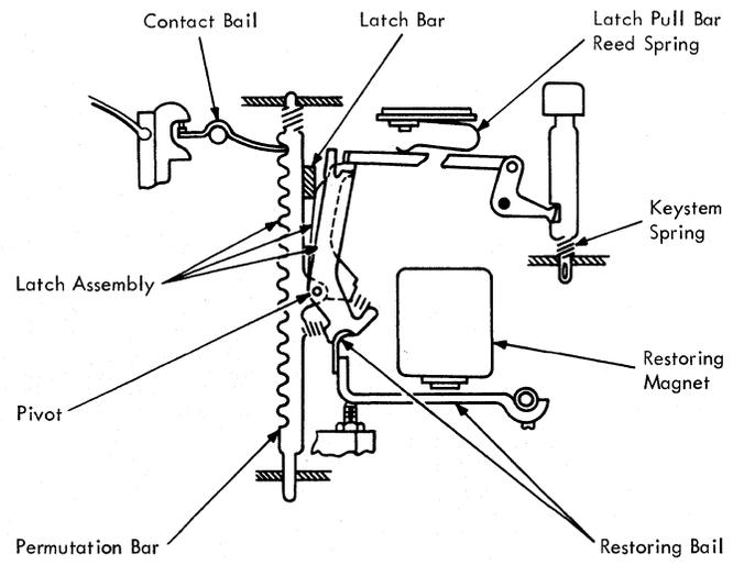
Figure 2-13. Permutation Bar and Keyboard Latch (Tripped)
