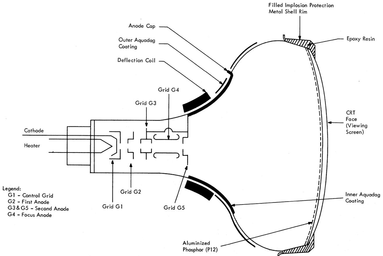
Figure 2-3. Cathode-Ray Tube
