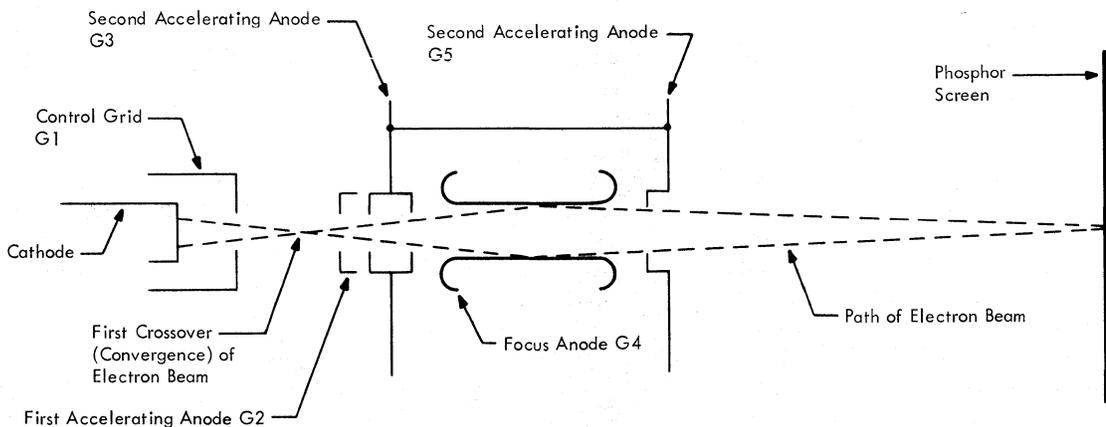
Figure 2-4. CRT Electron Gun
