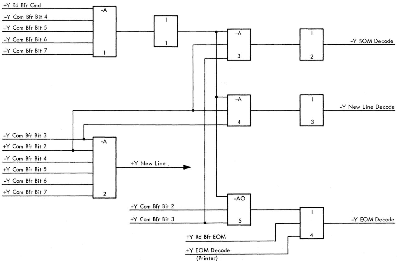
Figure 2-62. SOM, New Line, and EOM Decode Circuit
