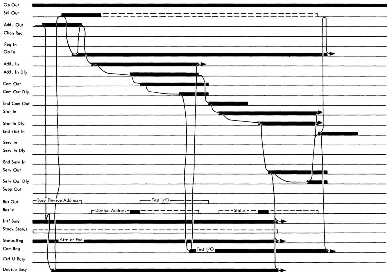
Figure 2-109. Test I/O To Busy Device
