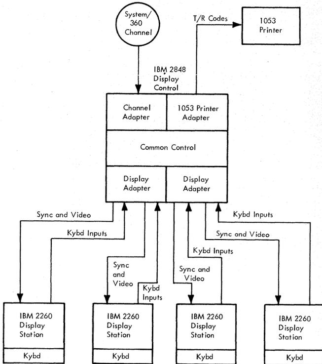
Figure 1-5. IBM 2848 - IBM 2260 Display Complex, Block Diagram
