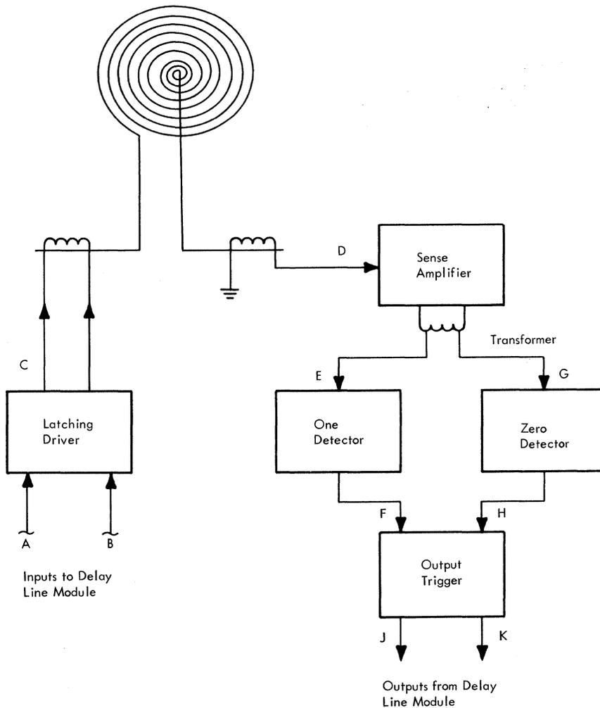
Figure 2-24. Delay Line Module, Simplified Block Diagram
