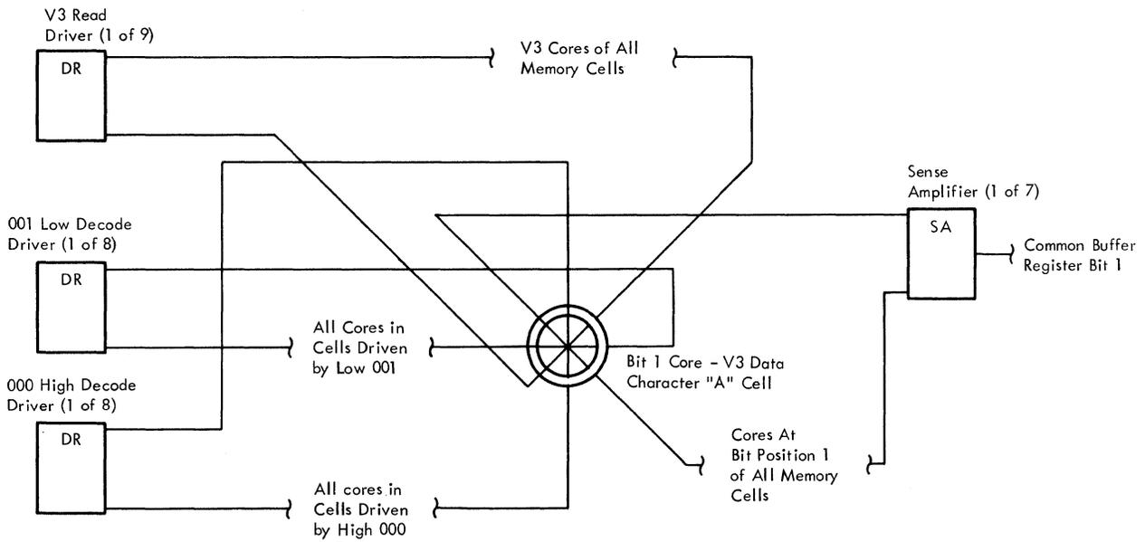
Figure 2-67. Selection, Read, and Sense Winding Connections
