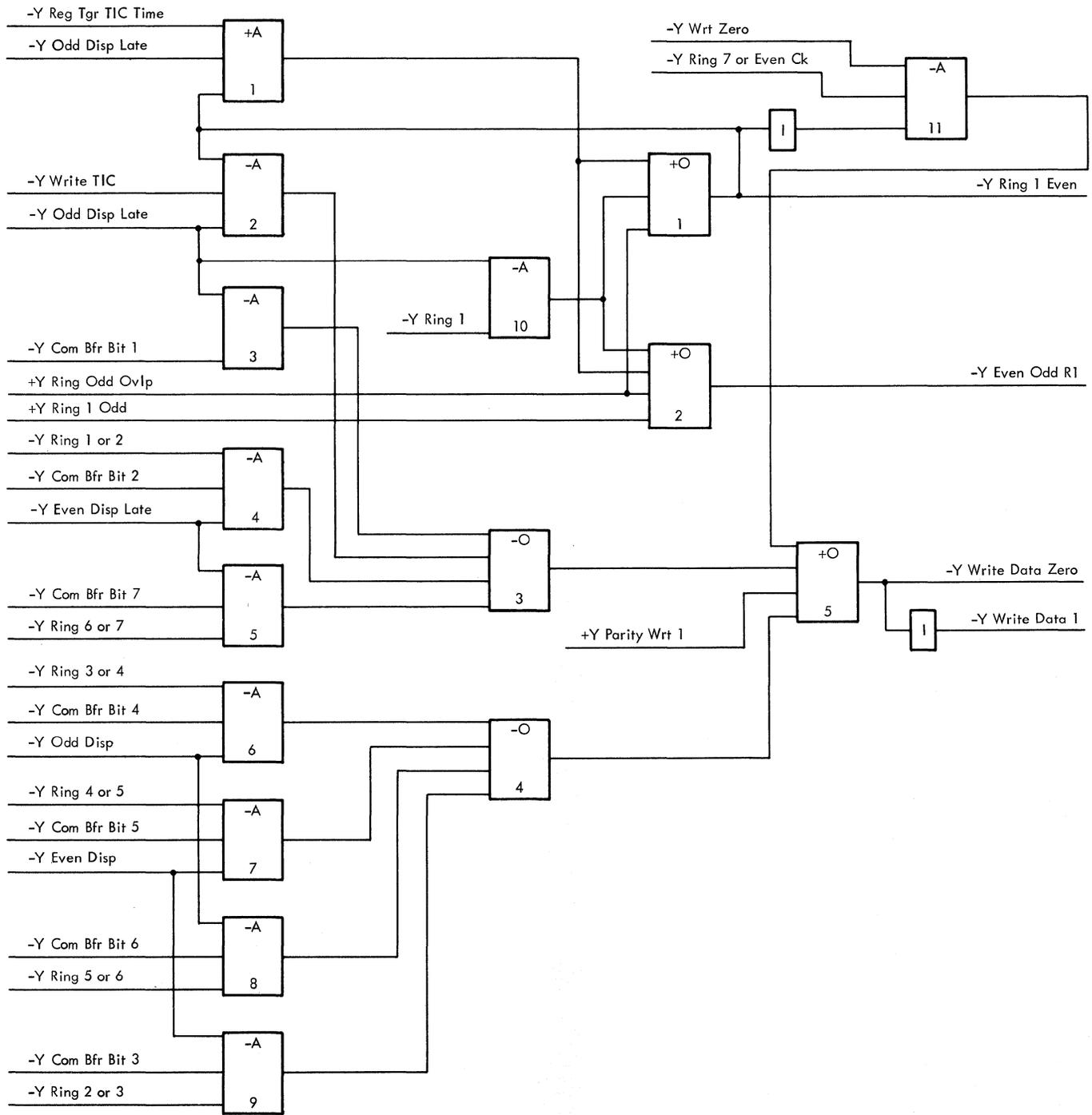
Figure 2-55. Serializer, A Delay
