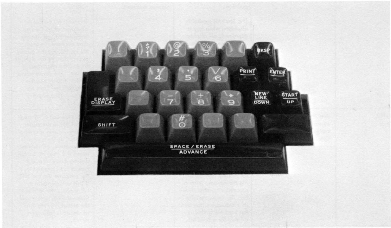
Figure 6-6. 2260 Display Station Numeric Keyboard
