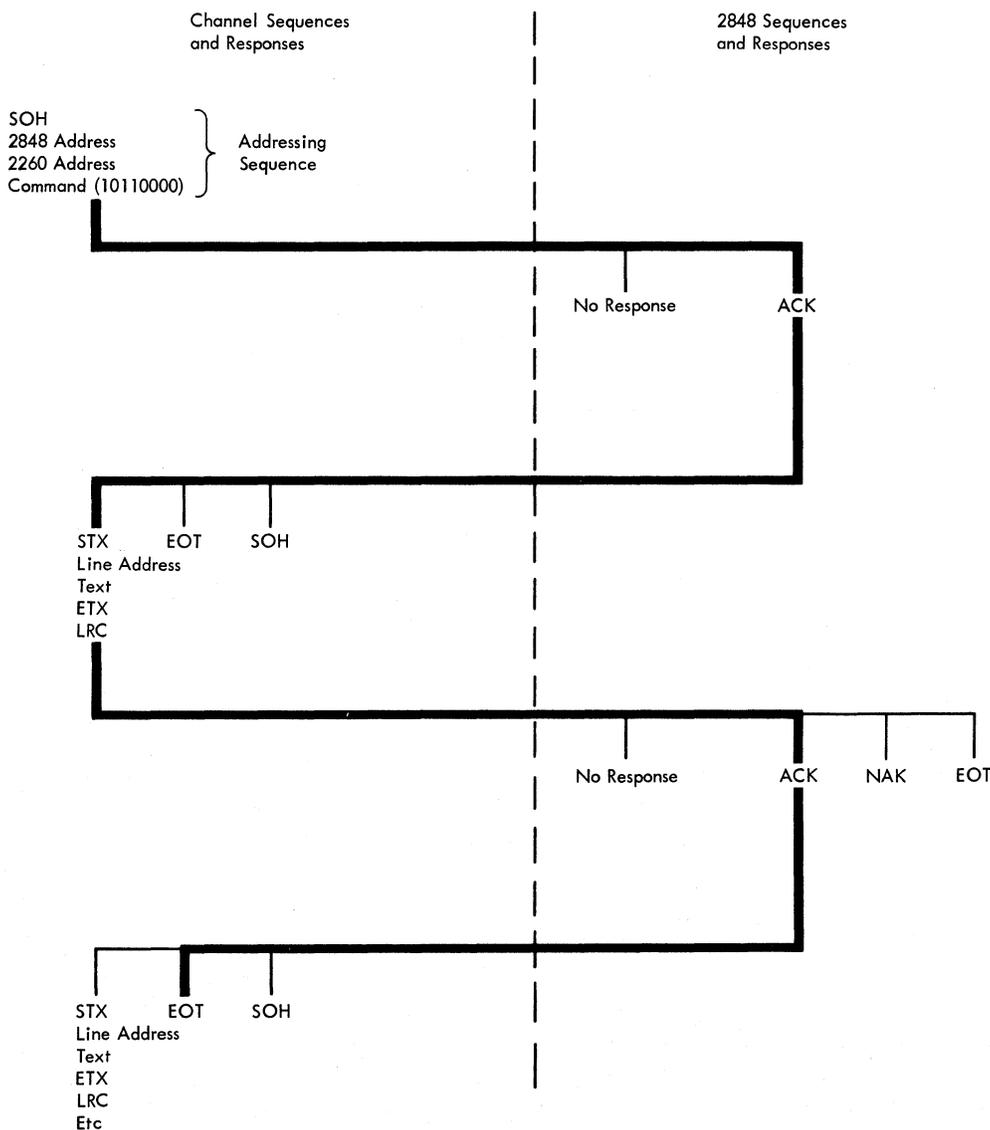
Figure 4-13. Sequence/Response Diagram - Line Address Write
