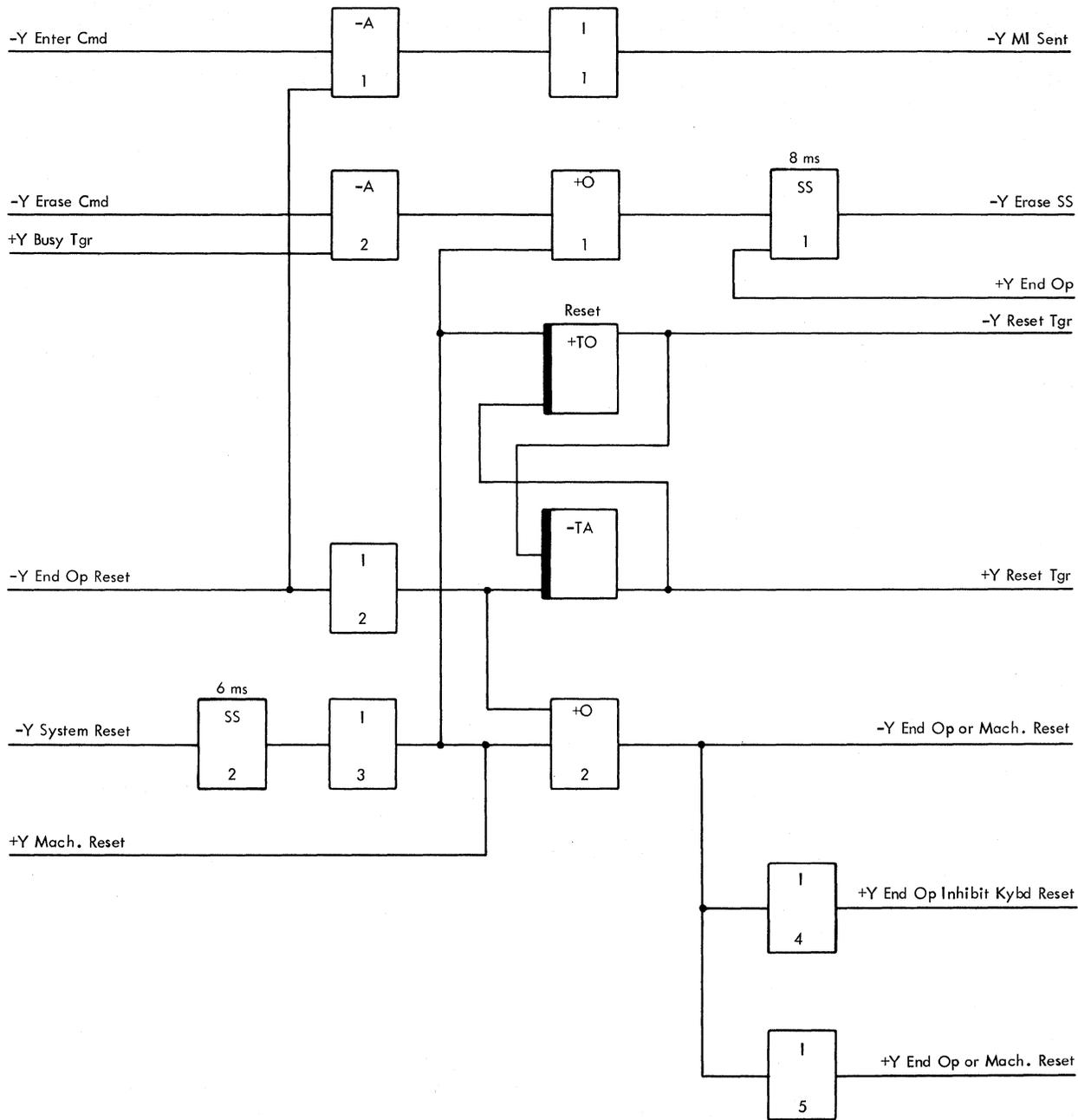
Figure 2-45. Reset Controls
