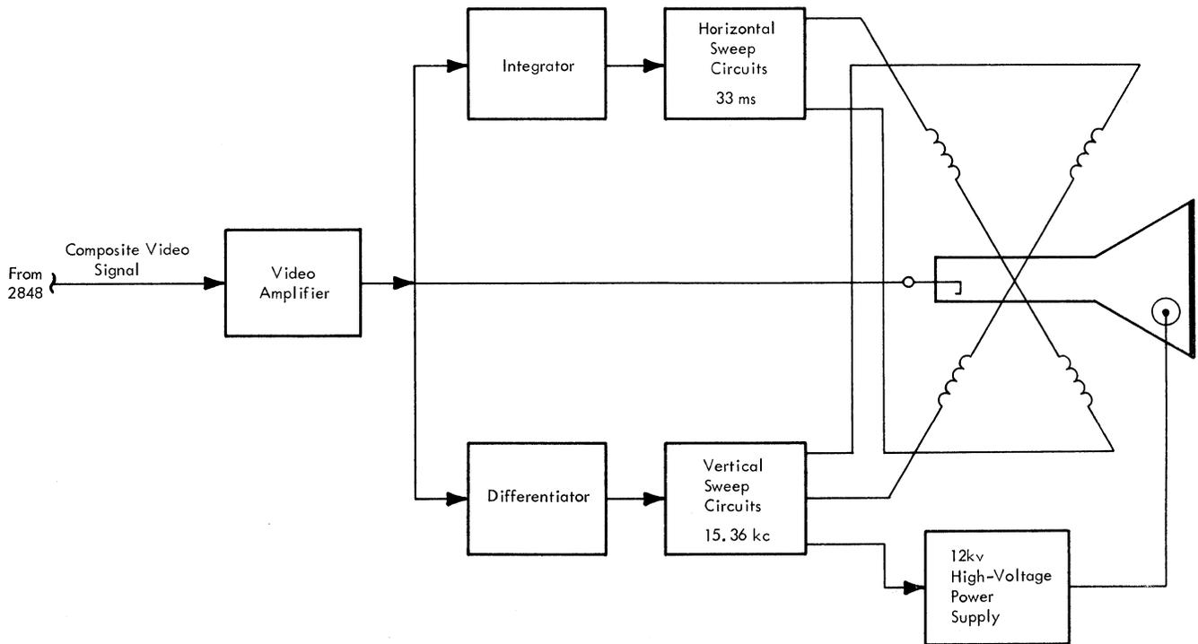
Figure 1-9. 2260 Display Station, Block Diagram
