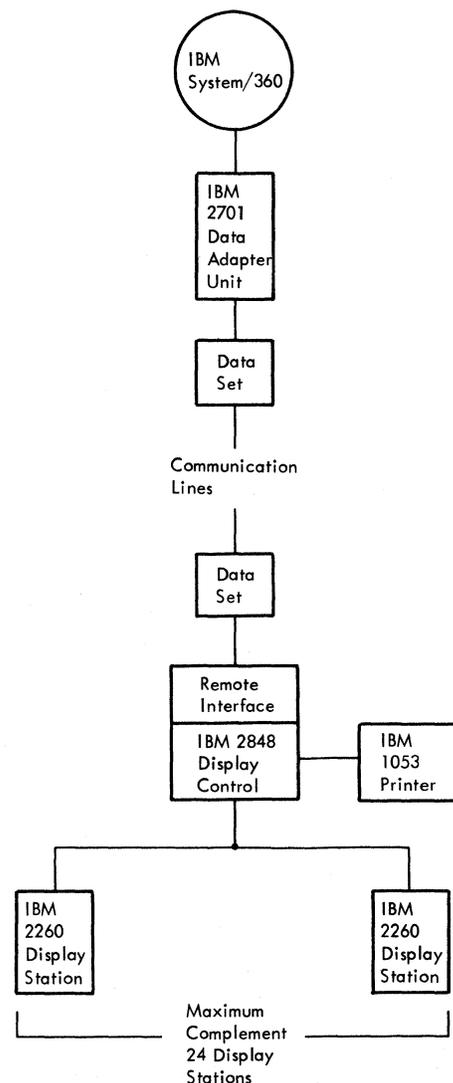
Figure 4-1. Remote Display Complex Configuration
