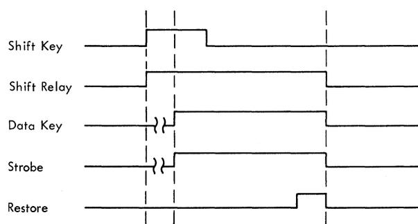
Figure 2-21. Keyboard Data Transfer Timing
