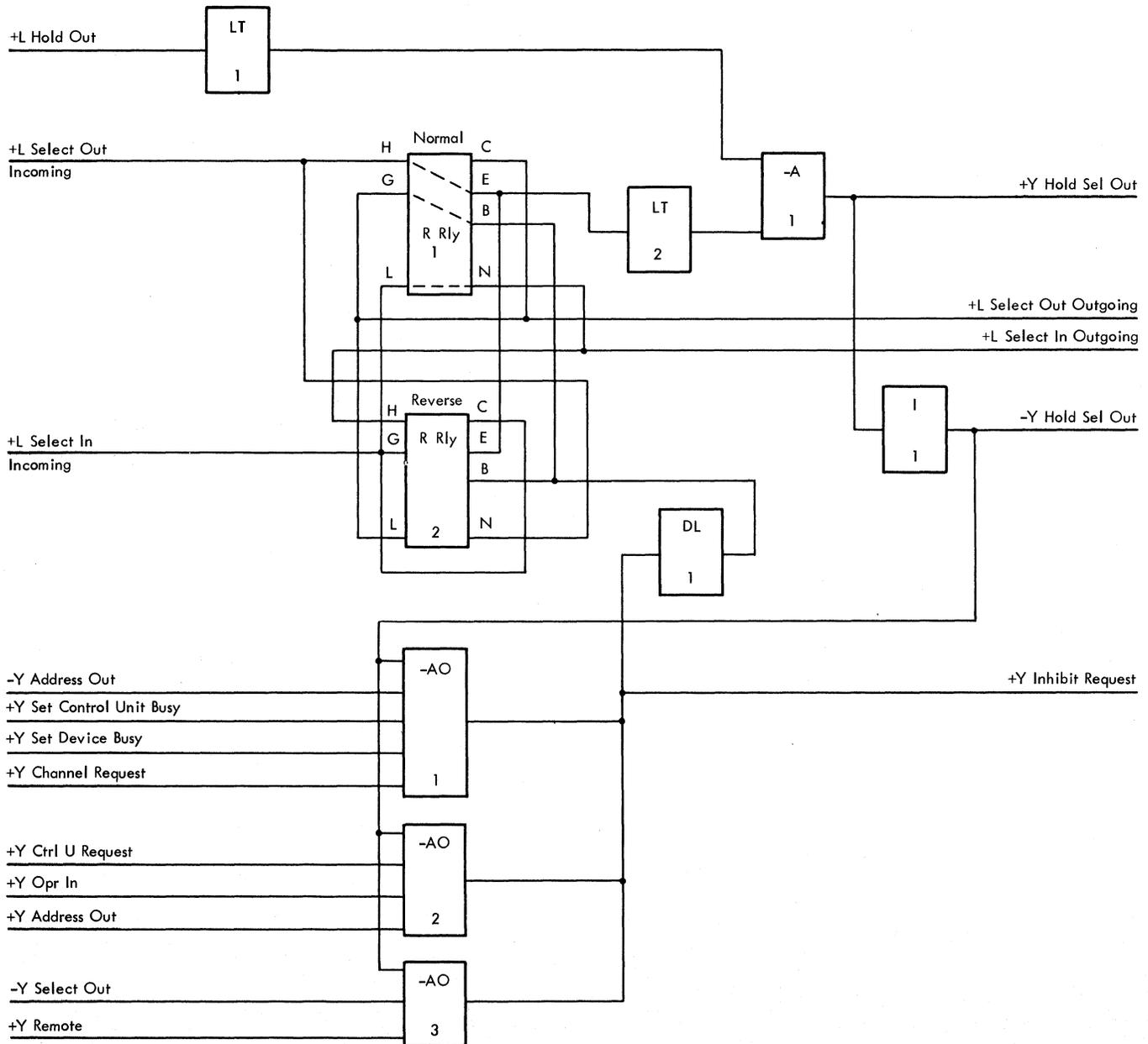
Figure 2-96. Hold-Select Circuit for Units Not Equipped with Isolation Feature
