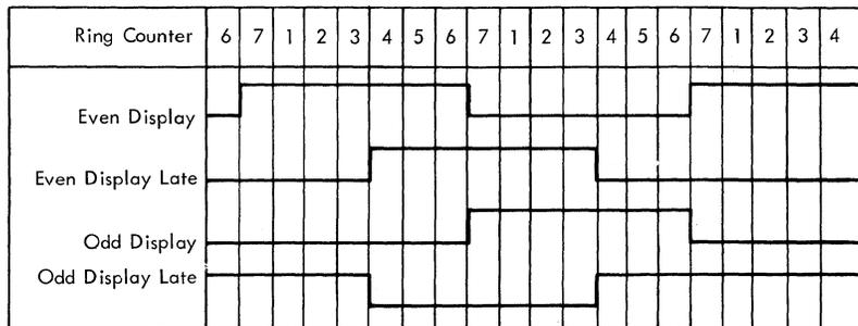
Figure 2-36. Even-Odd Display Trigger Circuit
