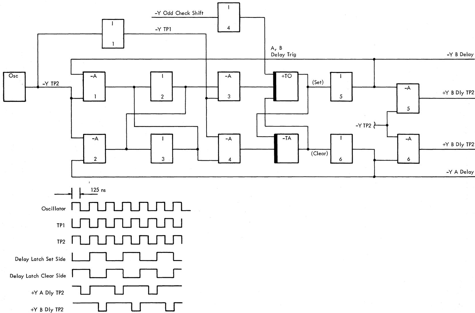
Figure 2-34. Oscillator and A-B Delay Pulse Circuit
