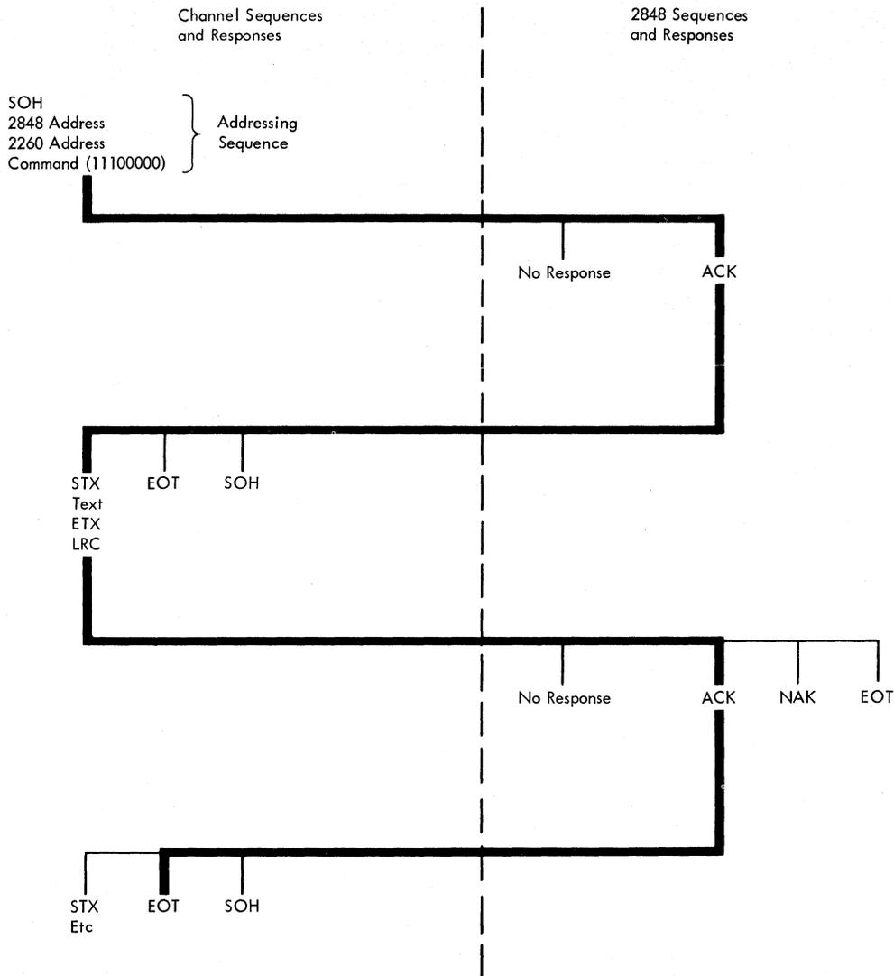
Figure 4-11. Sequence/Response Diagram - Erase/Write
