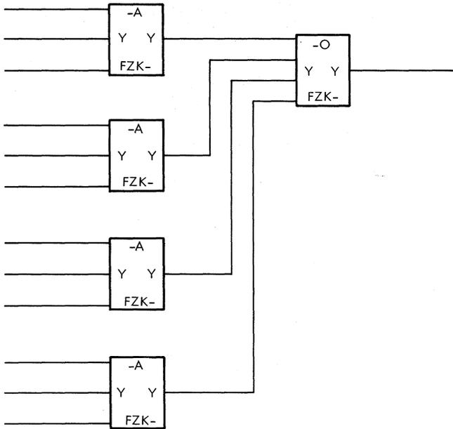
Figure B-2. Four Diode Coupled 3-Way AND Circuit, Type FZK
