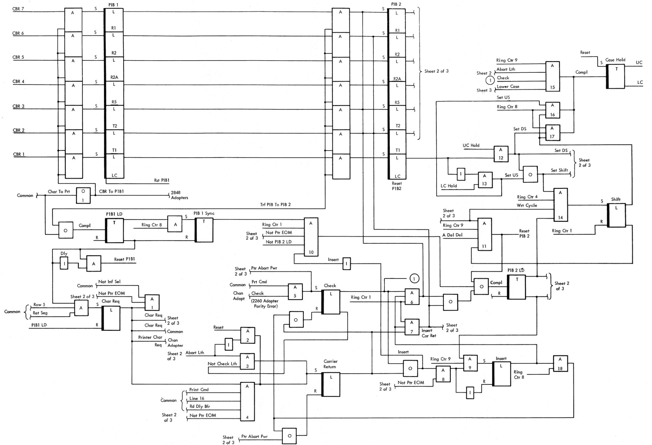
Figure 2-117. Printer Adapter, Logic Diagram (Sheet 1 of 3)
