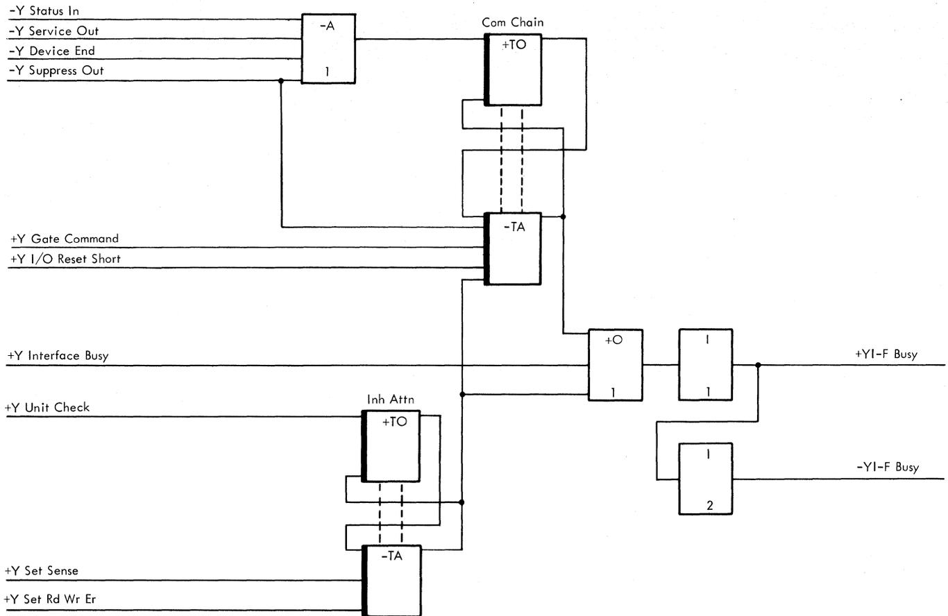
Figure 2-94. Command Chaining, Inhibit Attention
