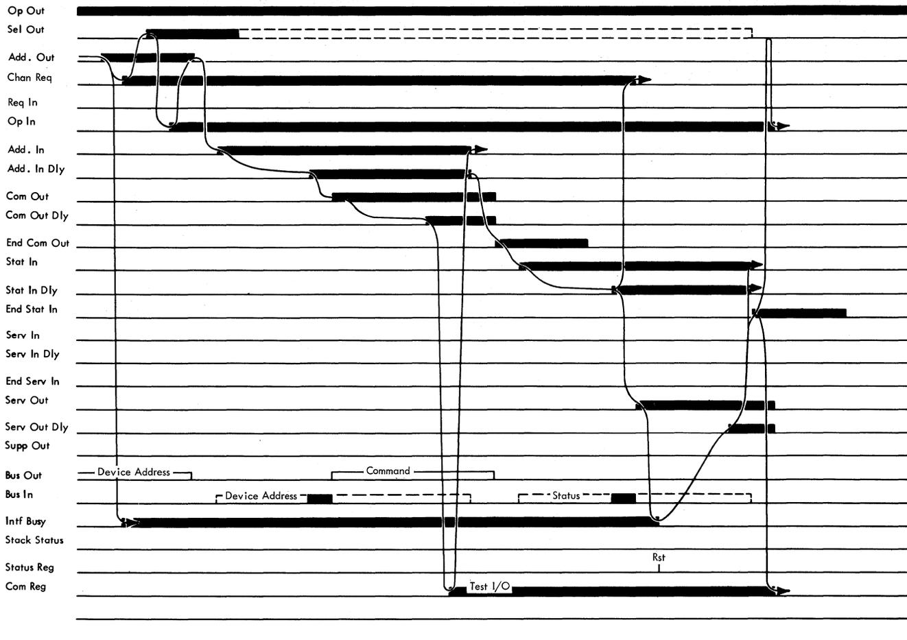
Figure 2-108. Test I/O Operation
