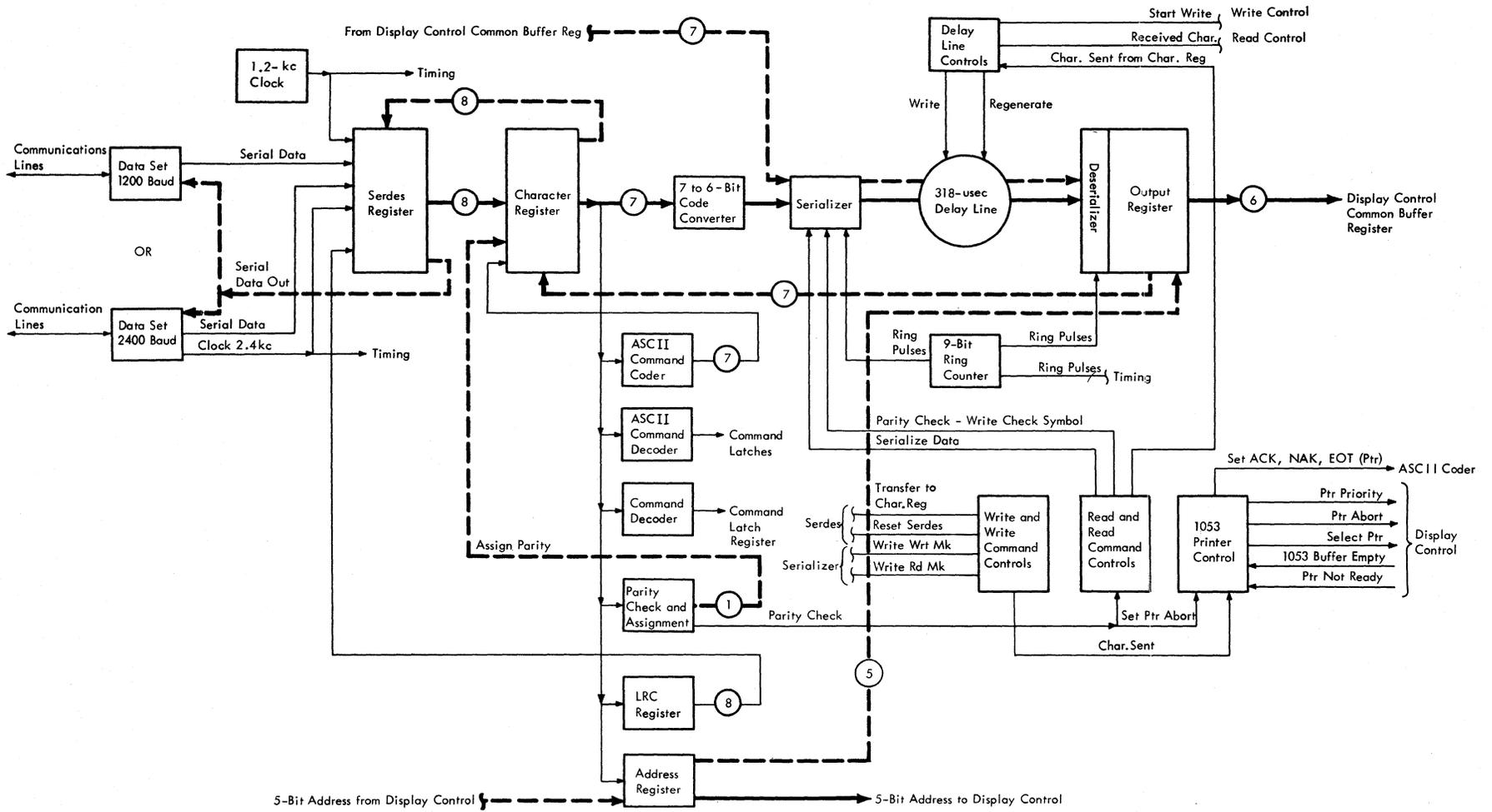
Figure 4-15. Remote Interface Adapter, Data Flow Diagram
