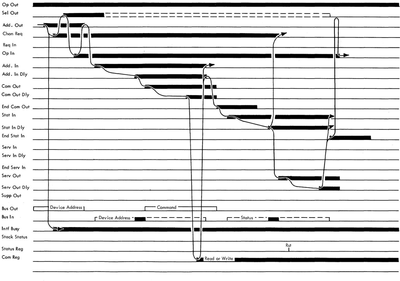
Figure 2-104. Channel-Initiated Selection (Read or Write)
