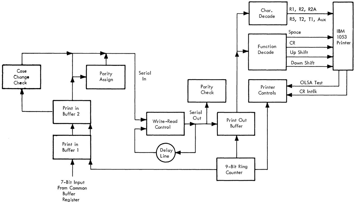
Figure 2-116. Printer Adapter, Simplified Block Diagram
