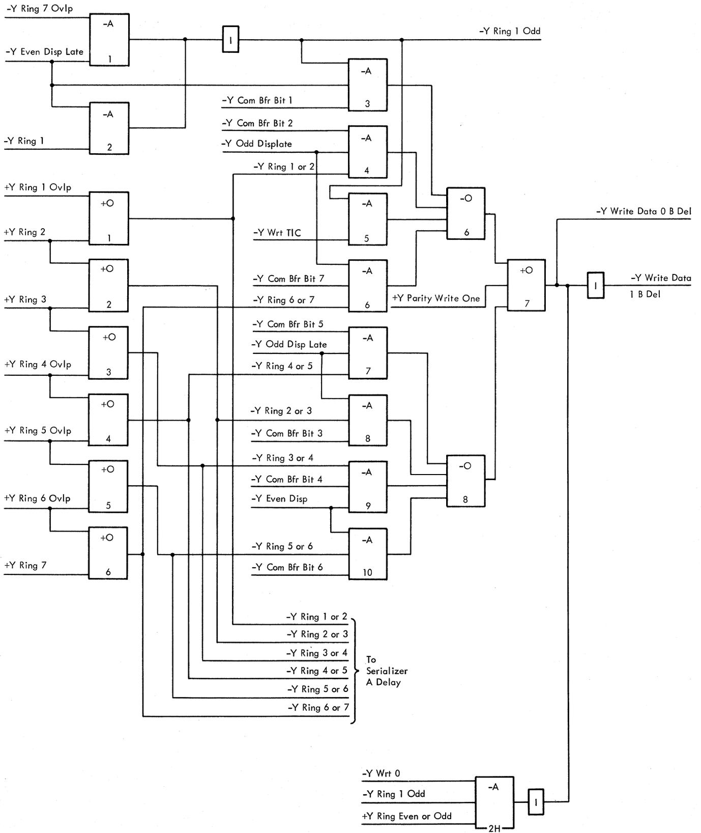
Figure 2-56. Serializer, B Delay
