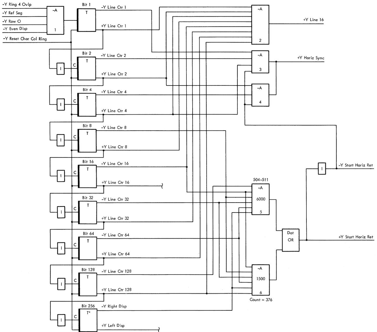
\* Trigger not used in Model 1 and Model 2 machines.
