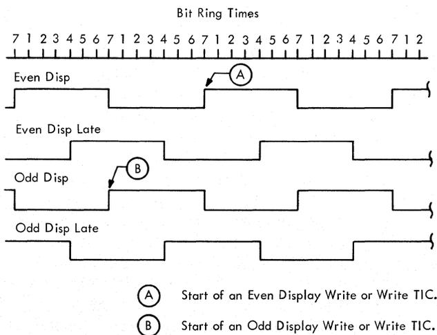
Figure 2-54. Even and Odd Display Signals, Timing Chart
