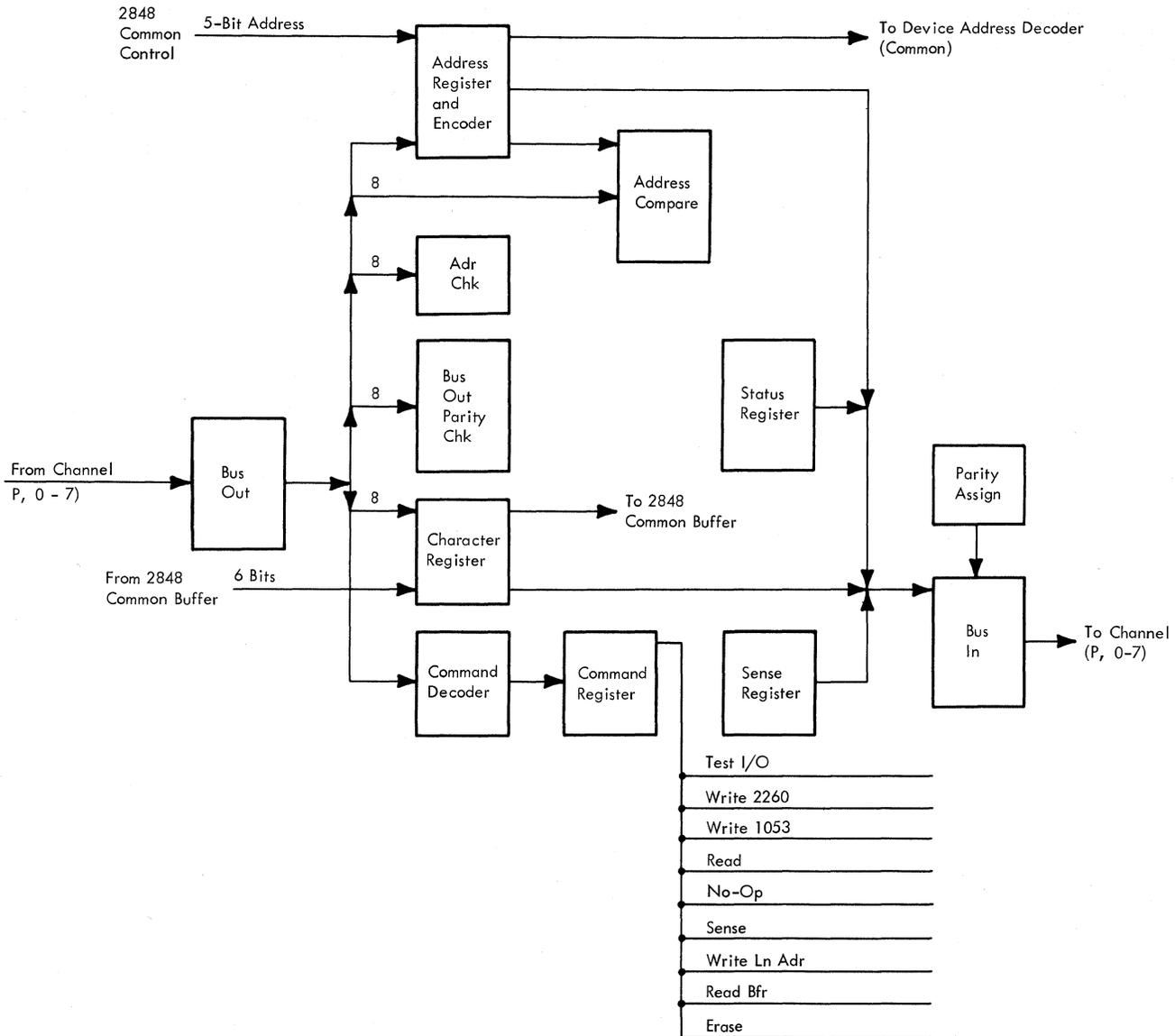
Figure 2-89. Channel Interface Controls
