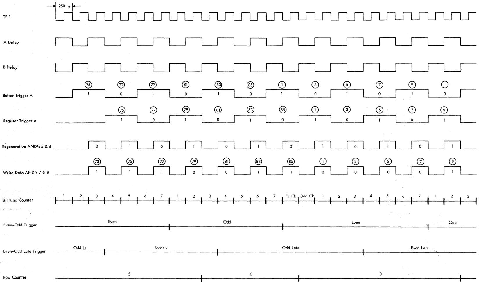
Figure 2-28. Delay Line Control Timing
