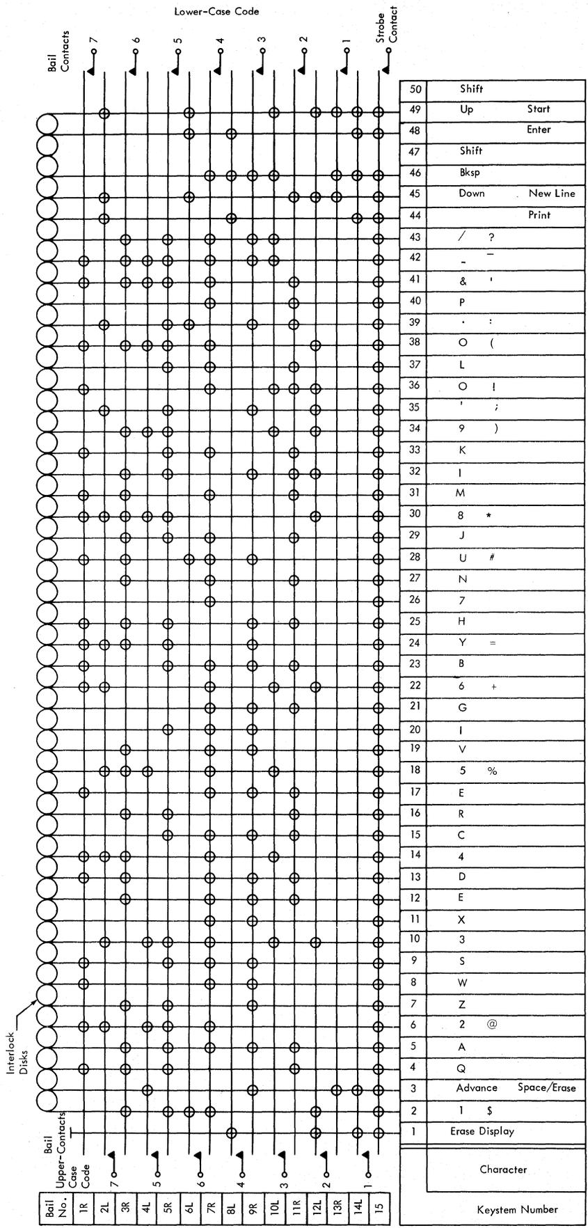
Figure 2-15. Keystem Number and Bail Selection For Alphanumeric Keyboard
