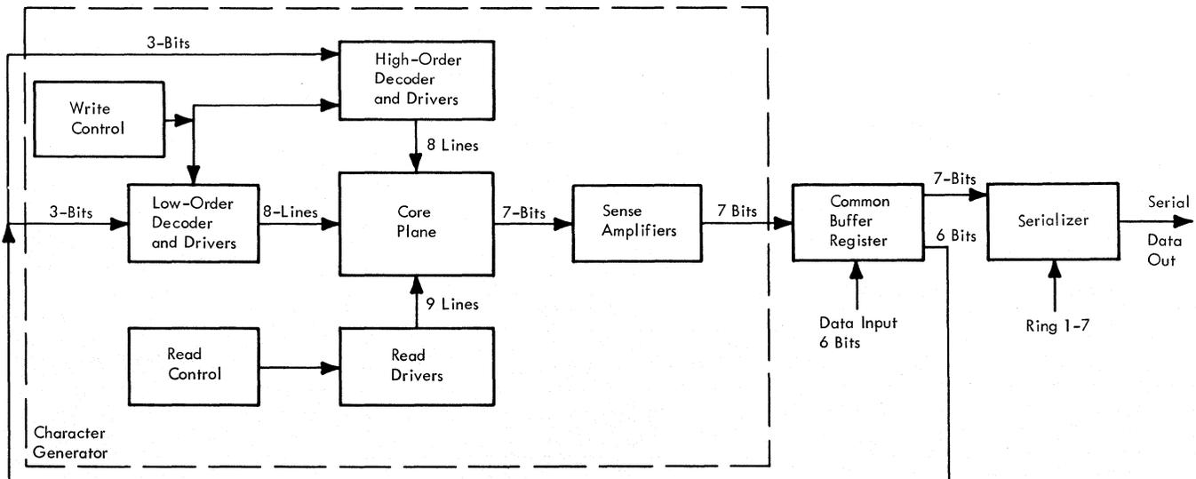
Figure 2-64. Character Generator, Block Diagram
