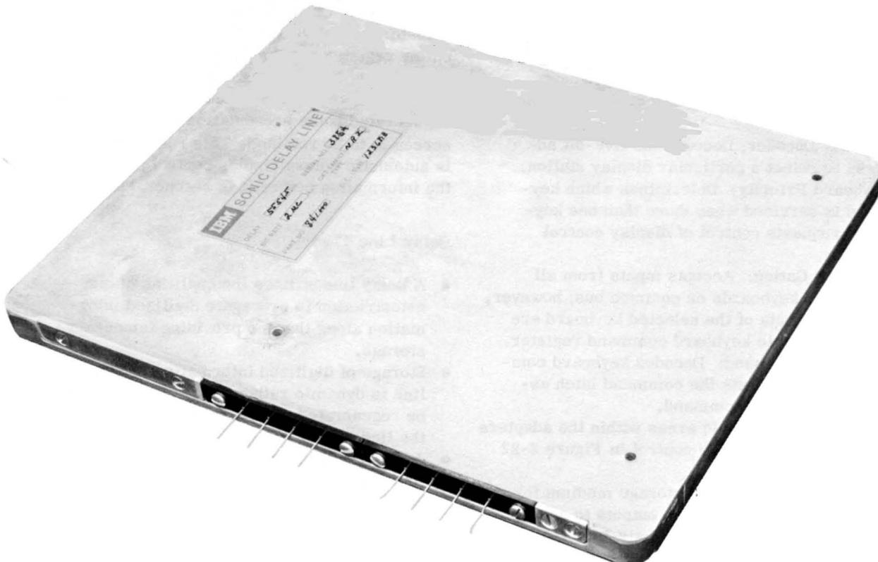
Figure 2-23. Delay Line Module
