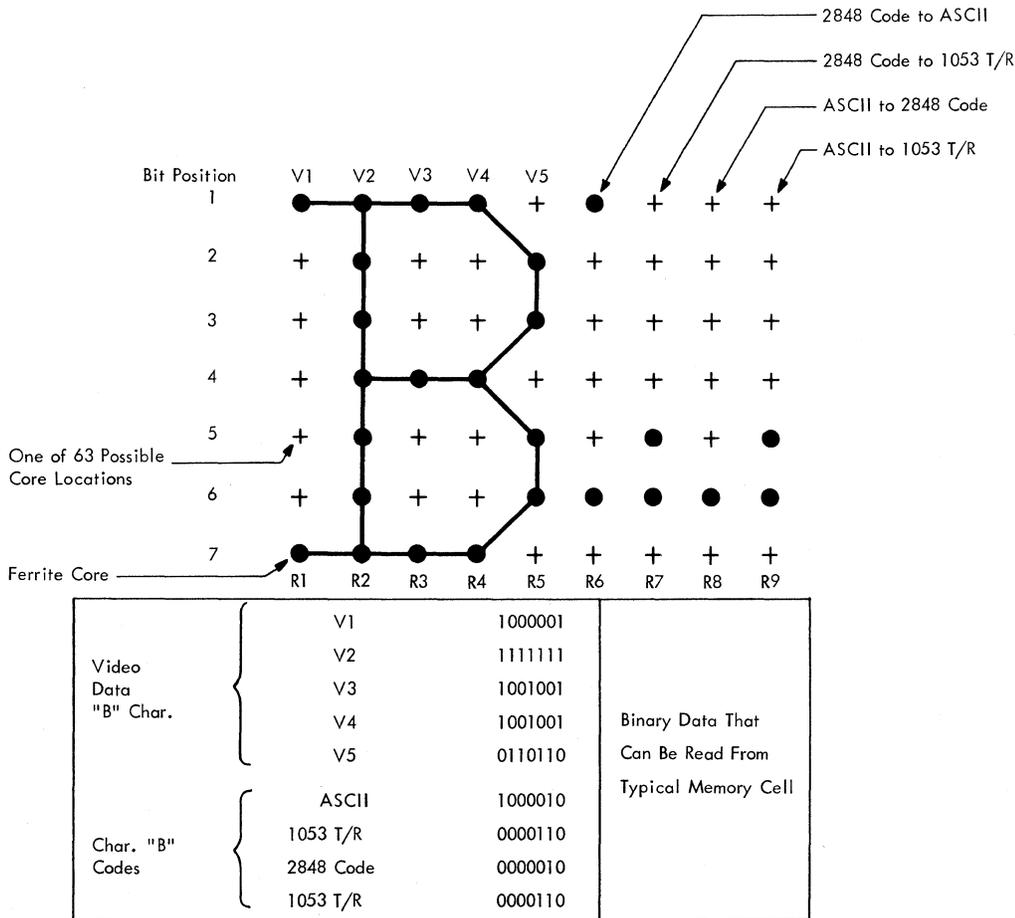
Figure 2-68. Generation of Binary Data from Memory Cell
