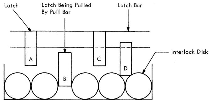
Figure 2-19. Interlock Disks (Partial)
