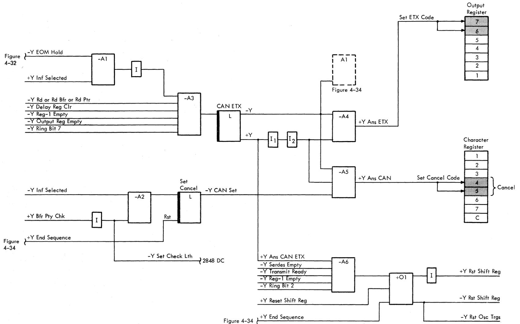
Figure 4-33. Read Operation - Buffer Parity Check Control
