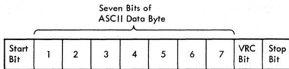
Figure 4-3. Ten-Bit Format of Transmitted ASCII Characters
