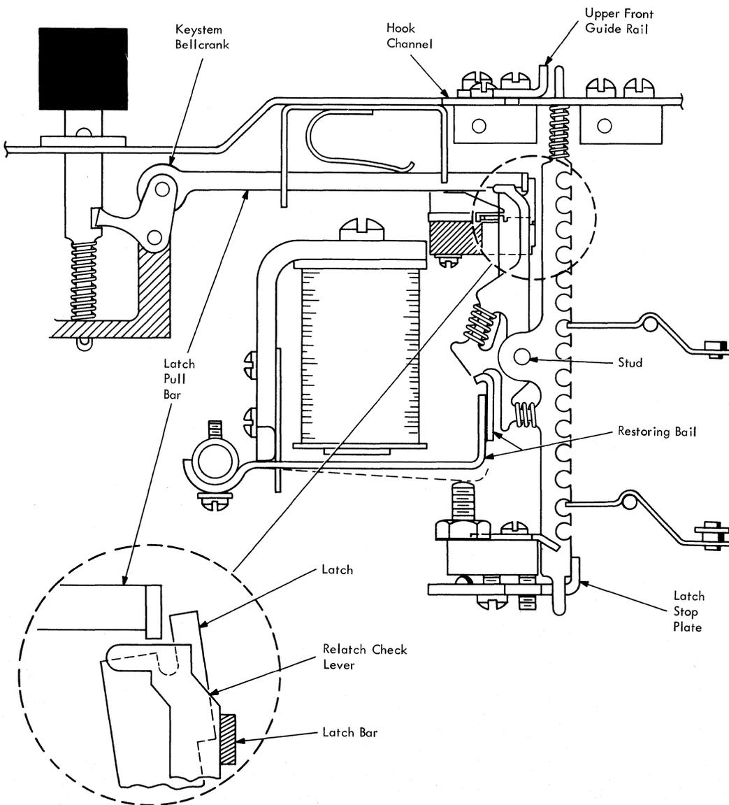
Figure 2-17. Key Position (Latched and Tripped)
