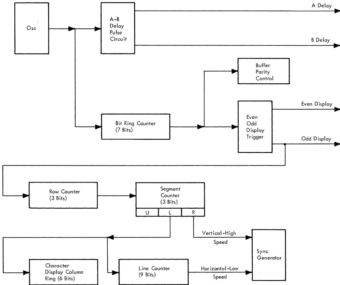
Figure 2-33. Timing and Clock Circuits, Simplified Block Diagram
