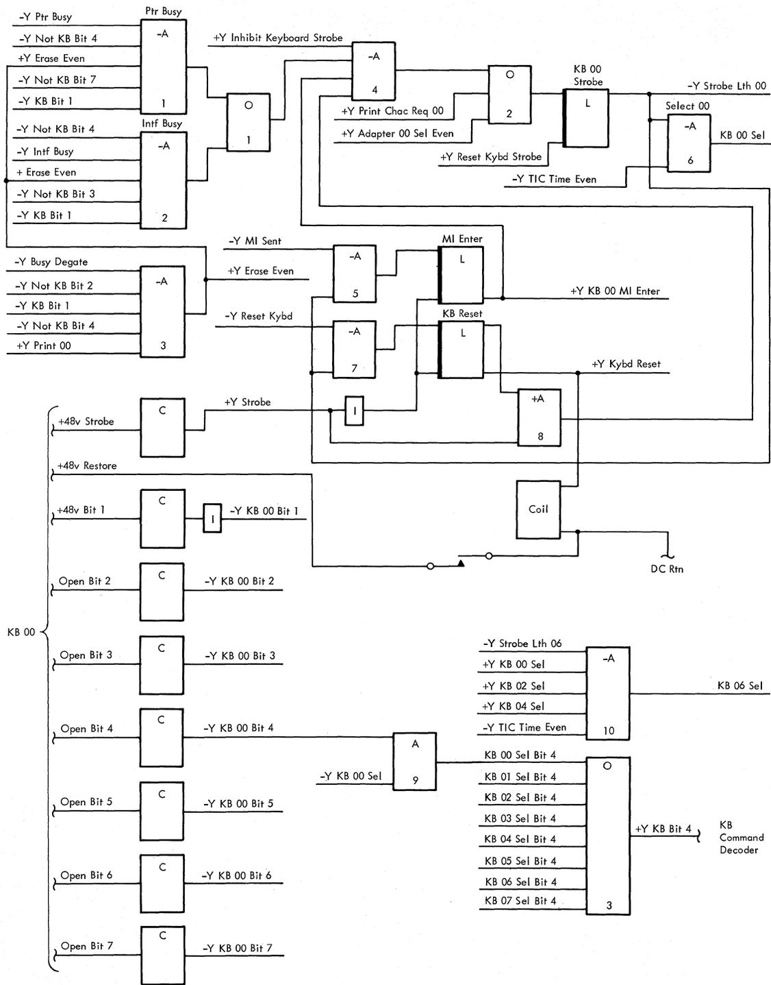
Figure 2-32. Keyboard Controls and Keyboard Data Bit Conversion and Gating
