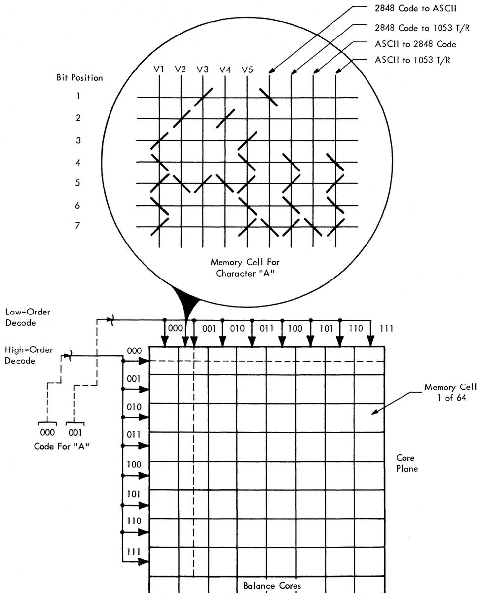
Figure 2-66. Core Plane Layout and Cell Selection
