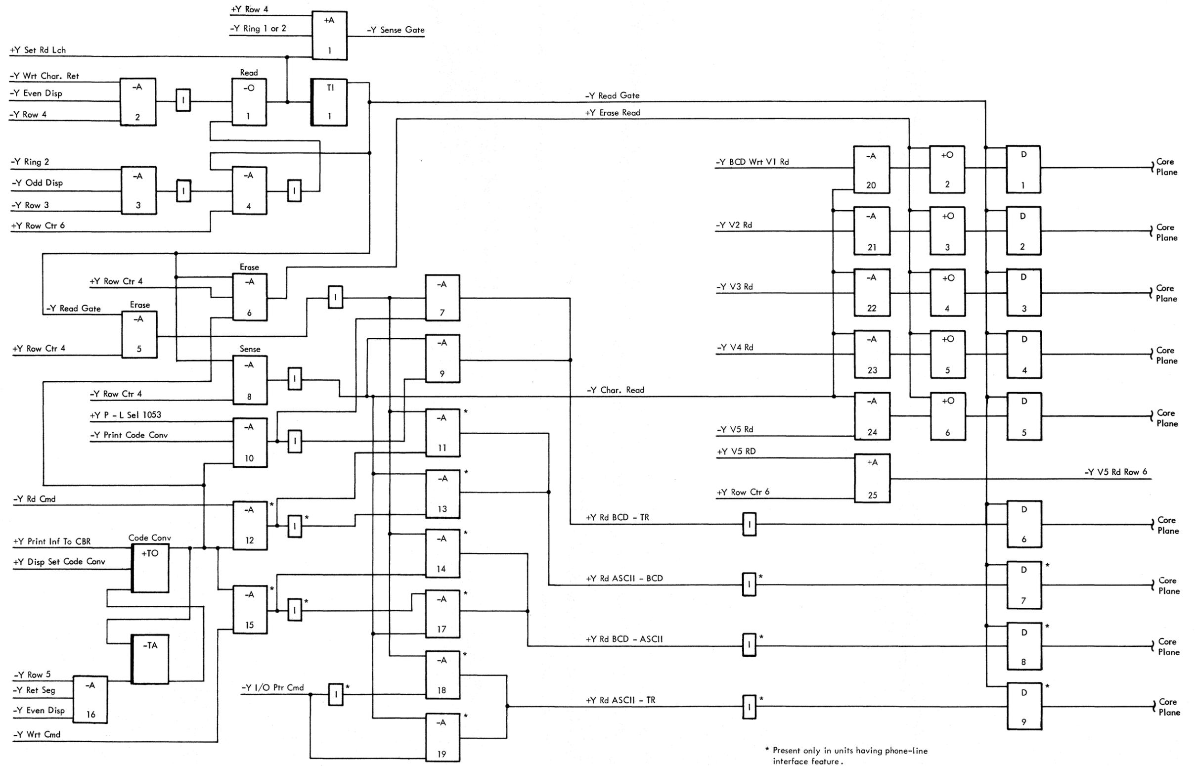
Figure 2-71. Character Generator Read Control Circuits
