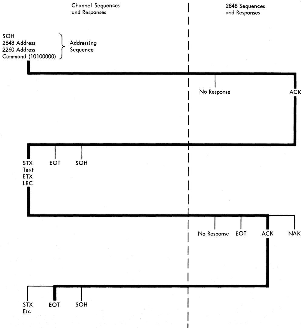
Figure 4-10. Sequence/Response Diagram - Write Addressed DS
