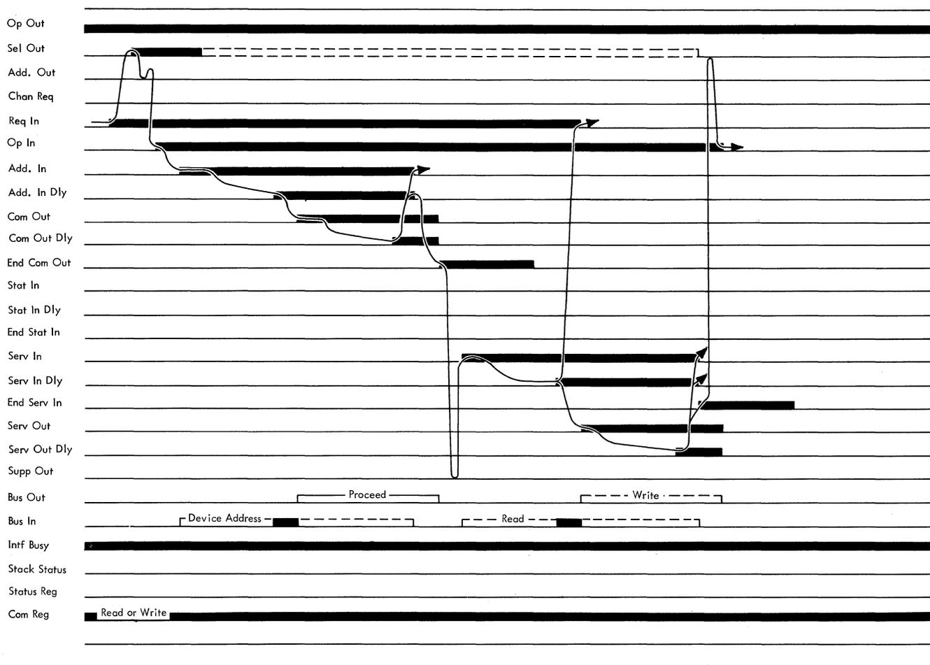
Figure 2-111. Control Unit Initiated Data Transfer (Read or Write)
