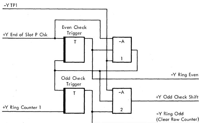
Figure 2-37. Buffer Parity Control Circuit
