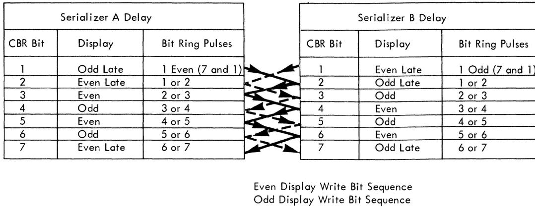
Figure 2-57. Serializer Data and Inputs and Even-Odd Bit Sequences
