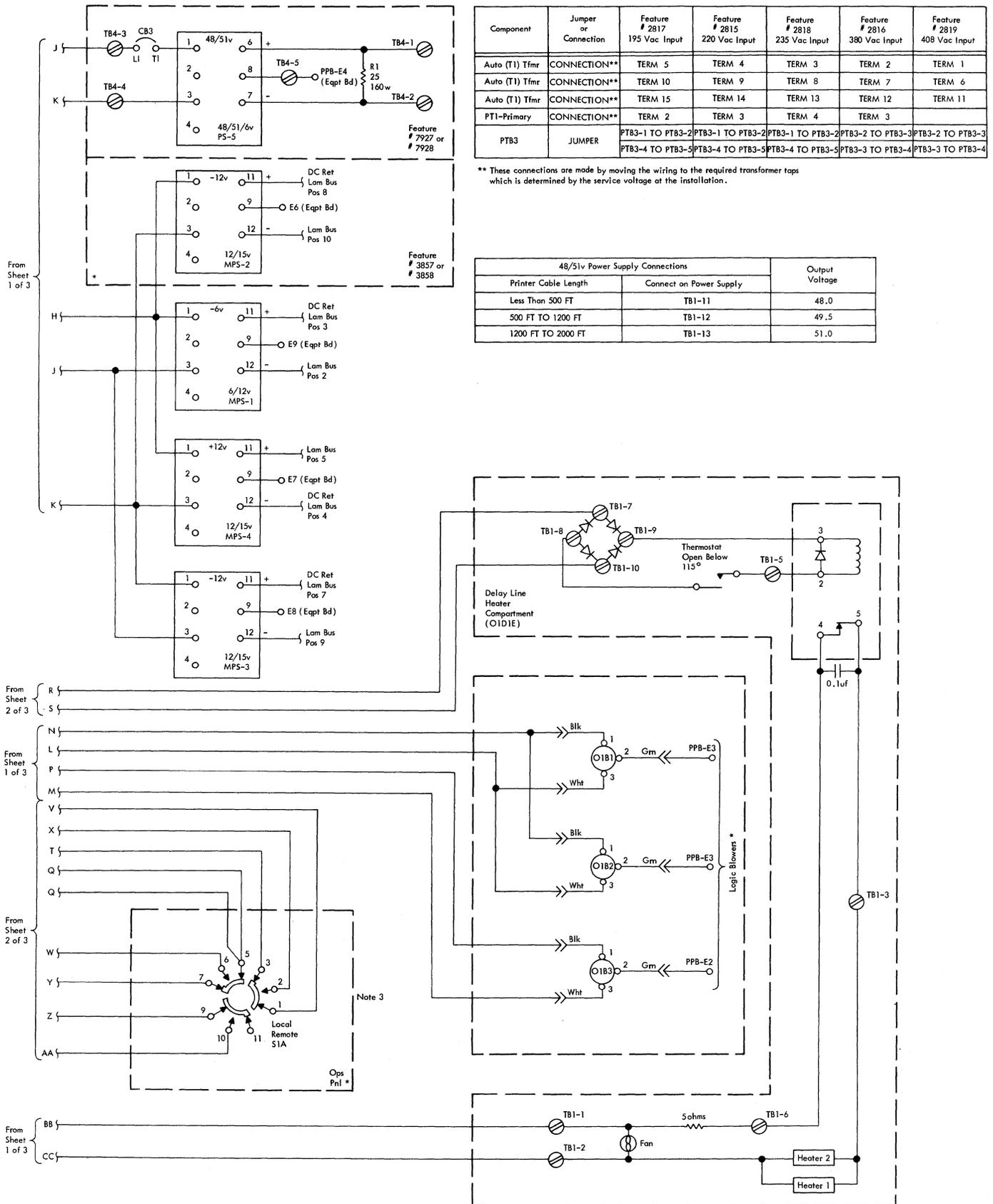
Figure 5-2. 50-Cycle Power Distribution and Control (Sheet 3 of 3)
