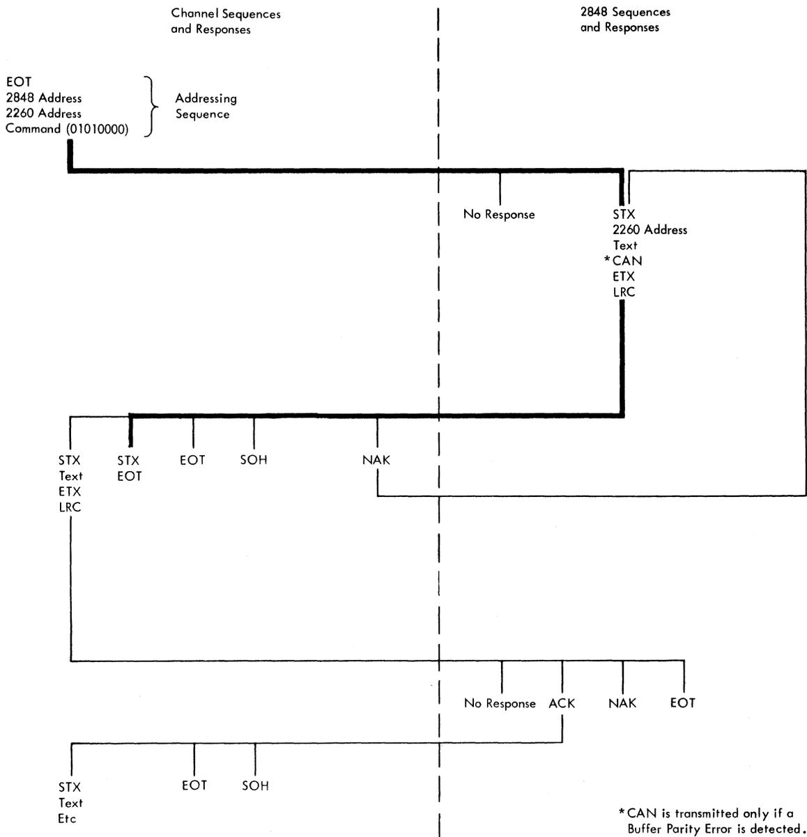
Figure 4-9. Sequence/Response Diagram - Read Addressed Full DS Buffer
