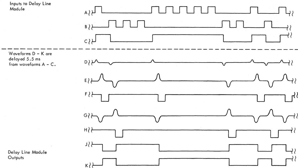
Figure 2-25. Delay Line Timing
