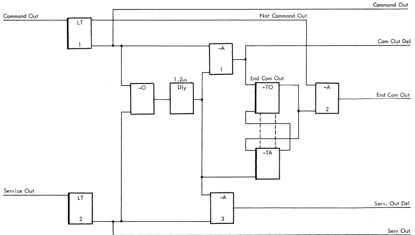
Figure 2-90. Out Tag Delays
