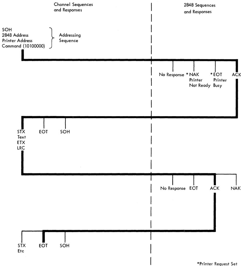
Figure 4-12. Sequence/Response Diagram - Write Printer
