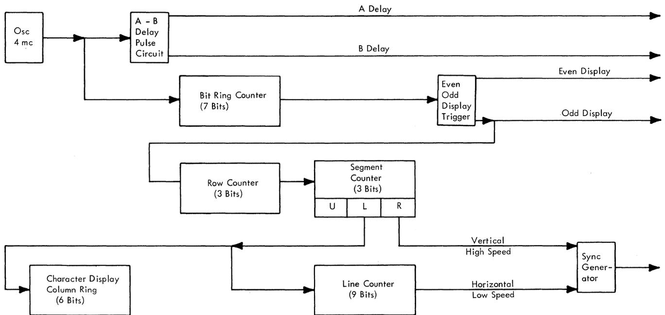
Figure 1-7. Timing and Clock Circuits, Simplified Block Diagram
