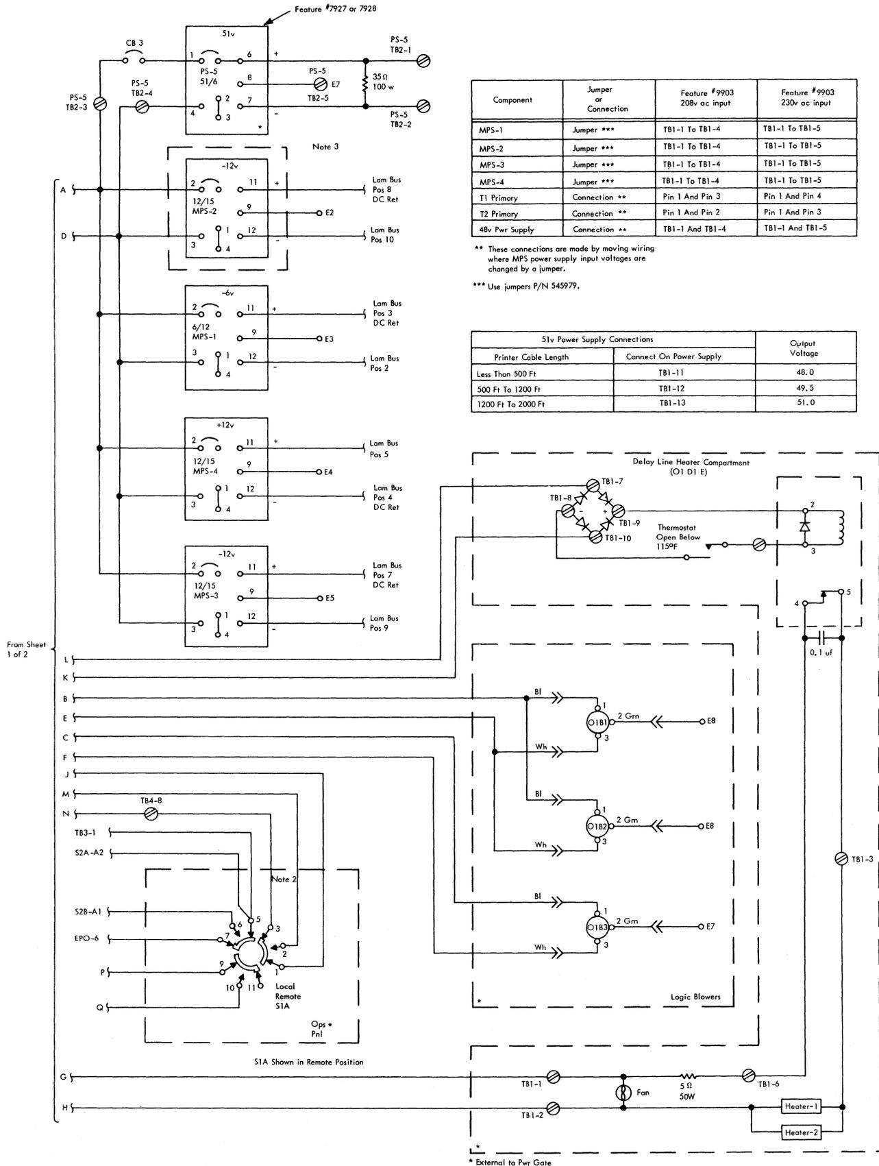
Figure 5-1. 60-Cycle Power Distribution and Control (Sheet 2 of 2)
