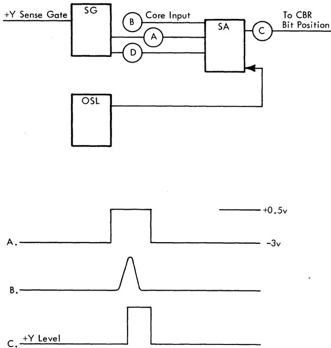
Figure B-4. Output Sense Level, and Sense Gate, Type FYZ
