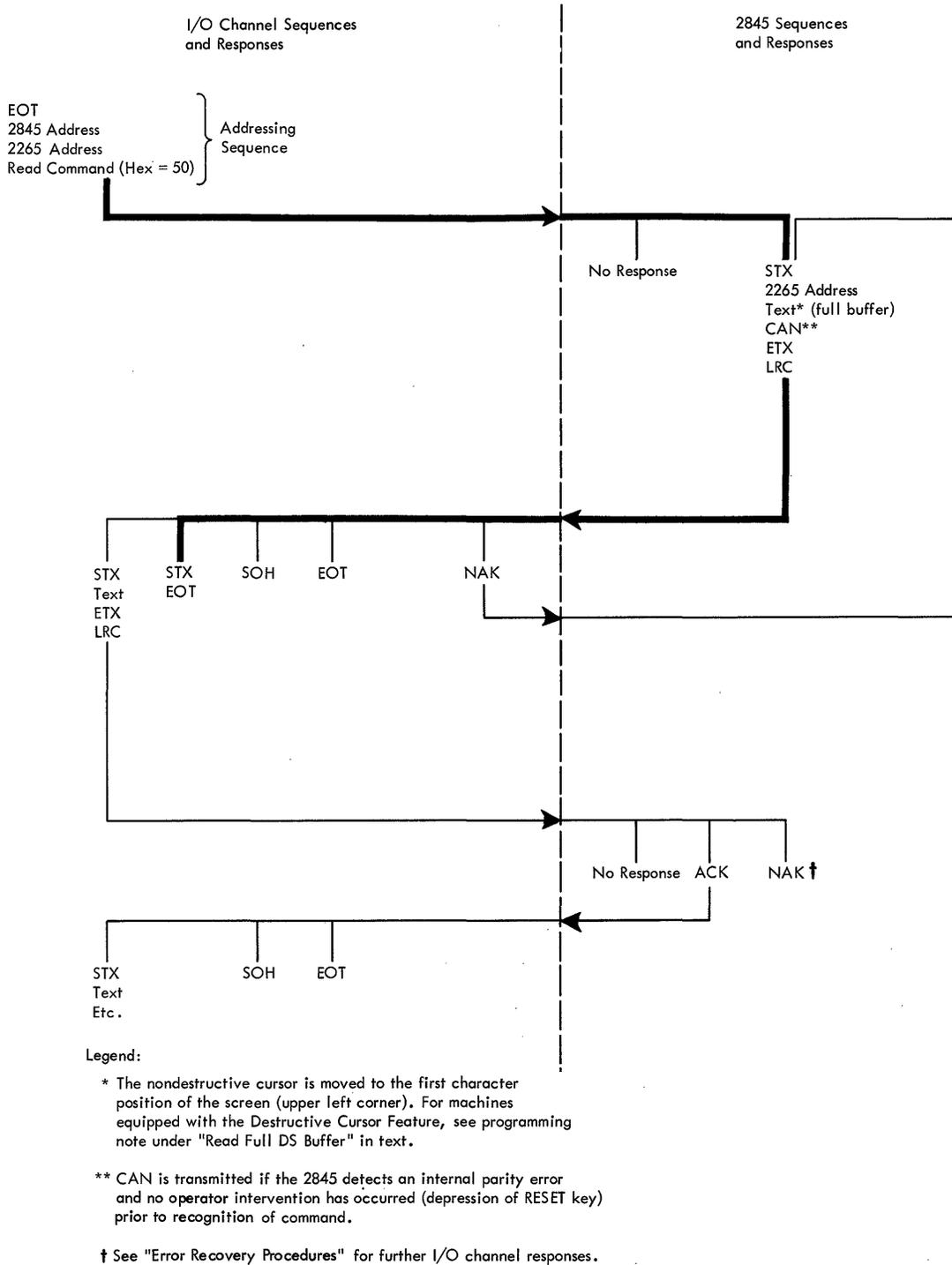
Figure 9. Read Addressed Full DS Buffer, Sequence/Response Diagram
