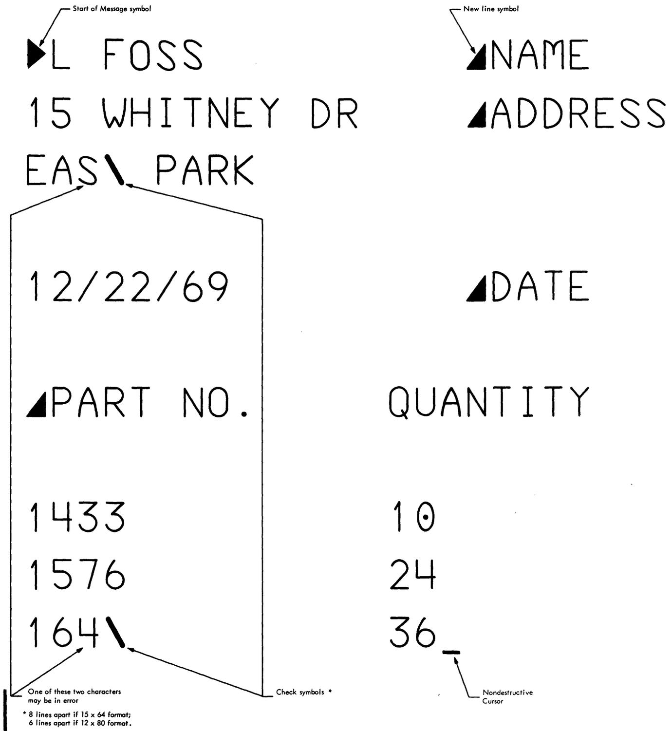
●Figure 3. Example Display Showing SOM, NL, Check Symbols, and Nondestructive Cursor (15 x 64 Display Format)
