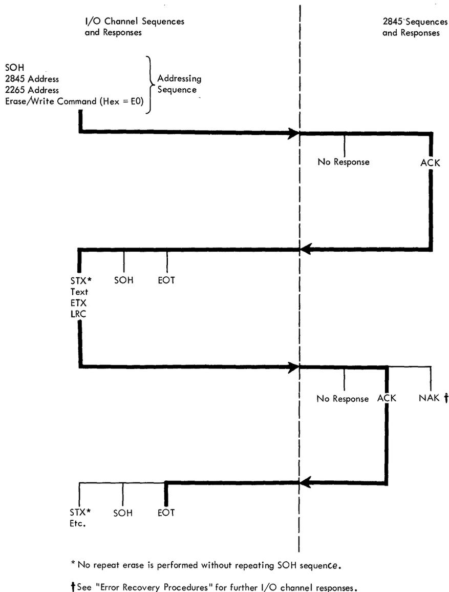
Figure 11. Erase/Write Addressed DS, Sequence/Response Diagram
