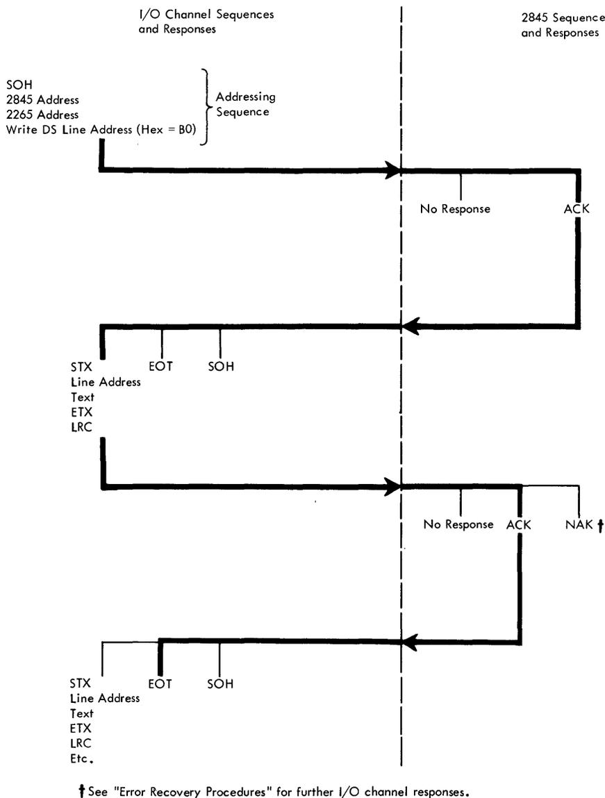
Figure 13. Write DS Line Address, Sequence/Response Diagram
