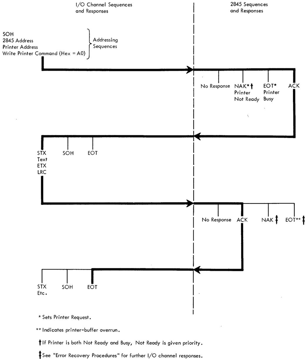
Figure 12. Write Printer, Sequence/Response Diagram
