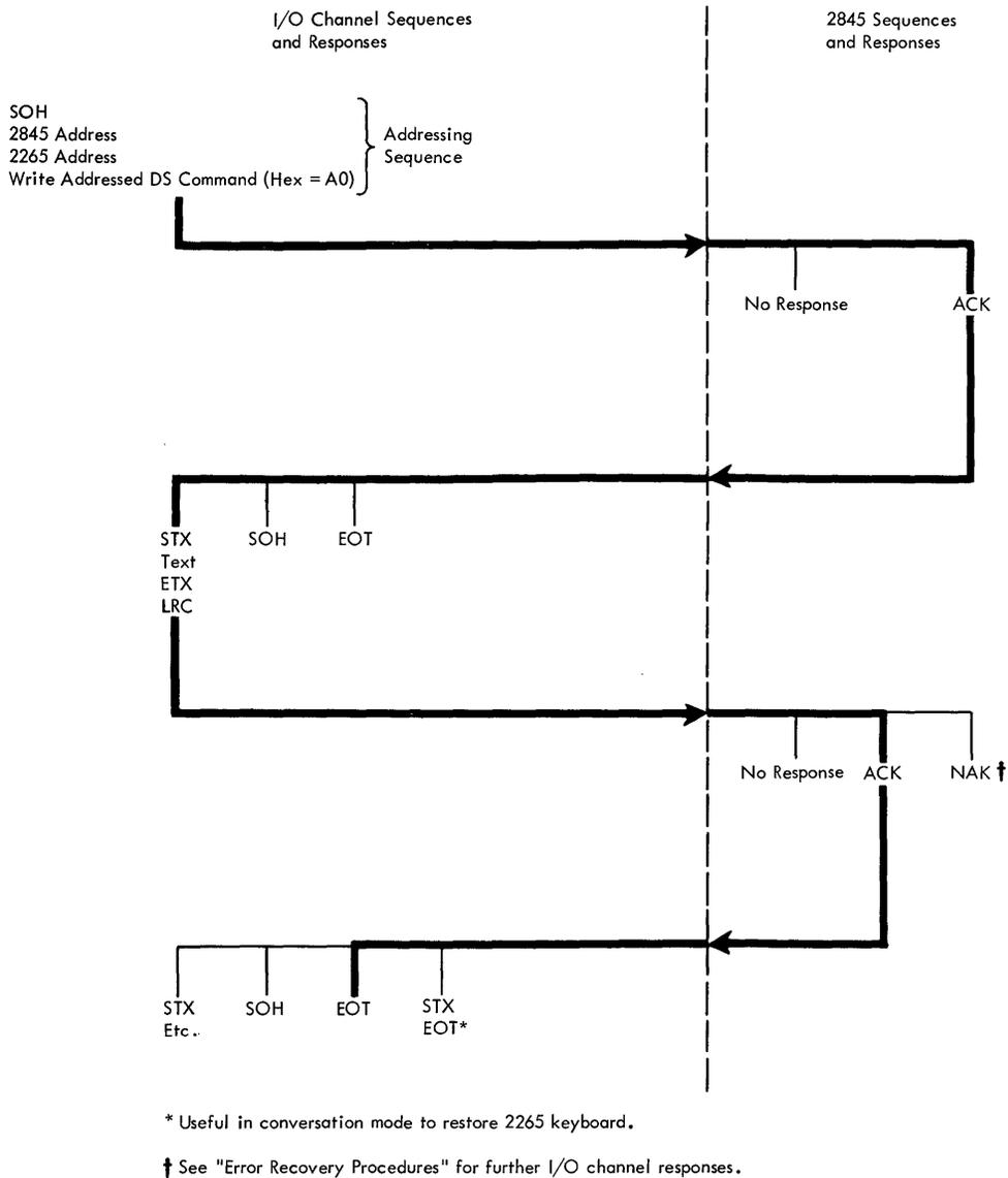
Figure 10. Write Addressed DS, Sequence/Response Diagram
