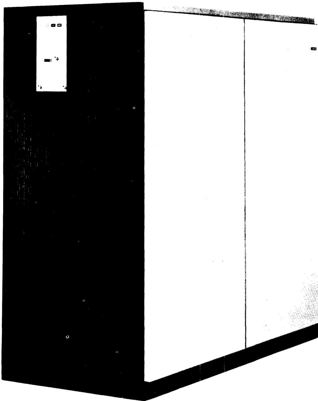
Figure 1. IBM 2703 Transmission Control
