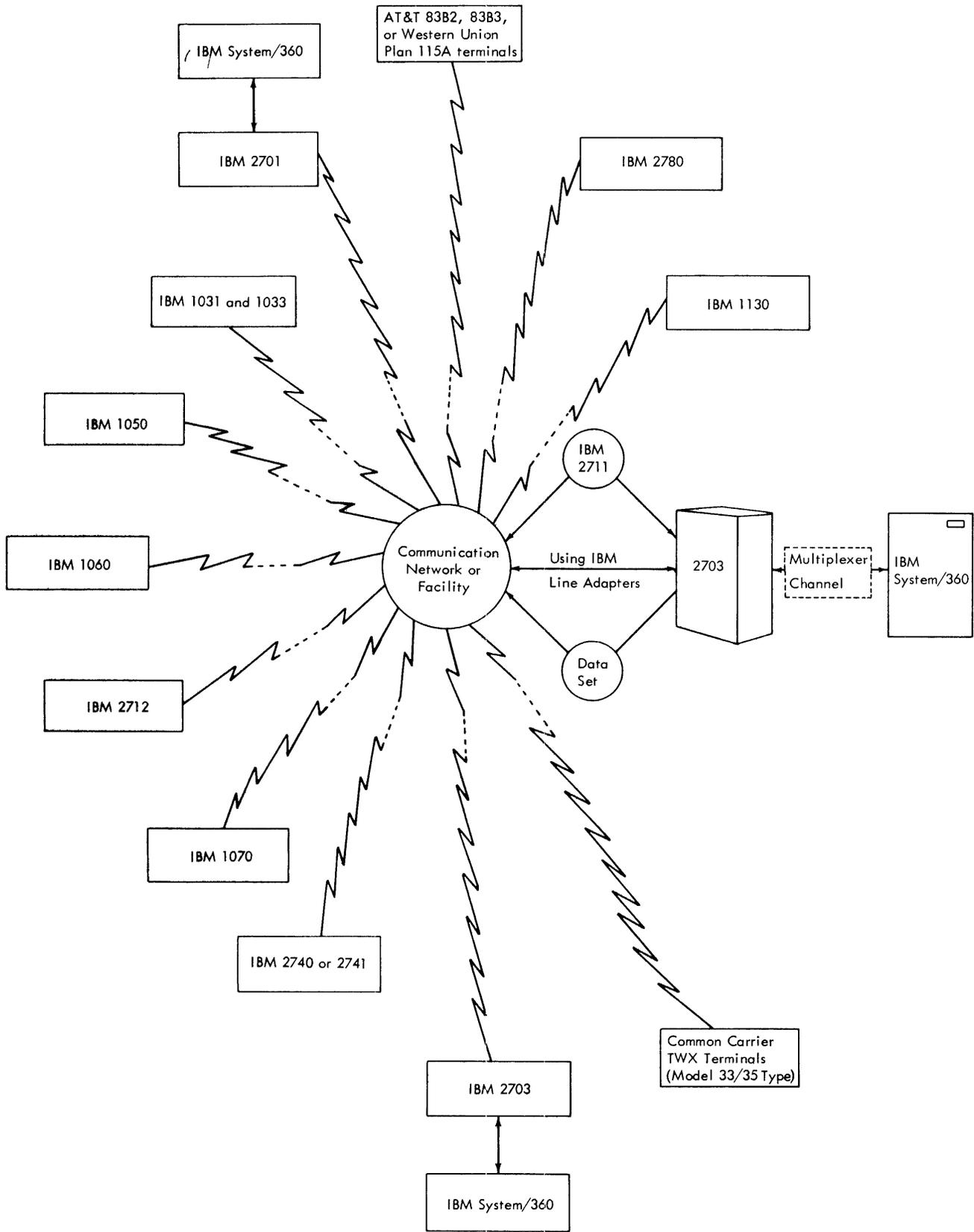
Figure 2. Data Communication Units Attachable to the 2703
