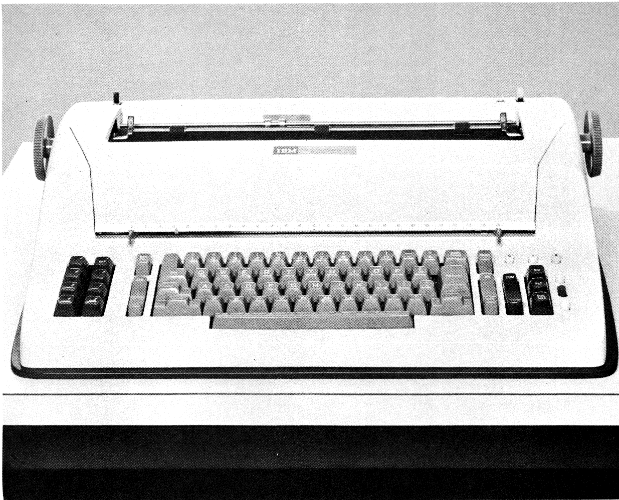
Figure 2. 2740 Model 1 Keyboard (PTTC/BCD)
