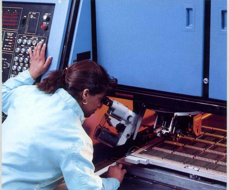
An assembler at the control panel of the machine that puts twisted pair wires on the TCM circuit board.
