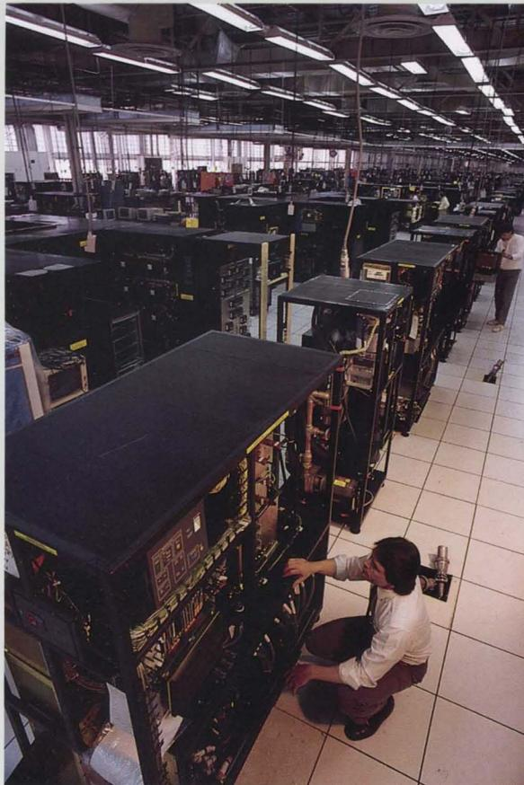
**IBM 3090 systems line up for final test prior to shipment at the half-mile-long testing facility in Kingston, New York.**
