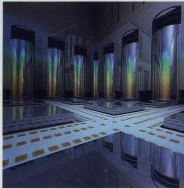
Extensive upgrade options are made possible in part by the extendibility of the 3090 advanced packaging technology as shown by this three-dimensional computer-generated closeup of a cutaway Thermal Conduction Module.
