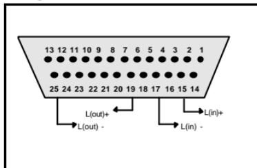
RS-422 Host/Printer Port 1 Pin Assignments
