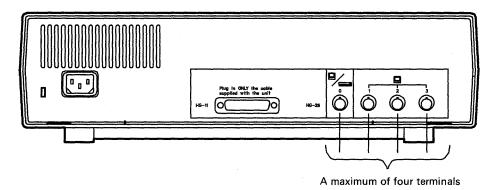
Figure 4-16. Models 81R, 82R, 91R, and 92R with Terminals Attached Directly to the Terminal Adapter
