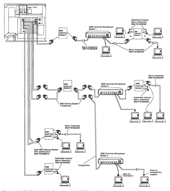
Figure 4-21. 3174 Terminal Cable Connections Using IBM Cabling System Media
