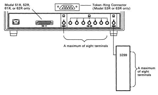
Figure 4-13. Models 51R, 52R, 53R, 61R, 62R, and 63R with One 3299 Terminal Multiplexer
