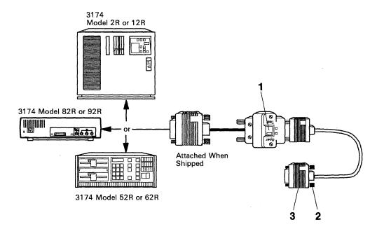
Figure 4-23. An X.21 Cable Connection
