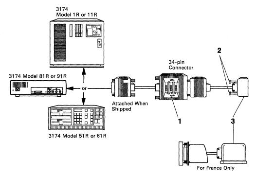
Figure 4-24. A CCITT V.35 Cable Connection
