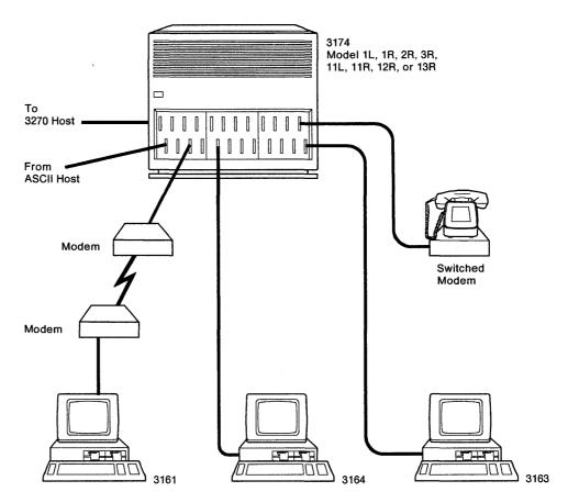
Figure 1-3. An Example of a 3174 Subsystem with the AEA Feature
