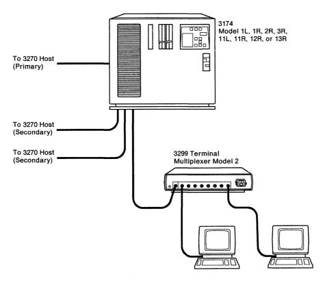
Figure 1-4. An Example of a 3174 Subsystem with the CCA Feature
