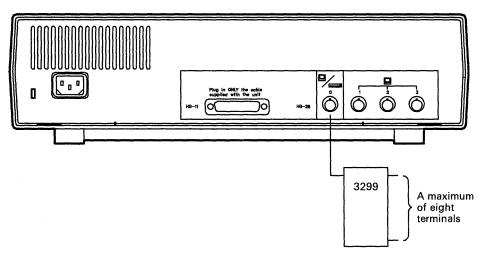
Figure 4-17. Models 81R, 82R, 91R, and 92R With One 3299 Terminal Multiplexer
