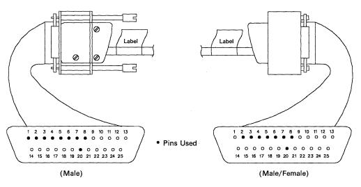
Figure 3-7. EIA 232D External Interface Cabling to a DTE
