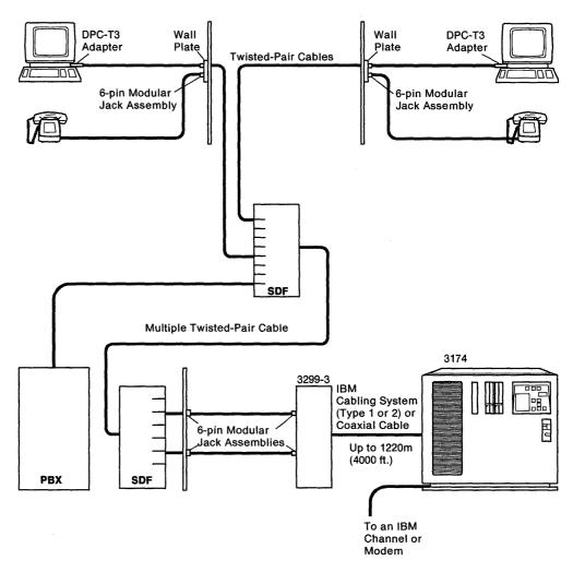
Figure 3-4. A 3270 Installation Using DPC-T3 Adapters and a 3299 Terminal Multiplexer Model 3
