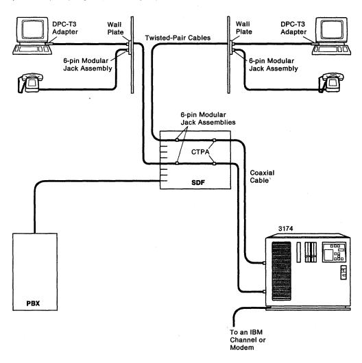
Figure 3-3. A 3270 Installation Using DPC-T3 Adapters with Coaxial and Twisted-Pair Cable (U.S. and Canada only)
