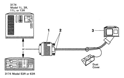
Figure 4-25. A Token-Ring Network Adapter Cable Connection
