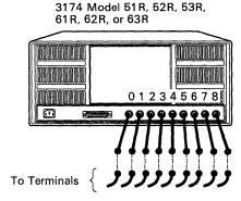
Complete the connection for each DIRECT-ATTACHED terminal to be installed.
