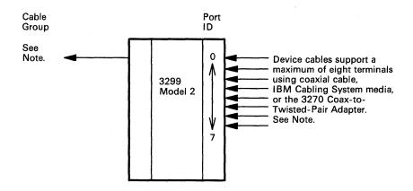
Note: Device cables are supplied, installed, and maintained by the customer. For additional information about device cables, see Chapter 3, "Planning Subsystem Cabling," and the following manuals:
