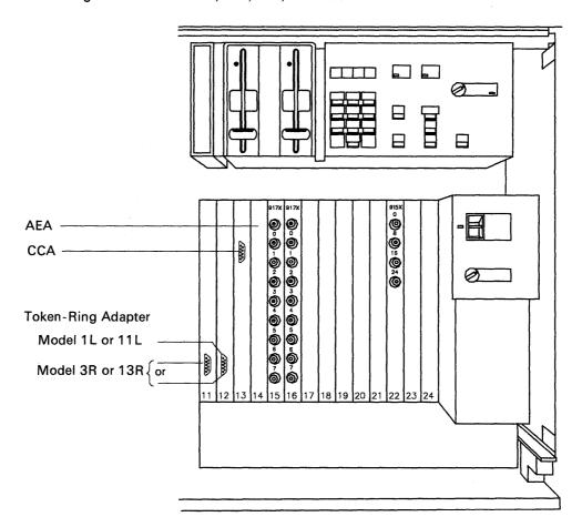
Figure 4-8. 3174 Logic Board with Labeled Slots. The terminal adapter is in slot 22, and there are two TMAs, in slots 15 and 16.
