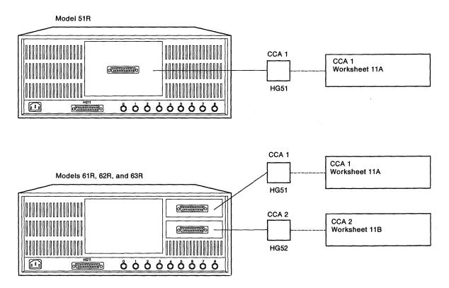
Note: You can install only one Concurrent Communication Adapter in Model 63R. It will be assigned hardware group number 51.
