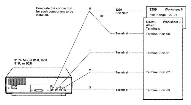
**Note:** If a 3299 Terminal Multiplexer is attached to connector 0, then no terminals can be directly attached to connector 1, 2, or 3.
