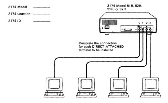
Note: If a 3299 is attached to connector 0, then no terminals can be directly attached to connectors 1 through 7.
