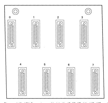
Figure 4-18. AEA Connectors on Models 1L, 1R, 2R, 3R, 11L, 11R, 12R, and 13R. For an illustration of the AEA connectors on other models, see Figure 3-6 on page 3-15.
