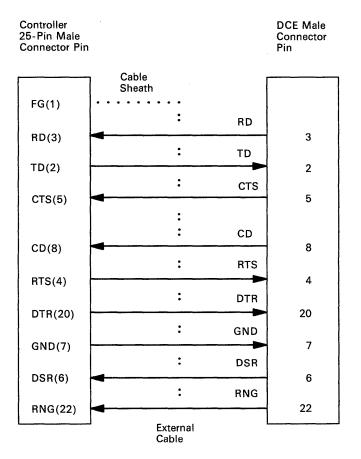
Figure 3-8. EIA 232D External Interface Cabling to a DCE
