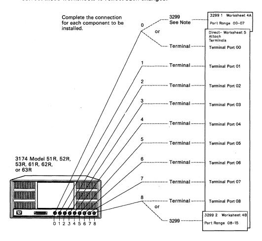
Note: If a 3299 Terminal Multiplexer is attached to connector 0, then no terminals can be directly attached to connectors 1 through 7.
