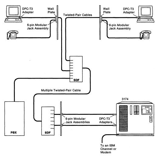
Figure 3-2. A 3270 Installation Using DPC-T3 Adapters and Twisted-Pair Cable
