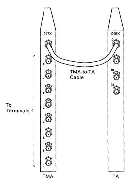
Figure 4-10. Cabling from Terminal Multiplexer Adapter to Terminal Adapter
