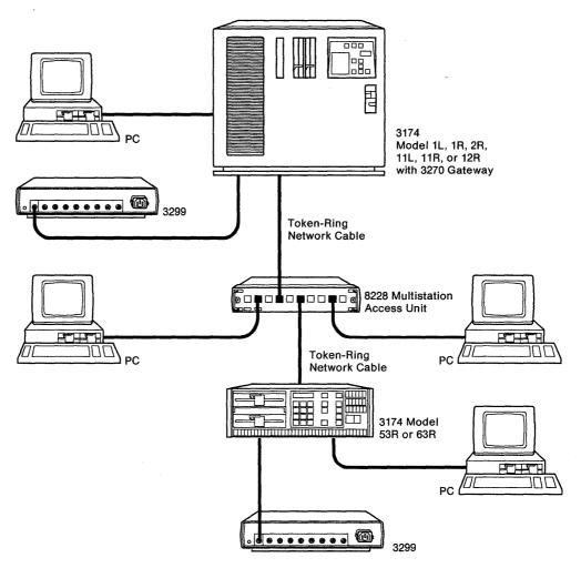
Figure 1-2. An Example of a 3174 Subsystem with a Token-Ring Network
