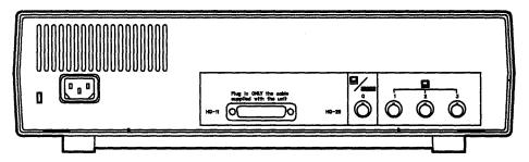
Figure 4-15. The Four Connectors on Models 81R, 82R, 91R, and 92R
