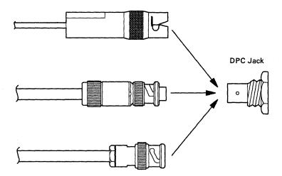
The BNC jack accepts only the BNC connector. Note that the BNC jack is shorter than the DPC jack.
