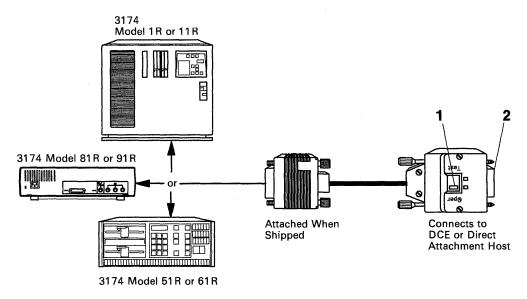
Figure 4-22. An EIA 232D Cable Connection
