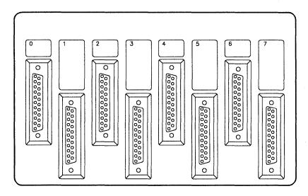
Figure 3-6. AEA Connectors for Models 51R, 52R, 61R, 62R, and 63R
