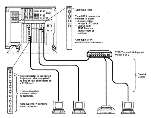
Figure 4-20. 3174 Terminal Cable Connections Using Coaxial Cable
