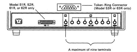
Figure 4-12. Models 51R, 52R, 53R, 61R, 62R, and 63R with Terminals Attached Directly to the Terminal Adapter
