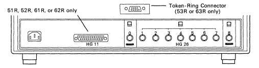
Figure 4-11. The Nine Connectors on Models 51R, 52R, 53R, 61R, 62R, and 63R
