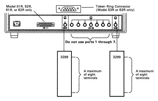
Figure 4-14. Models 51R, 52R, 53R, 61R, 62R, and 63R with Two 3299 Terminal Multiplexers
