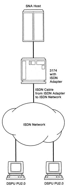
Figure 1-2. An Example of an ISDN Network
