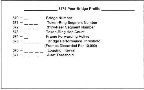
Figure 13-2. An Example of the 3174-Peer Bridge Profile Worksheet
