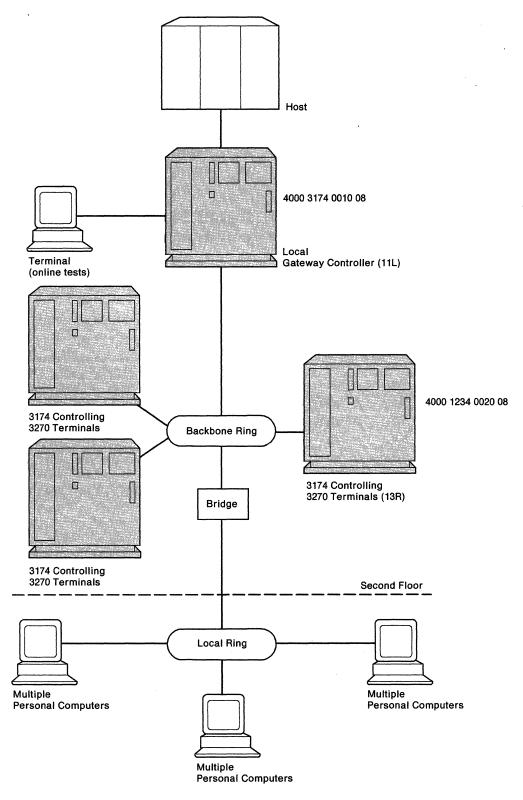
Figure C-1. Token-Ring Network - Local Gateway and Downstream 3174 13Rs
