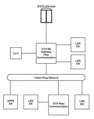
Figure 12-13. 3174 APPN NN/GW with Peer Communication including Bridge
