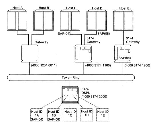
Figure E-5. Combination of Gateway Capabilities
