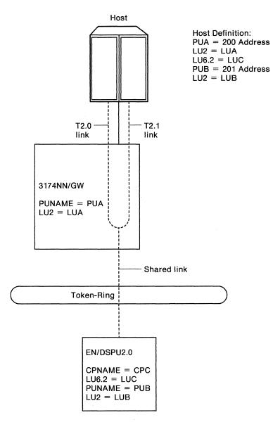
Figure 12-8. Network Node/Gateway Shared Link Support
