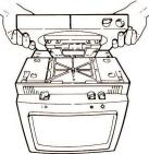
4. Holding the top edge of the front side of the video element, pull the logic element toward you until the stand snaps into place.
