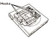
3. Insert the five hooks into the five slots of the video element.
