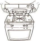
6. Holding the top edge of the front side of the video element, pull the logic element toward you until the stand snaps into place.
