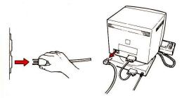
3. Unscrew and pull out **all cables** from the logic element.
