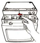
7. Remove the logic element with the stand from the video element.
