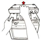
6. Push the latch to the left to unlock the stand from the video element.
