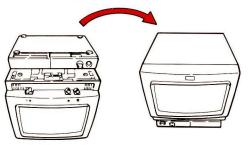
7. Insert **all cables**, except the power cord, into the video and logic elements and tighten the screws.
