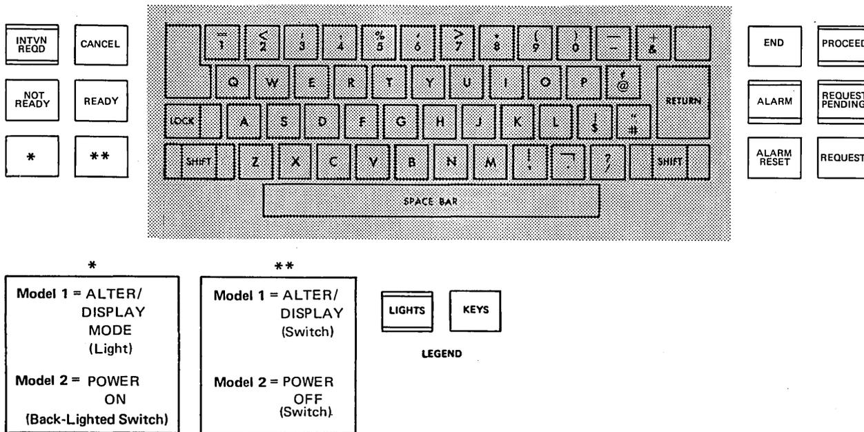
Figure 5. Operator's Control Keys and Indicator Lights
