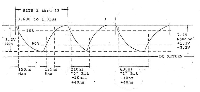
The following conditions for the coaxial cable must be observed:
