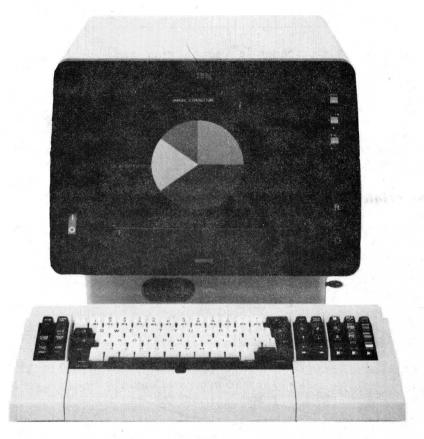
Figure 2-7. IBM 3279 Color Display Station
