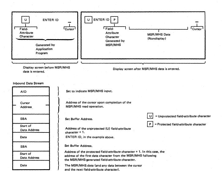
Figure 3-29. Operation of the Display with a Formatted Screen (MSR or MHS Using Numeric or Alphameric Character Set), Example 1
