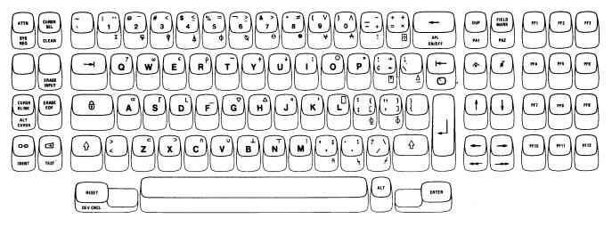
Figure E-8. 87-Key Typewriter/APL Keyboard
