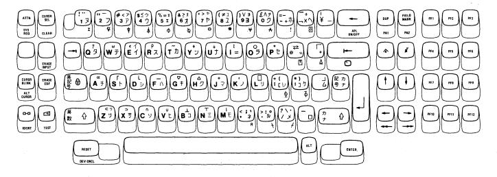
Figure E-9. 88-Key Katakana Typewriter/APL Keyboard
