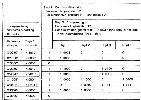
Figure K-3. Example of Compression Algorithm Using Comparison Rule 2
