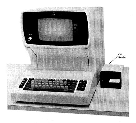
Figure 3-16. Operator Identification Card Reader (3275 and 3277 Attachment)
