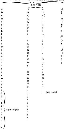
Note: The characters listed in the second and third columns constitute the character set for the (optional) 64-character EBCDIC print belt. The broken vertical bar  $(\frac{1}{1})$  is not on the 120-character TN print belt and cannot be entered from the text keyboard.
