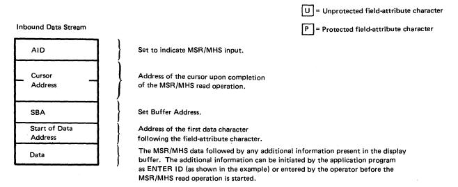
Note that with an unformatted screen the MSR/MHS data is the first data sent to the application program in the data stream.
