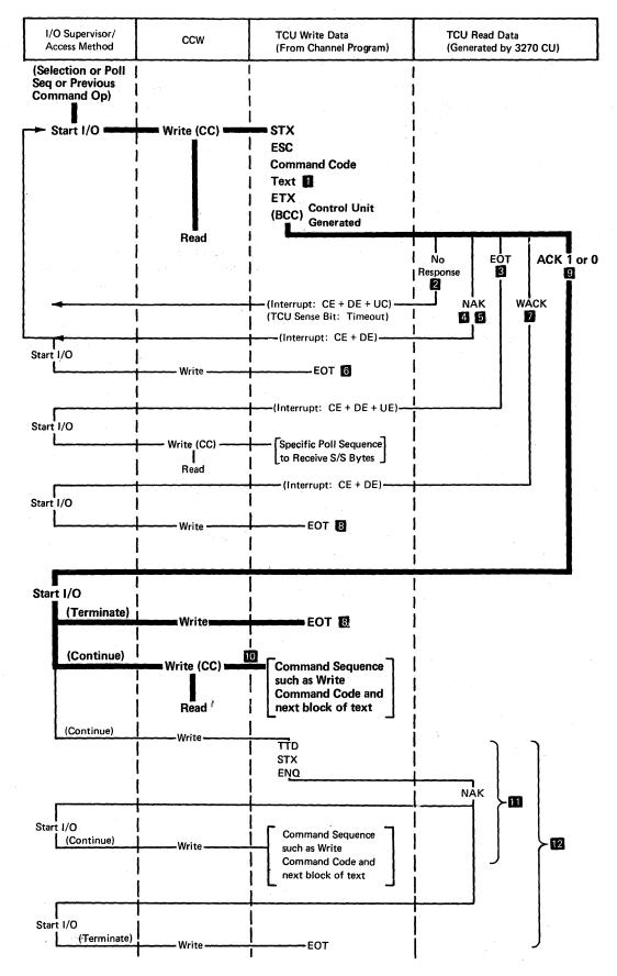
Figure 6-5 (Part 1 of 2). Write-Type and Control-Type Commands, Sequence/Response Diagram
