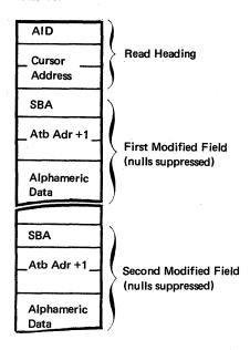
If a space or null selector-light-pen-attention AID is generated, at a 3275 or 3277 display, fields are not transferred to main storage during the read-modified operation. Instead, when a set MDT bit is found (indicating selector-light-pen and/or keyboard activity), only the Read Heading, the SBA order code, and the attribute address +1 are transferred.
