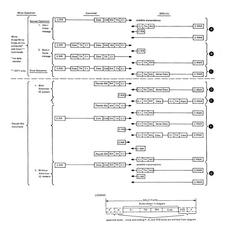
Figure 8-5 (Part 1 of 2). Write-Type Command Sequence/Response Diagram
