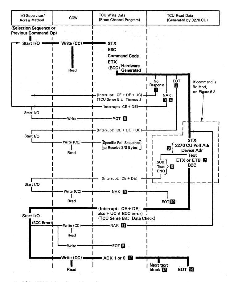
Figure 6-6 (Part 1 of 2). Read-Type Command, Sequence/Response Diagram
