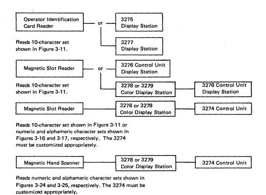
Figure 3-15. Attachment of Magnetic Reading Devices to 3270 System Units
