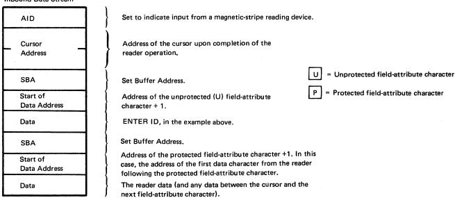
Figure 3-22. Operation of the Display with a Formatted Screen (OICR or MSR Using 10-Character Set), Example 1
