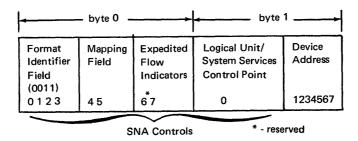
The SNA controls are employed by higher-level network management. A description of these controls, as implemented by the 3270 system, is provided in this section.
