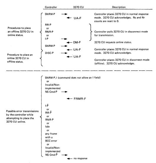
Note: Only SDLC by tes that are significant for the sequence being illustrated are shown in the diagram.
