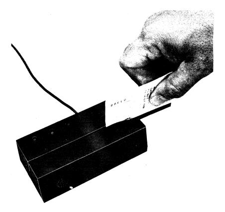
Figure 3-17. Magnetic Slot Reader (3276, 3278, and 3279 Attachments)
