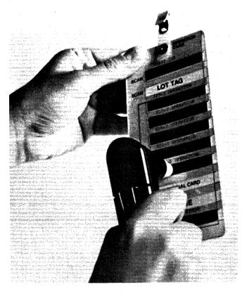
Figure 3-18. Magnetic Hand Scanner (3278 and 3279 Attachments)
