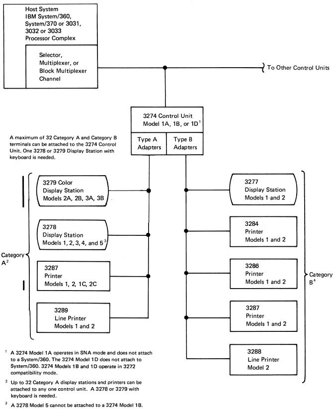
Figure 5-2. Locally Attached 3270 Display System Using a 3274 Control Unit Model 1A, 1B, or 1D
