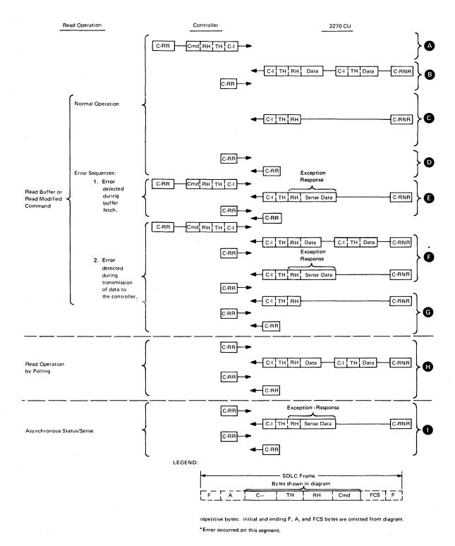
Figure 8-4 (Part 1 of 2). Read-Type Command Sequence/Response Diagram
