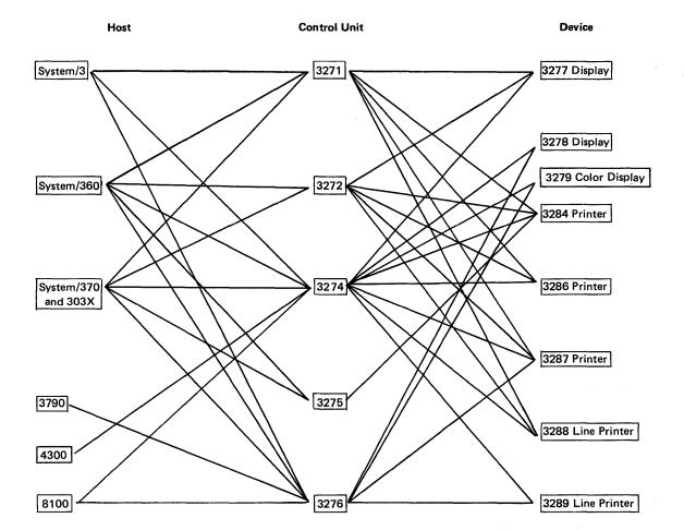
Figure 1-1. Host Control Unit and Device Combinations
