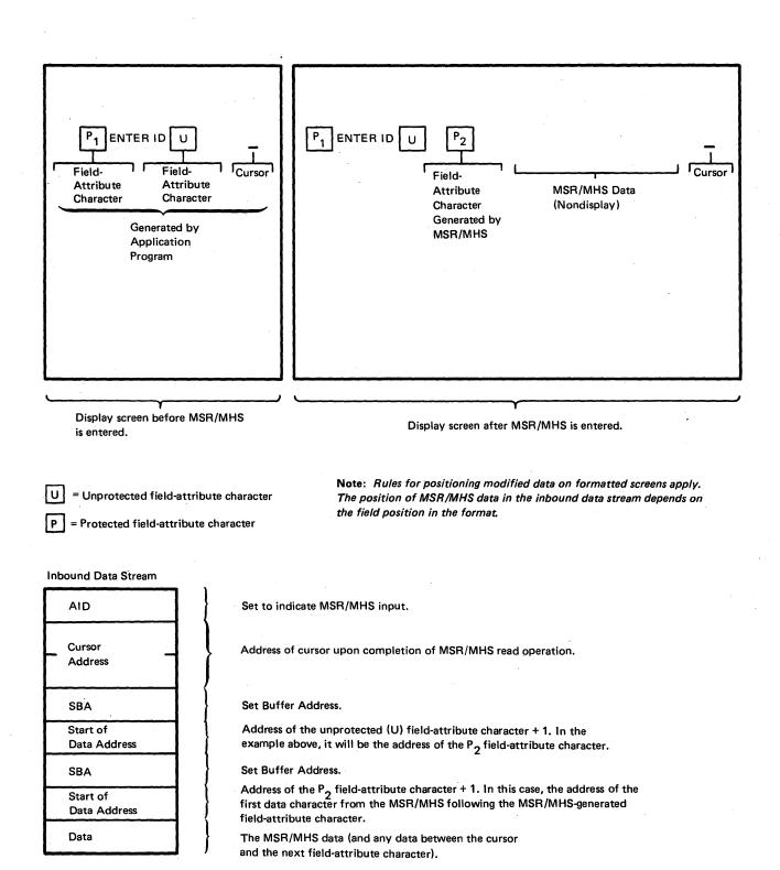
Figure 3-30. Operation of the Display with a Formatted Screen (MSR or MHS Using Numeric or Alphameric Character Set), Example 2
