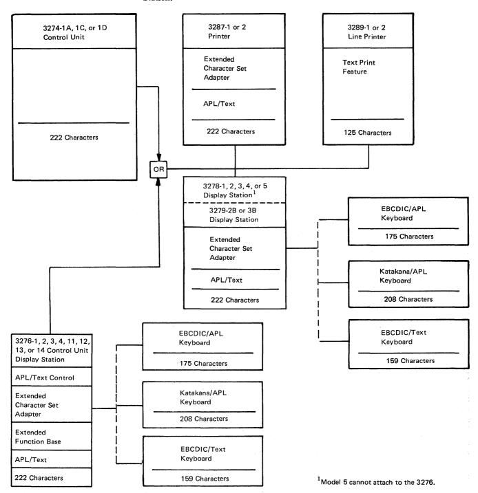
Figure E-1. Diagram of APL/Text Devices
