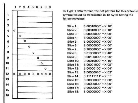
Figure K-1. Type 1 Data Format - An Example Dot Pattern Encoded
