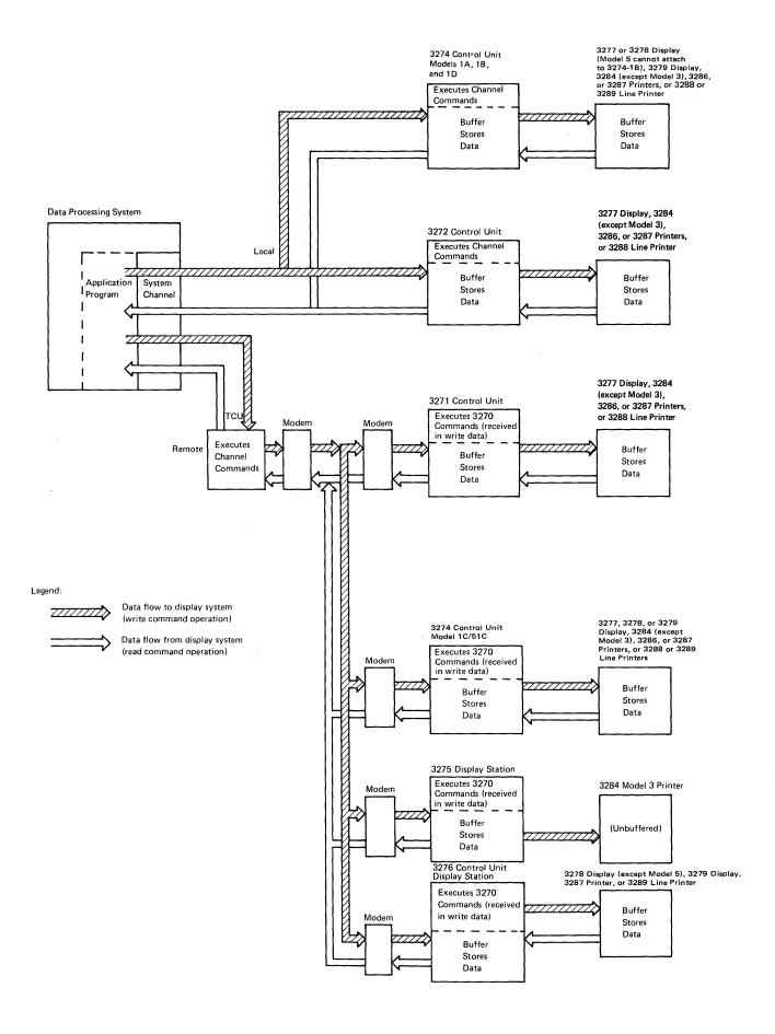
Figure 2-1. Data Flow between Data Processing System and 3270 Display System
