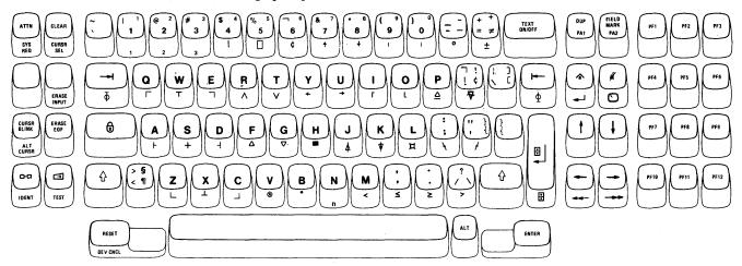
Figure E-10. 87-Key Typewriter/Text Keyboard
