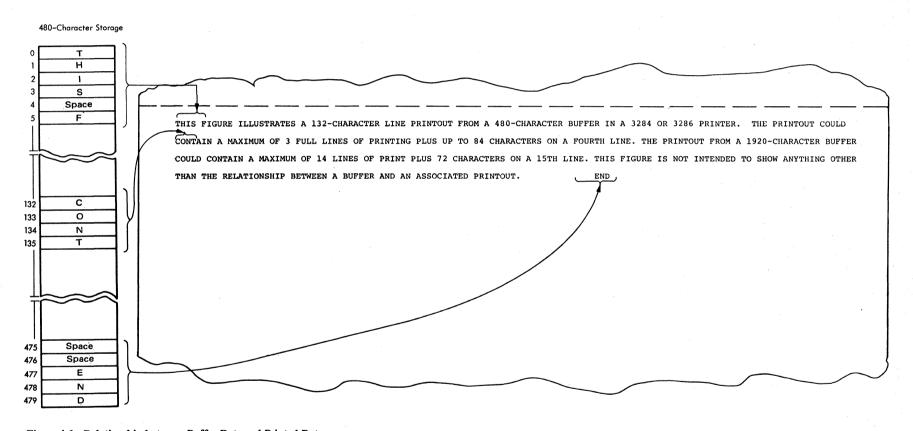
Figure 4-1. Relationship between Buffer Data and Printed Data
