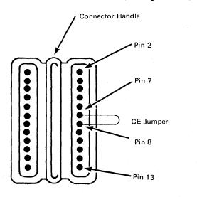
Figure 5-13. 3278 Top-Card Connector CE Jumper (Three Base Cards)
