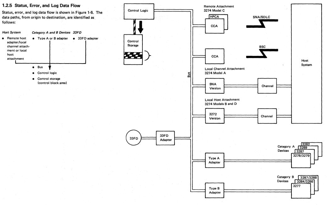
Figure 1-6. Status, Error, and Logic Data Flow
