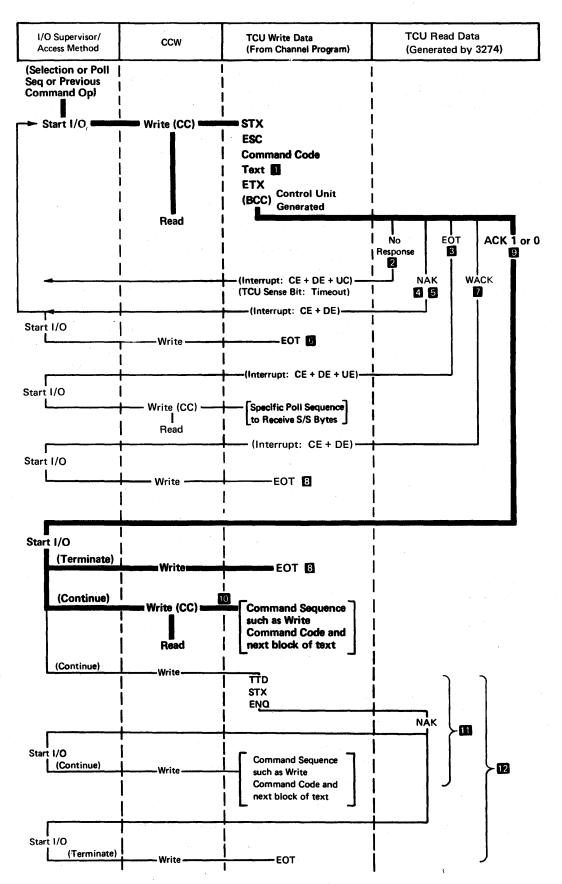
Figure 5-32. Write-Type and Control-Type Commands, Sequence/Response Diagram
