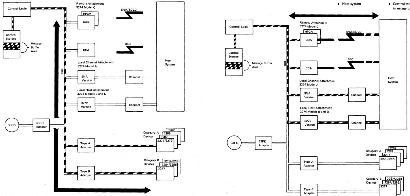
Figure 1-4. Message Data Flow between 3274 Control Unit and Devices
