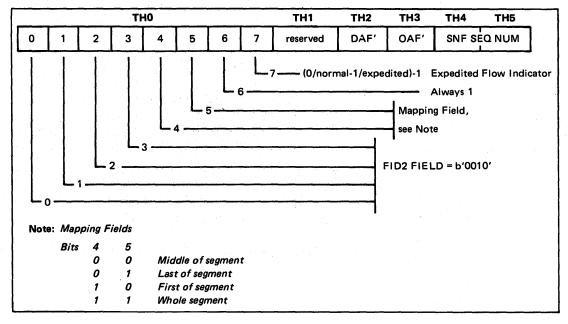
Figure 5-49. Transmission Header Format
