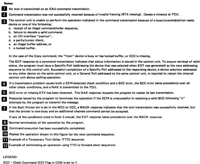
(Interrupt) = TCU-generated interruption (CE = Channel End, DE = Device End, UE = Unit Exception, UC = Unit Check).
