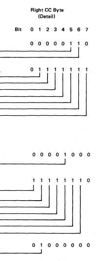
Figure 3-4 explains the sense-byte breakdown for CCA BSC. These conditions are logged only for nnn codes 311, 501, 530, 535, and 536, and the last error condition of that type.
