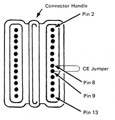
Figure 5-15. 3279 Top-Card Connector CE Jumper
