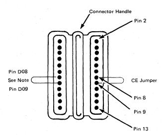
Figure 5-14. 3278 Top-Card Connector CE Jumper (Two Base Cards)
