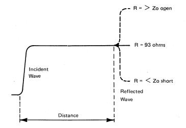
Figure 4-19. Incident and Reflected Waves
