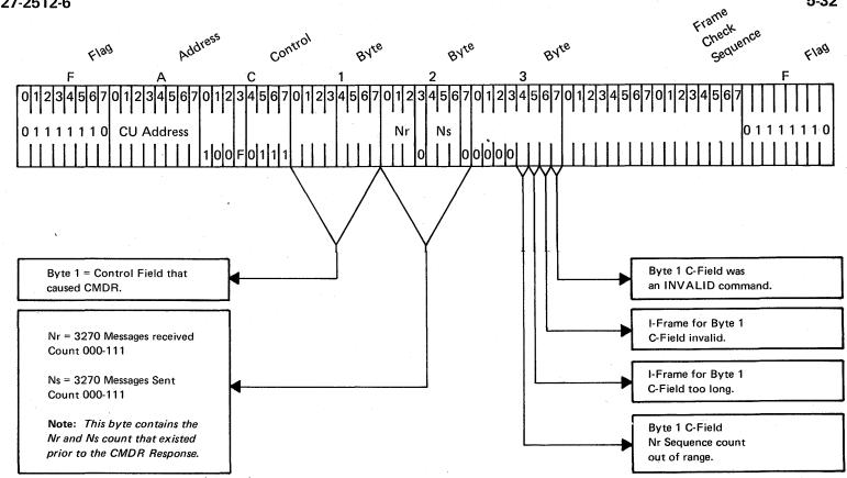
Figure 5-54. Command Reject (CMDR) Message Format
