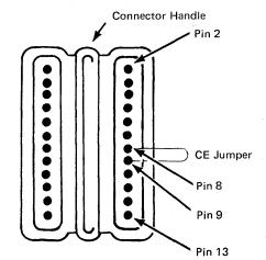
Figure 5-15. 3279 Top-Card Connector CE Jumper
