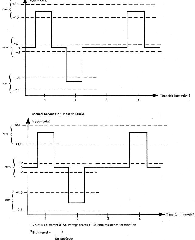
Figure 5-59. Digital Data Waveshapes
