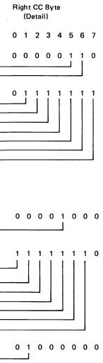
Figure 3-4 explains the sense-byte breakdown for CCA BSC. These conditions are logged only for nnn codes 311, 501, 530, 535, and 536, and the last error condition of that type.
