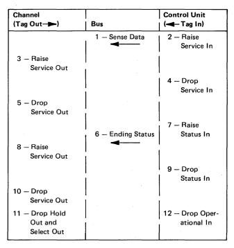
Figure 5-23. Sense—After Selection with Sense Command (Issued in Response to Unit Check Status)
