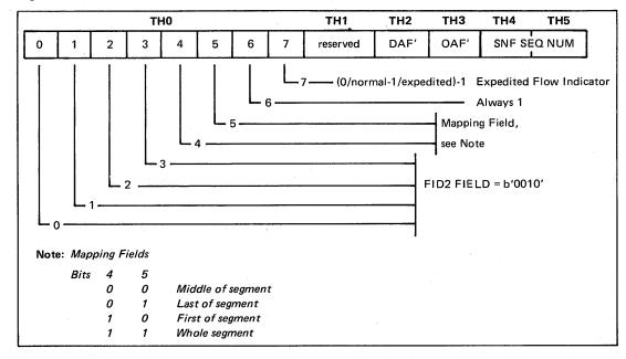
Figure 5-49. Transmission Header Format
