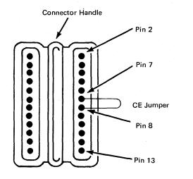
Figure 5-13. 3278 Top-Card Connector CE Jumper (Three Base Cards)
