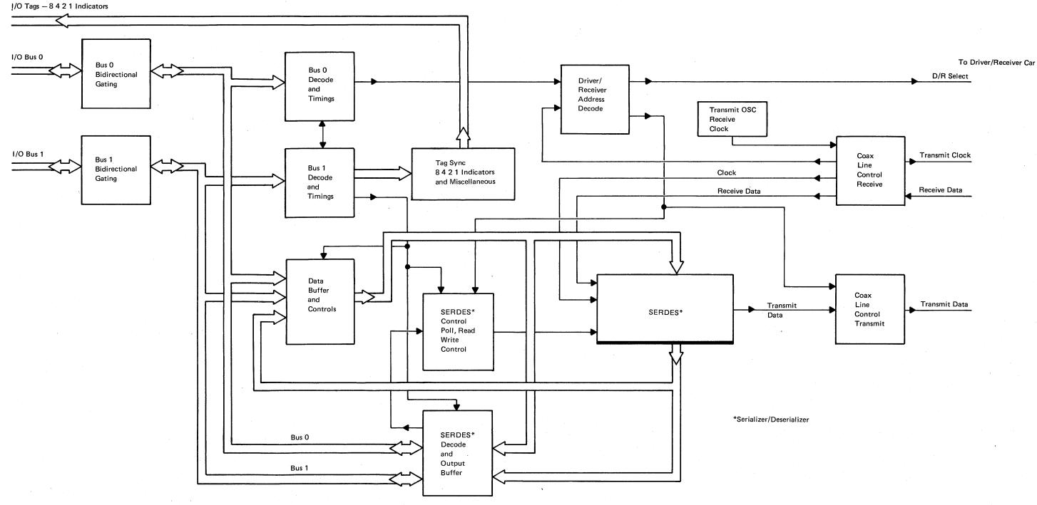
Figure 1-8. Keystroke Handling, Type A Adapter (without 3299)
