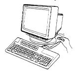
15. Remove the power cord from the display element.
