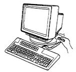
14. Remove the power cord from the display element.
