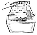
23. Remove the logic element from the display element.
