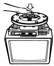
5 Make sure the stand is locked onto the display element by attempting to move the stand forward and backward.
