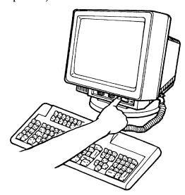
2 Insert the power cord into the display element as shown.
