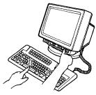
6. Hold the Space Bar down and wait approximately ten seconds. The "Offline Setup" panel appears on the screen.
