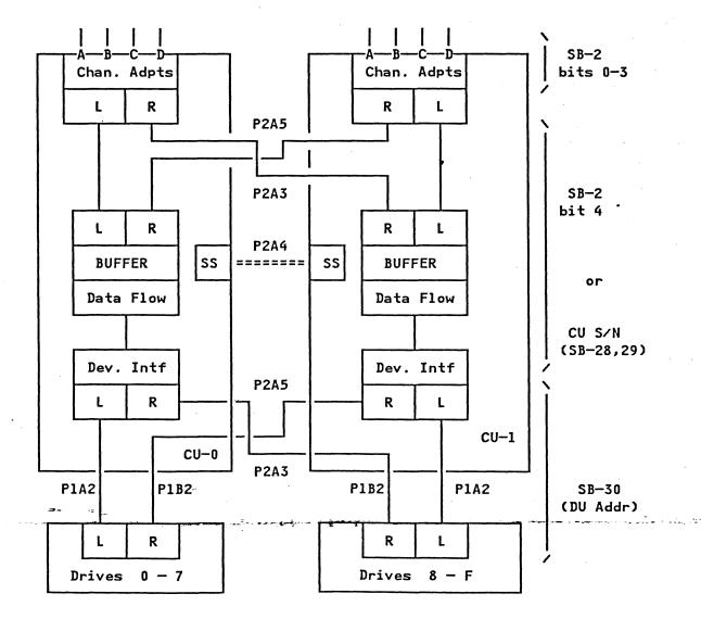
As showed above, SB2 bits 0-3 identify the CA and the CU having it, over which the sense data was sent to the host, I mean, through which, the error was reported.
